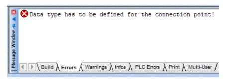
To correct this issue, double click the line in the network which is connected between two functions to bring up the flag type or right click the line. Choose 'Object Properties' and select the appropriate flag type. For example, select BOOL for flag type in case the line in the network is connected to EN/ENO which requires Boolean input.
