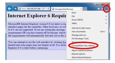
3. In the Compatibility View Setting dialog, the controller's IP address will automatically populate the "Add this website:" entry field. Click the Add button to add it to the compatibility list. You must do this for every controller you wish to connect to.
