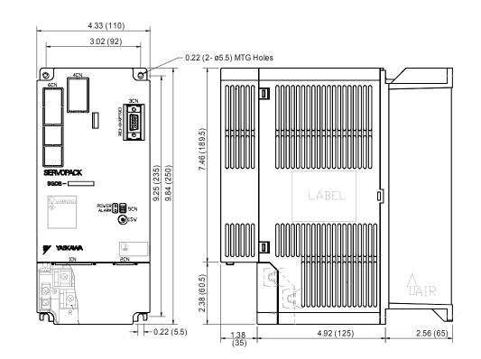
Sigma I ServoAmplifier SGDB-05AD SGDB-10AD
