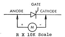
R greater than 20K ...... thyristor O.K. R greater than 2K, less than 20K ..... questionable thyristor R less than 2K ..... faulty thyristor
