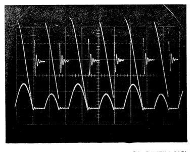
F. UNBALANCED OUTPUT (WITH LOAD)
