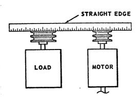
Figure 3.2 Sheave Alignment
