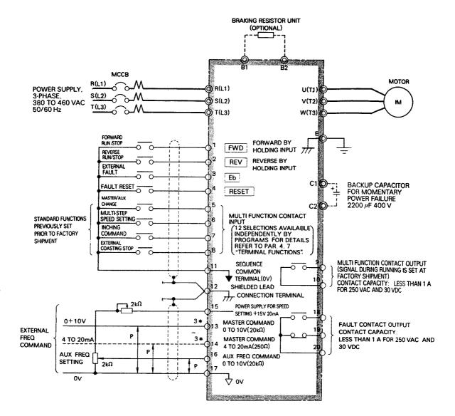
Fig. 5 Example of Interconections for Operation by External Signals
