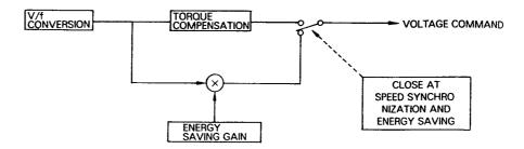
Fig. 20 Output Voltage During Energy-Saving Run
