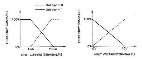
Fig. 10 Input method of Master Frequency Command
