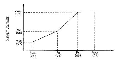
Fig. 16 V/f Characteristics by Control Constants 1 to 7
