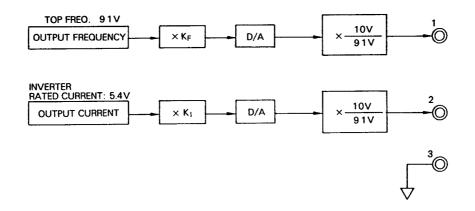
Fig. 19 Block Diagram of F-I Monitor
