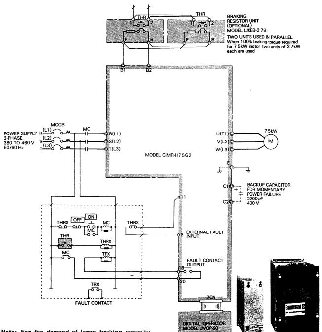
Note: For the demand of large braking capacity, refer to the right table and connect braking resistor units in parallel.
