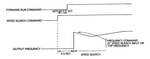
Fig. 13 Time chart at Speed search command Input
