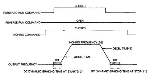
Fig. 12 Time chart at Forward and Inching Operations
