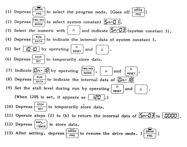
To remove the function to prevent stall prevention during operation To remove the function to prevent stall during operation, set the stall prevention during operation level to 200%.
