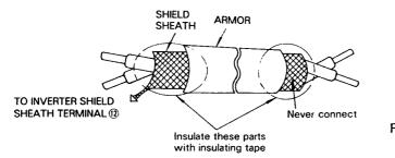
Fig. 6 Shielded Lead Termination
