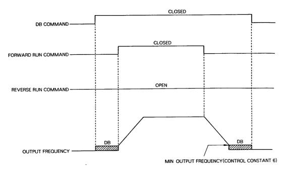
Fig. 15 Time Chart of DC Dynamic Braking
