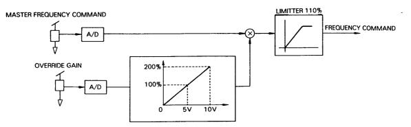
Fig. 11 Block Diagram of Override
