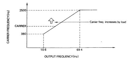
Fig. 18 Carrier Frequency and Output Frequency
