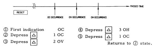
(2) To indicate the sequence of failure items that occurred before the power was turned off
