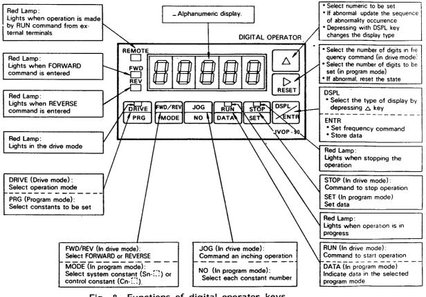
Fig. 8 Functions of digital operator keys
