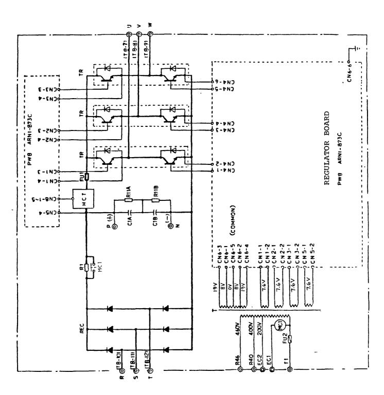
FIGURE 27 WIRING DIAGRAM-MAIN CIRCUIT
