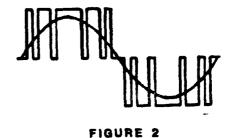
Pulse width is decreased for lower RMS voltage and increased for higher voltage. Lower frequencies have a greater number of pulses in one cycle. As the frequency increases, the microprocessor selects the optimum number of pulses per waveform.
