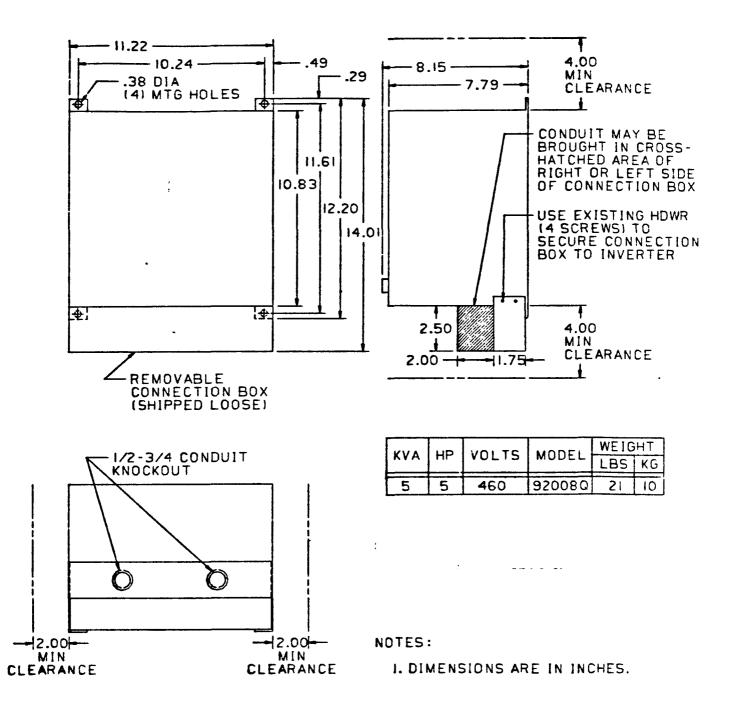
FIGURE 14 EXTERNAL VIEW AND DIMENSIONS
