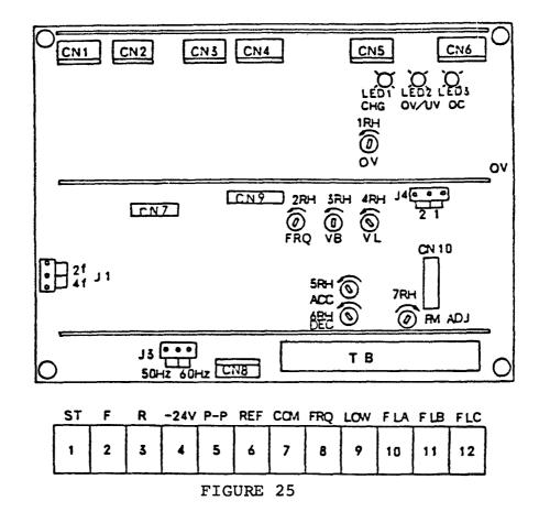
Printed Circuit Board Parts Arrangement Diagram with Enlarged View of Terminal Board
