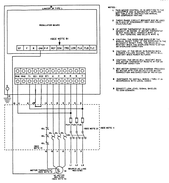
FIGURE 188 INTERCONNECTION DIAGRAM
