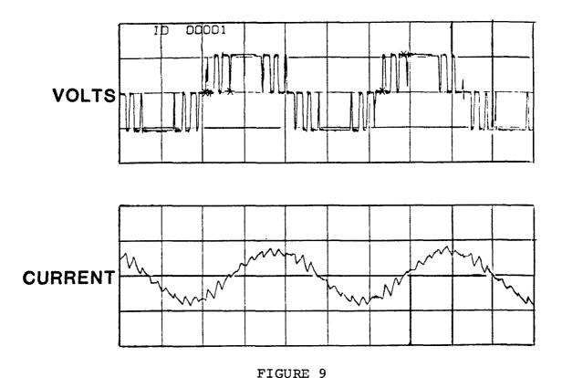
Proper 120° phase shift between output leads stays constant over the entire frequency range. Typical motor voltage and current at 60 hertz (full load) is shown in Figure 9. Note that although the voltage is pulses, the current waveform is near sinusoidal. Voltage is leading current, typical in induction motors.
