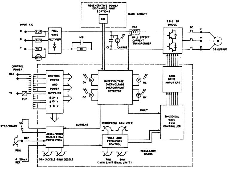
Figure 3 shows a block diagram of the 460V unit.
