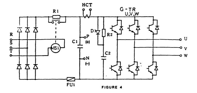
Incoming 3 phase A.C. line voltage is rectified to a 650V D.C. bus by the diodes in the full wave rectifier.
