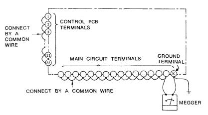
Figure 10. Connections for Megger Testing
