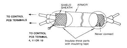
Figure 8. Shielded Lead Termination
