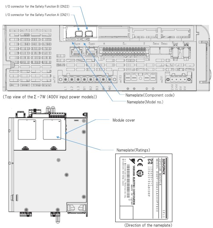
(Side view of the  $\Sigma$  -7W (400V input power models))
