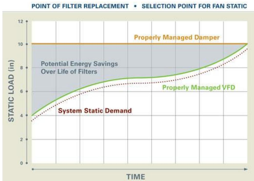
Figure 1 Design System Static <sup>2</sup>
