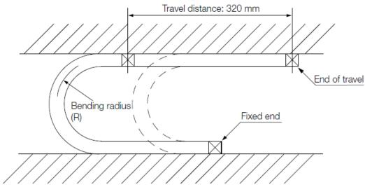
Note: The service life of a Flexible Cable indicates the number of bends while the lead wires are electrically charged for which no cracks or damage that affects the performance of the cable sheathing occurs. Breaking of the shield wire is not considered.
