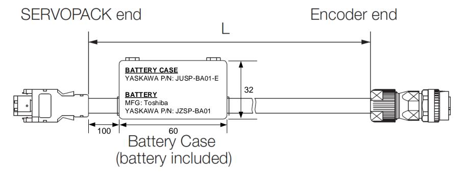
The recommended bend radius is **46mm** or larger for **moving** parts of machines, such as robots. See <u>Page 2</u> for Precautions for Flexible Cables.
