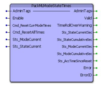
The PackMLModeStateTimes function block keeps track of the times spent in each mode and state of operation for the machine. Whenever the cpu is running, time is added to the current state of the current mode every second.
