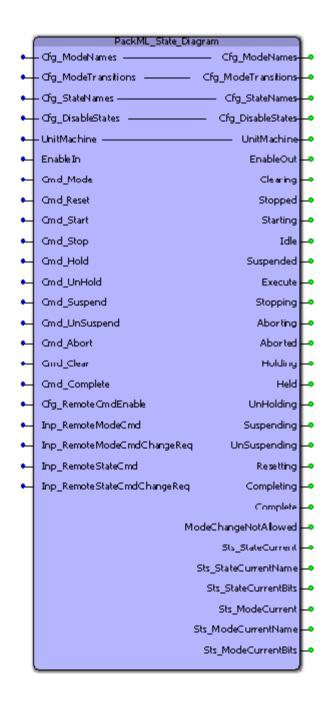
The PackML\_State\_Diagram function block handles the operation of the state machine, including mode and state transitions, as defined in the OMAC PackML specification. This function block, when first enabled, initializes the machine to be in mode 3 (Manual Mode) and in the Stopped state.
