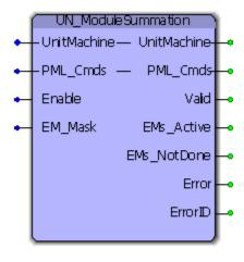
The UN\_ModuleSummation function block rolls up the Equipment Module (EM) State Complete bits for all active and enabled EMs. The result is an overall PMLs State Complete bit that is transferred to the PackML\_StateControl function.
