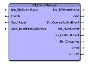
The EM\_EventManager function block collects all the events that occurred in the enabled and active Control Modules within a particular Equipment Module. Active categories are OR'd together and outputs are provided for the number of active events and which event was the first to occur. Activating Cmd\_Reset will clear all the stored events for the module.
