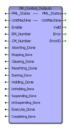
The CM\_Control\_Outputs function block sets the State Complete bits for the control module to be passed up and assembled into the Equipment Module status in the EM00\_ModuleControl worksheet.
