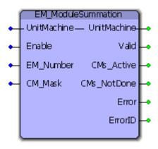
The EM\_Module\_Summation function block rolls up the Control Module State Complete bits for all active and enabled CMs. The result is an overall Equipment Module State Complete bit that is transferred to the UN\_ModuleControl Worksheet.
