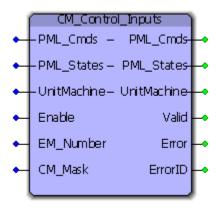
The CM\_Control\_Inputs function block passes the high level commands from the PackML\_StateControl into each of the enabled and active Control Modules.
