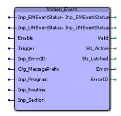
The Motion\_Event function block is designed specifically for capturing Yaskawa Motion Function Block alarms. It features an internal lookup that provides alarm information based on the error code. Typically, a function block from the Yaskawa firmware library triggers the Motion\_Event block.
