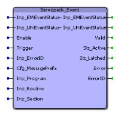
The Servopack\_Event function block is designed specifically for capturing Yaskawa SERVOPACK alarms. It features an internal lookup that provides alarm information based on the error code. Typically, an Axis\_Control function block from the Yaskawa PLCopen Toolbox triggers the Servopack\_Event block.
