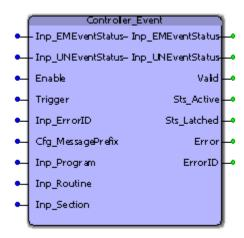
The Controller\_Event function block is designed specifically for capturing Yaskawa MPiec Controller alarms. It features an internal lookup that provides alarm information based on the error code. Typically, an Axis\_Control function block from the Yaskawa PLCopen Toolbox triggers the Controller\_Event block.
