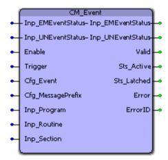
The CM\_Event function block captures User-Defined Events that occur in a Control Module to be fed up to the EM\_EventSummation block. Custom User Events are configured in the PackMLEvents\_Init function block. Additional inputs are provided for the user to attach descriptive strings that can further identify where the event originated. As events are triggered, the time of the event is time stamped. When the event is cleared, another timestamp records the acknowledged time.
