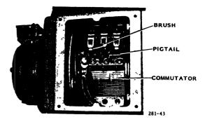
Fig. 5 Inspection Window of DC Motor
