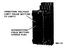
Fig. 10 Field Adjuster Type JCSM-51-17
