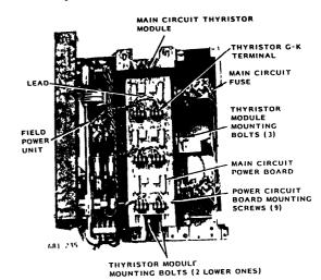
Fig. 15 Main Circuit Thyristor Assembly (230V, 260A System)
