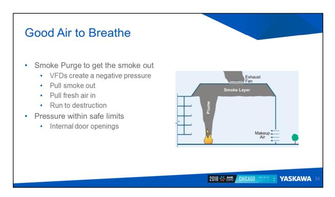
Different from exit path pressurization, smoke removal means using VFDs and fans to exhaust the smoke and harmful gases.
