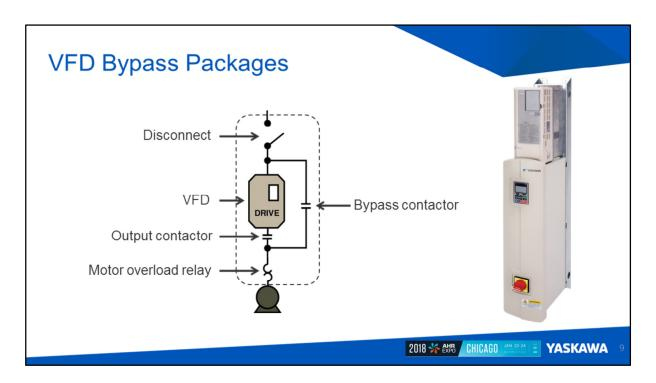
As we've discussed, to run a fan at variable speed, you can use a VFD to vary the speed of the motor.
