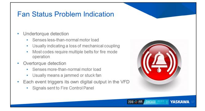
In addition to fan speed control, firefighters require positive status of fan operation at the Fire Fighters' Smoke Control System (FSCS) Panel. They want to know, at the panel, whether the fan is running properly, and if not, the nature of the problem. The VFD can monitor motor current draw to detect a wide variety of problems that would cause the fans to not move air as needed. Here, Undertorque Detection senses too little current draw and Overtorque Detection senses too much.
