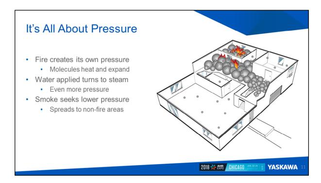
In the process of fire, fuel is combined with oxygen to produce light, heat and smoke. In a building fire, this usually mean solid objects are being converted to gas, so what was a relatively small volume is now many, many times its original size as molecules heat and expand. So in that process, fire creates its own pressure within a structure. Added to that, is the pressure from the steam that results from the water that responders apply to suppress the fire.
