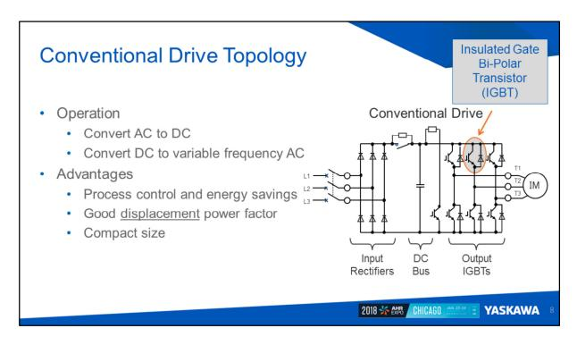
Now a quick review on how VFDs work. Conventional VFDs – and I use the term "conventional" here to distinguish them from a newer and different design – are all of the same basic structure.
