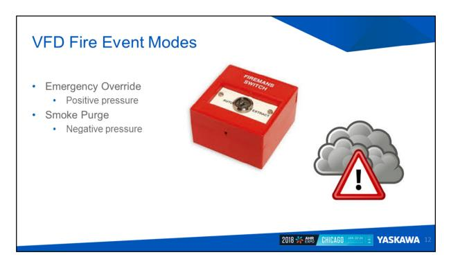
Different brands of VFDs have different modes for dealing with pressure during fire events. The names given for these modes include Emergency Override, Firemen's Override, Smoke Purge, and others, which differ in their capabilities for controlling speed and reacting to faults. However, what they have in common is the ability drive fans to raise or lower pressure to help insure occupant safety.
