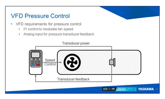
Using a variable frequency drive to control the stairwell pressurization fan can assure the proper safe pressure level, provided it meets two critical functionality requirements.
