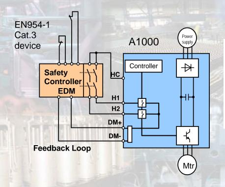
To use the Safe Disable input function, remove the short between H1/H2 and HC (a temporary jumper is placed between these terminals for shipping).
