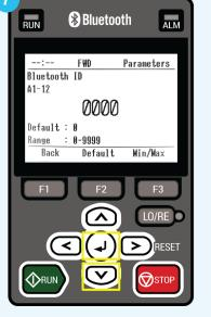
Push the arrow keys to set the Bluetooth ID, then push Enter when done. Set a non-zero value to enable Bluetooth.
