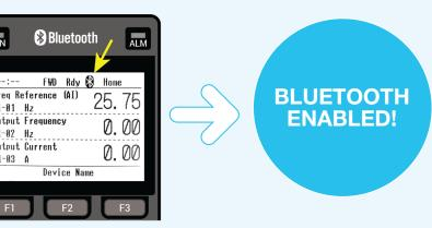
WAIT 60 seconds or unplug and reconnect the keypad to immediately broadcast Bluetooth. The Bluetooth icon indicates Bluetooth is ON.
