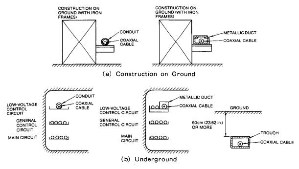
Fig. 2.9 Laying Coaxial Cables between Buildings
