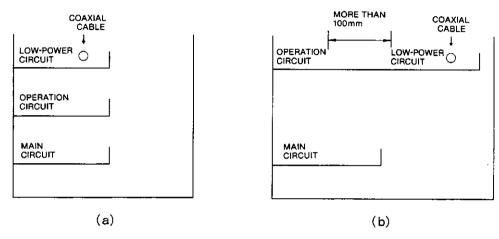
Fig. 2.5 Wiring Duct Separation
