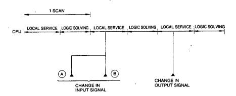
Fig. 4.3 I/O Timing of Local I/O Channel
