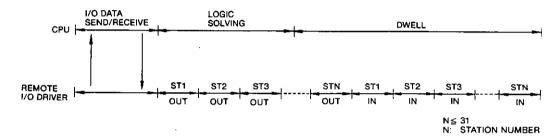
Fig. 4.1 Logic Solving and I/O Processing
