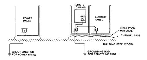
Fig. 2.14 Remote I/O Panel Insulation
