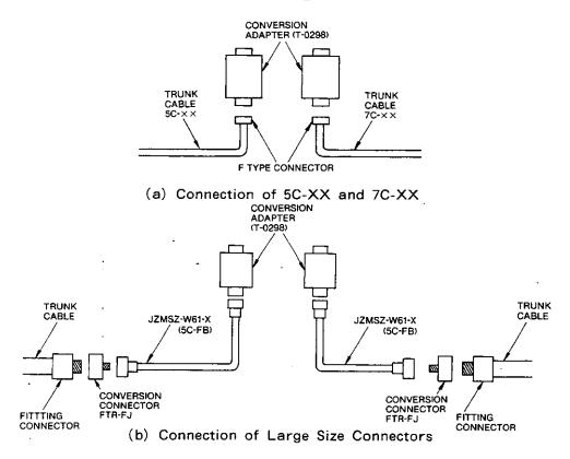
Fig. 2.3 Connection using F Type Connector
