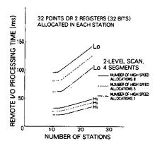
Number of I/O Allocations: 1024 bits constant Transmission Speed: 4 Mbps Number of Segments: 4
