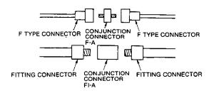
Fig. 2.4 Connection between Coaxial Cables
