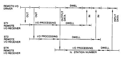
Fig. 4.6 I/O Timing of Remote I/O Station
