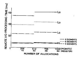
Number of Stations: 1Transmission Speed: 2 MbpsOutput Processing
