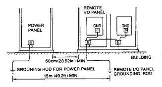
Fig. 2.12 Separation from Power Panel
