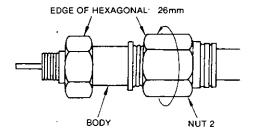
Note: Fully insert the body and tighten nut 2.
