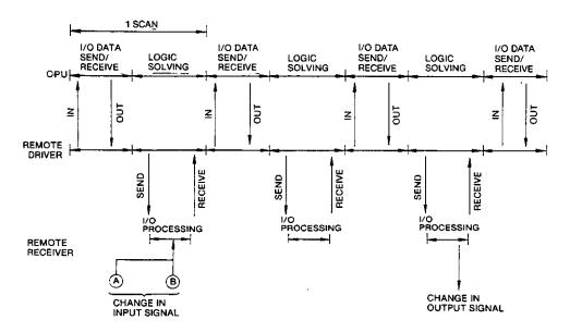
Fig. 4.4 1/O Timing of Remote I/O Channel
