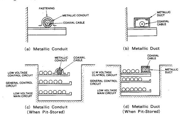
Fig. 2.6 Coaxial Cable Installment
