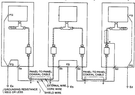
Fig. 2.11 Example of Coaxial Cable Grounding
