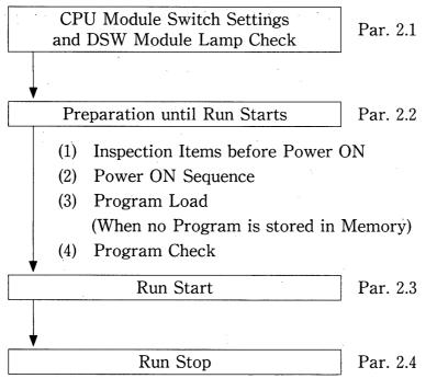
Fig. 2.1 Run Operation Procedure of CP-3300
