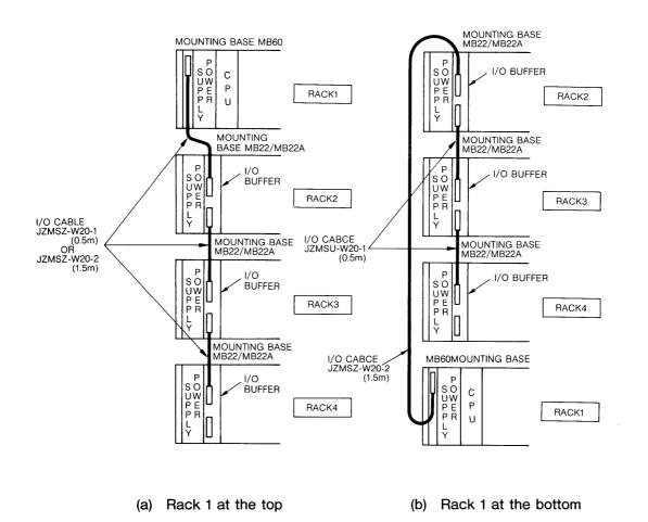
Connect the I/O cable so that the signal flow will be from OUT to IN. (See Fig. 1.9.)
