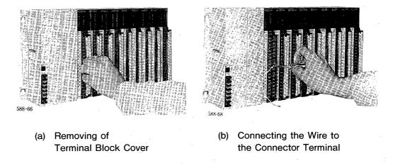
Fig. 1.10 Connecting the Wire to the Connector Terminal
