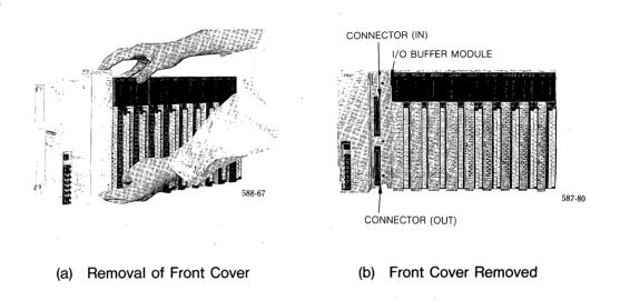
Fig. 1.8 Connector for I/O Cable Connection of I/O Buffer Module
