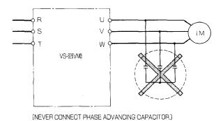
Fig. 4.16 Removal of Phase Advancing Capacitor
