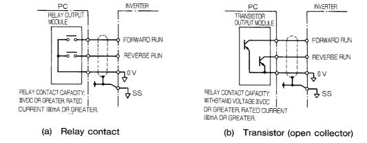
Fig. 7.14 Example of Connection of Operation Signals
