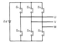
Fig. 6.1 Operating Principle of an Inverter
