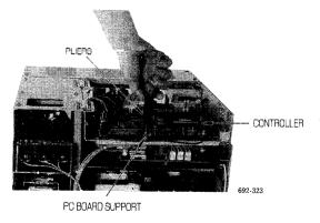
Fig. 15.5 Holding the PC Board Support with Pliers
