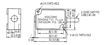
Fig. 5.4 Dimensions of Magnetic Sensor in mm (inches)
