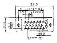
Fig. 5.22 Dimensions of I/O Signal Connector
