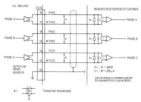
Fig. 4.25 Output Circuit and Receiver circuit
