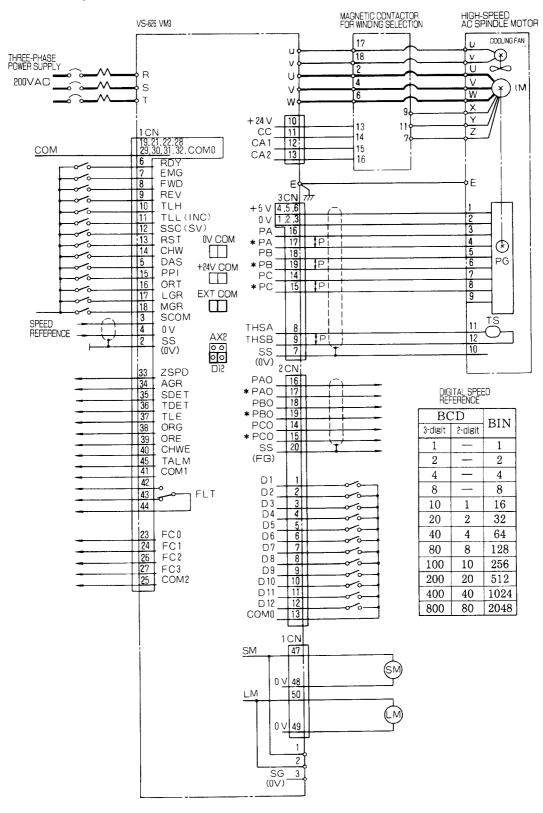
Fig. 4.11 Standard Wiring Diagram (Winding Selection Type)
