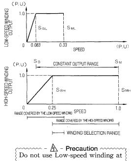
Do not use Low-speed winding at speeds over  $S_{ML}$ , which are not covered.
