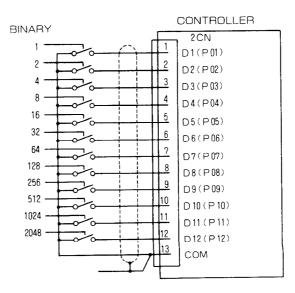
Fig. 5.6 Interconnection Diagram
