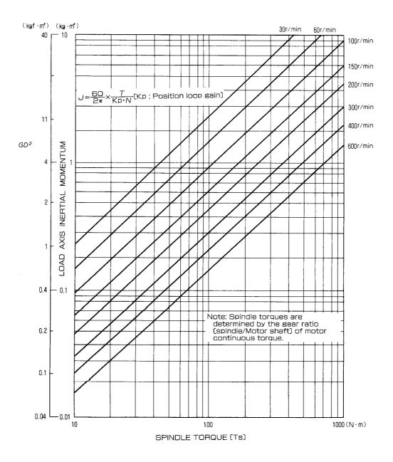
Fig. 14.9 Orientation Speed Setting
