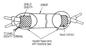
Fig. 11.5 Shielded Lead Termination
