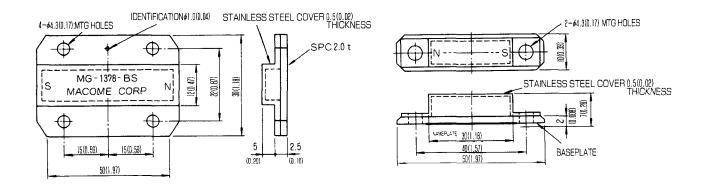
Fig. 5.3 Dimensions of Magneto in mm (inches)
