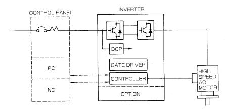
Fig. 4.2 System Configuration
