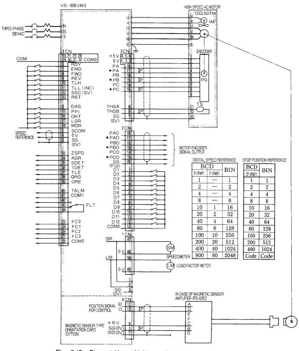
Fig. 8.18 Stop at Home/Arbitrary Position by Magnetic Sensor
