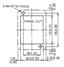
Fig. 5.19 Panel Cutting for Mounting the Digital Operator
