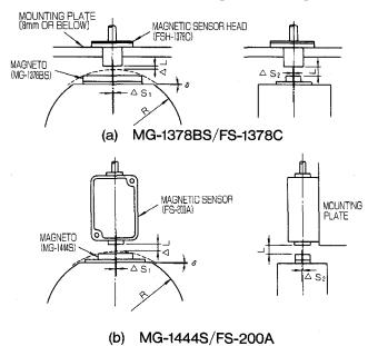
Fig. 5.8 Installing Magneto and Magnetic Sensor (1)
