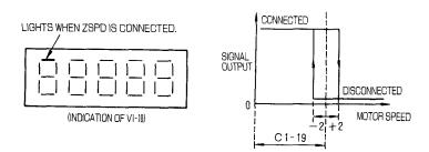
Fig. 14.3 Zero-speed Signal Detection Level and Operation Indication
