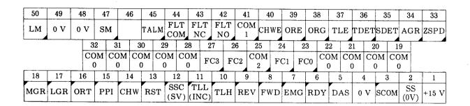
PCB Side Connector; MR-50RMAG Cable Side Connector; MR-50LF (G)
