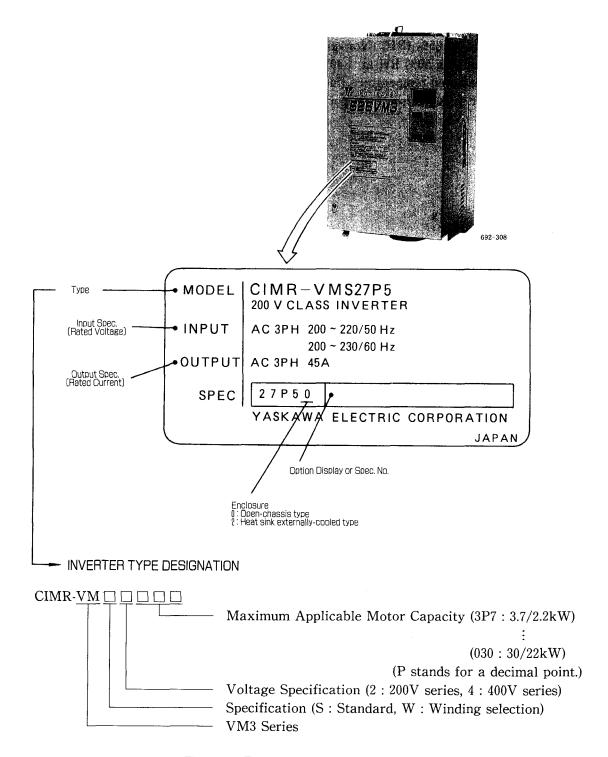
Fig. 9.2 Example of Inverter Nameplate
