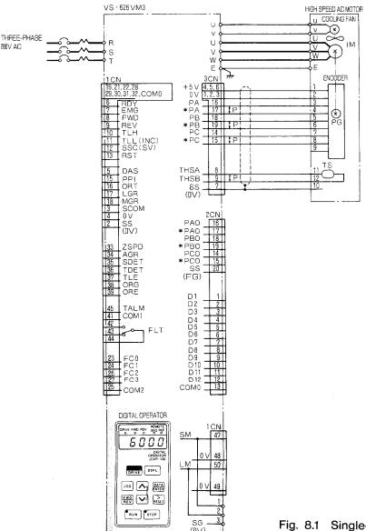
Fig. 8.1 Single-Motor Operation with Digital Operater
