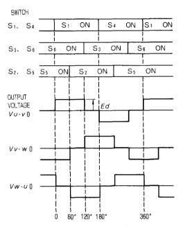
Fig. 6.2 Switching Operation and Output Voltage
