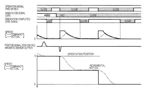
Note: When incremental positioning is performed, a position shift must not be generated while the orientation signal is turned off.
