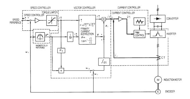
Fig. 6.6 Control Block Diagram of VS-626VM3
