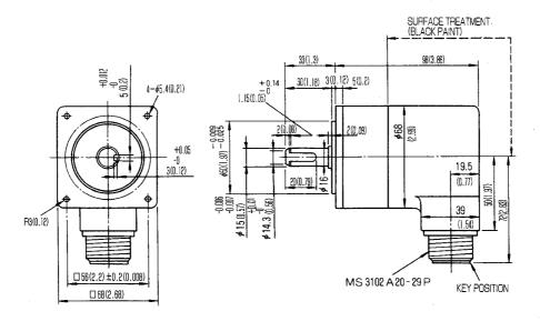
Note: 1. Install the encoder with the greatest possible care, so as not to generate backlash, because it will lead to a positional deviation.
