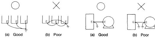
Fig. 4.14 Grounding of Three VS-626VM3 Units
