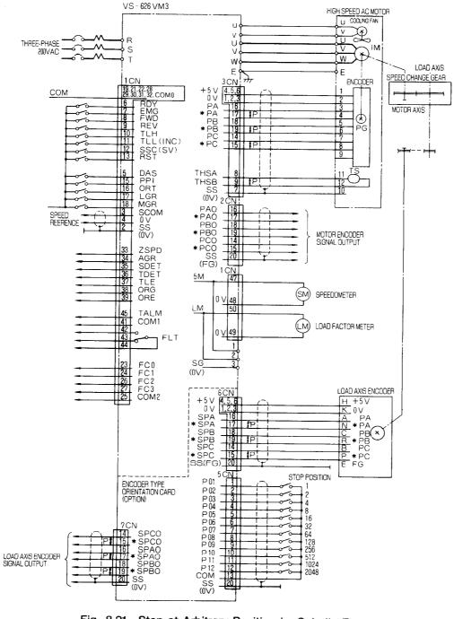
Fig. 8.21 Stop at Arbitrary Position by Spindle Encoder
