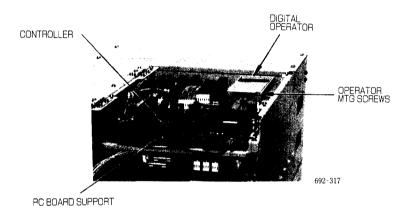
Fig. 15.6 Installing Controller
