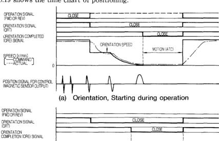
Fig. 8.19 shows the time chart of positioning.
