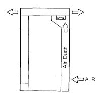
Fig. 7.19 Structure of control panel with air duct
