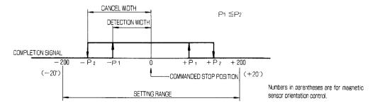
Fig. 14.8 Completion Signal Detection Position
