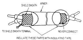
Fig. 4.13 Shielded Lead Termination
