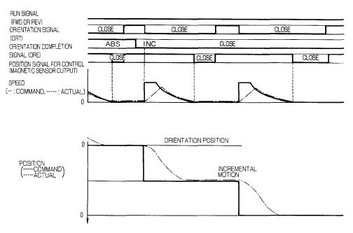
Note: When incremental positioning is performed, a position shift must not be generated while the orientation signal is turned off.
