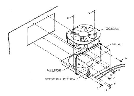
Fig. 15.7 Replacing the Inverter Cooling Fan
