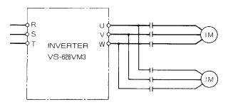
Fig. 4.18 Connection for Switching Motors
