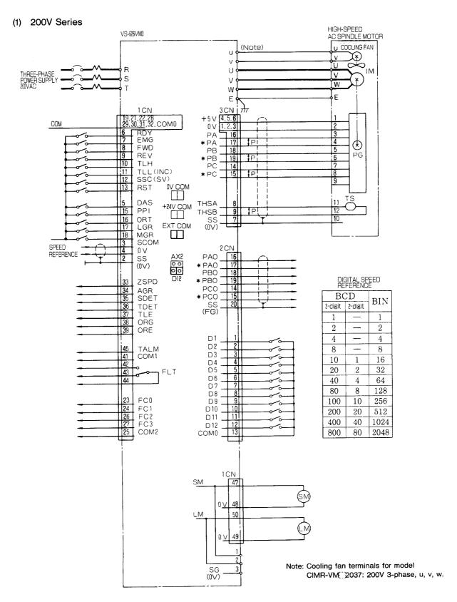
Fig. 4.9 Standard Wiring Diagram (200V Series)
