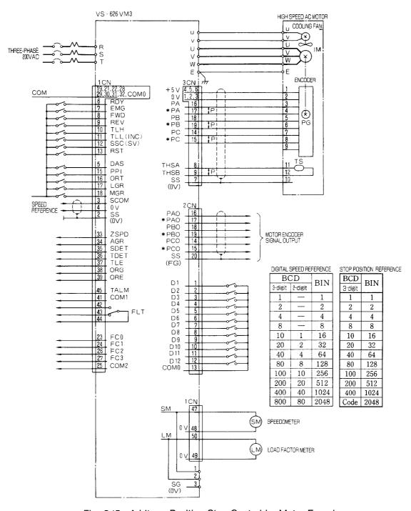
Fig. 8.15 Arbitrary Position Stop Control by Motor Encoder
