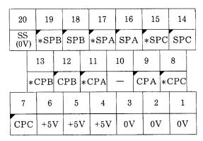
PC Board Connector: MR-20RMAG Cable Side Connector: MR-20LF (G)
