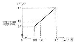
C1-17 = (120% of 30-minute rating) / indication on the load factor meter
