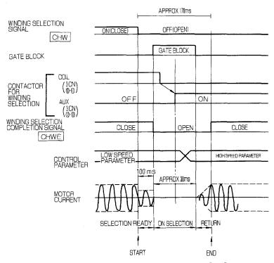
Note: Auxiliary contacts of magnetic contactor for winding selection type (3CN®-®) can be checked by control signal V1-09. CHWA LED of V1-09 goes ON when the auxiliary contacts are closed.
