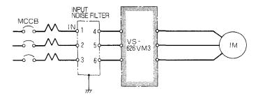
Fig. 4.19 Example of Connecting a Input Noise Filter
