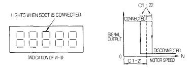
Fig. 14.5 Speed Detection Level and Operation Indication
