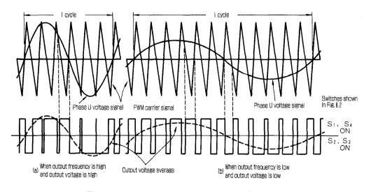
Fig. 6.3 Sine Wave PWM Control System
