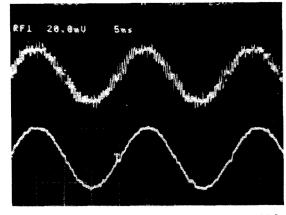
PWM FREQUENCY (Upper: 3.8kHz; Lower: 10kHz)
