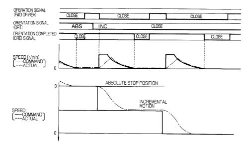
Note: To use incremental positioning, be careful not to move the spindle while the orientation signal is OFF. Otherwise, stop position precision is reduced.
