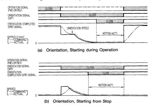
Fig. 8.22 Absolute Positioning Operation
