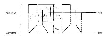
Fig. 7.13 Time Chart of Motor Torque and Speed
