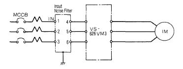
Fig. 5.20 Example of Connecting Input Noise Filter
