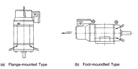
Fig. 14.1 Motor Cooling Air Passage
