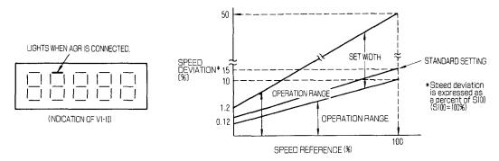
Fig. 14.4 Speed Agree Width Setting and Operation Indication
