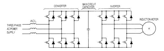
Fig. 6.4 Configuration of Inverter
