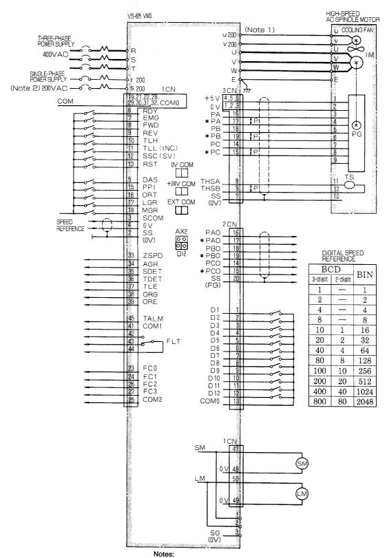
1. Cooling fan terminals for model CIMR-VM[]4037 : 200V 3-phase, u200, v200, w200. 2. Control power supply for model CIMR-VM[]4037 : 200V 3-phase, r200, s200, t200.
