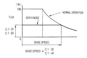
Fig. 14.7 Flux Level in Servo Mode
