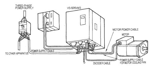
Fig. 11.4 Configuration for Single-Motor Drive System
