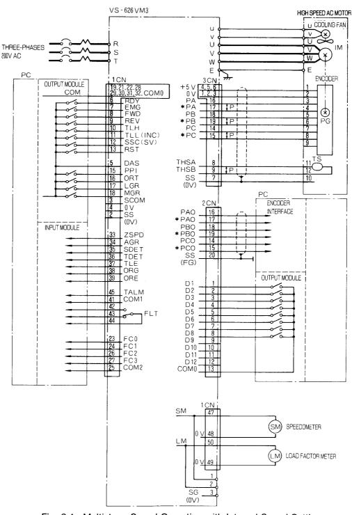
Fig. 8.4 Multistage Speed Operation with Internal Speed Setting
