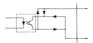
Fig. 4.23 Output Interface Circuit
