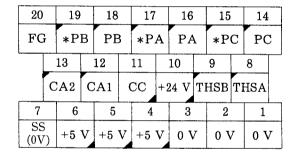
PCB Side Connector; MR-20RFAG Cable Side Connector; MR-20LM (G)
