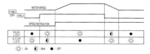
Note: RUN and STOP LEDs light, blink, and go OFF depending on the status of operation.
