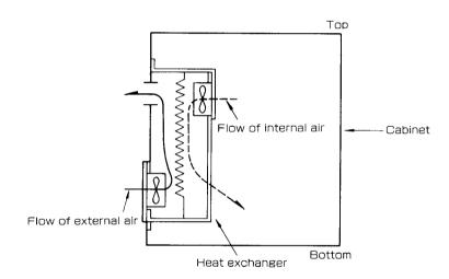
Fig. 7.20 Example of Installation of Heat Exchanger
