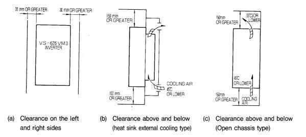
Fig. 11.3 Inverter Installation Space
