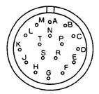
Main unit side MS3102A20-29P Cable side MS3108A20-29S
