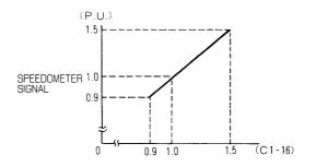
C1-16 = actual motor speed/indication on speedometer
