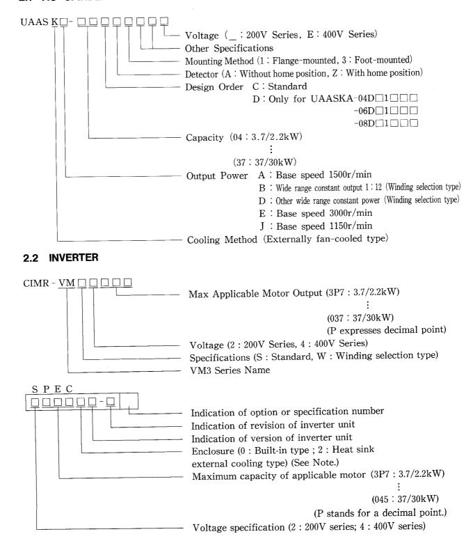
Note: The built-in type is mounted directly on the side or back of the control panel using the heat sink cover on the back of the inverter. The heat sink external cooling type is mounted with the heat sink exposed to the outside by drilling / cutting a hole of specified dimensions in the control panel. To use this type, an air duct must be prepared for cooling the heat sink.
