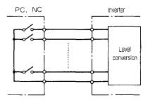
Fig. 7.16 Example of Analog Speed Reference Signal
