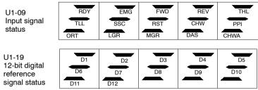
Notes: 1. The LED lights to indicate that the corresponding input signal is ON.
