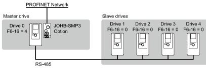
Figure 8.1 Gateway Mode Setup
