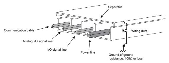
Fig. C.5 Wiring Example via a Wiring Duct
