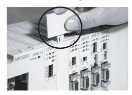
Release the hook on the bottom in the same way and remove the Option Cover.
