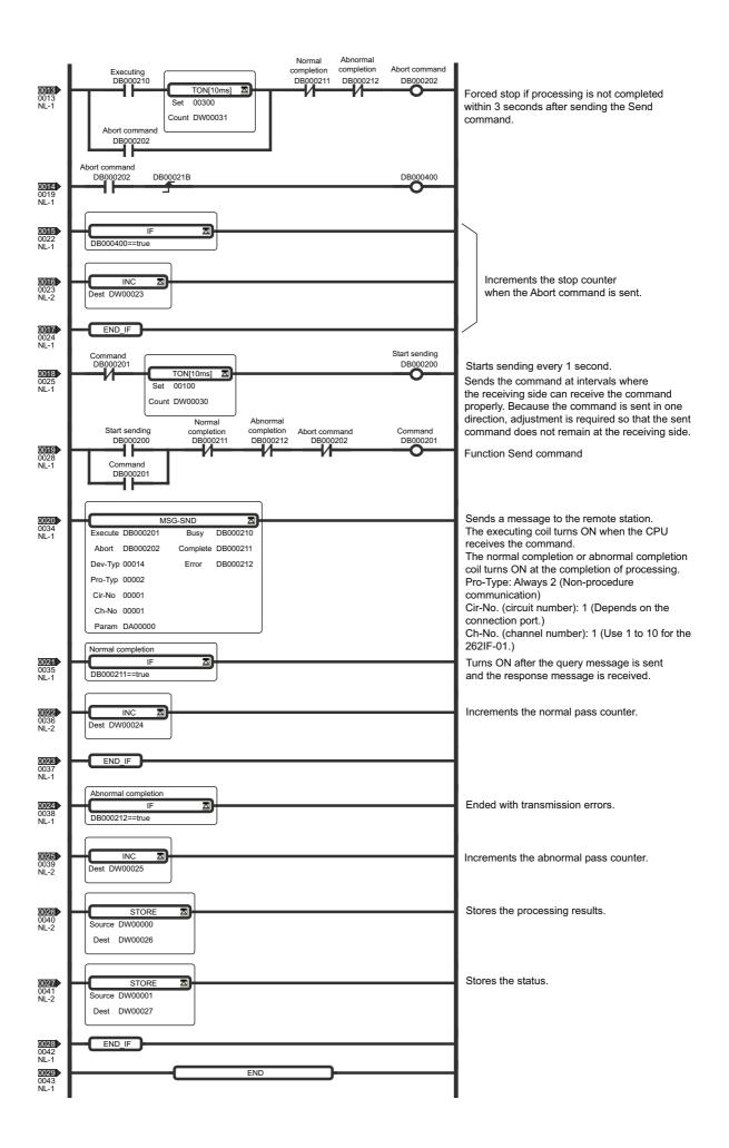
As for FL-net messages other than transparent messages, the MSG-RCV function must be started to receive a response message after message request was sent by the MSG-SND function.
