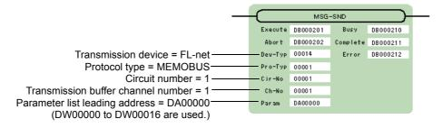
To use the Extended MEMOBUS protocol, the protocol type is set to MEMOBUS. The circuit number is set to the circuit number assigned to the 262IF-01 transmission device. Transmission buffer channel numbers in the same line must all be unique. For details on the settings, refer to *6.1.3 Inputs and Outputs for the Message Send Function* on page 6-3.
