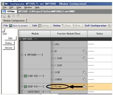
In Online Mode, the FL-net transmission definitions data saved in the Machine Controller are displayed. In Offline Mode, the definitions data saved in the personal computer on which MPE720 is running is displayed. The FL-net Transmission Configuration Window is composed of four tab pages: Transmission Parameters, Link Assignment, Link Status, and Status. These tab pages are used to set the definitions and monitor the settings.
