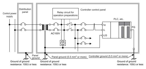
Fig. C.3 Example of Power Supply Wiring and Grounding in FL-net System
