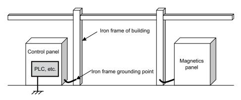
Fig. C.2 Example 2 of Grounding a Controller Control Panel (Grounding Controller Alone with Ground Resistance of  $100\Omega$  or less)
