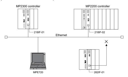
(2) The MPE720 engineering tool cannot be connected to the 262IF-01 directly. When connecting the MPE720, separately prepare a module with any of the RS232C, Ethernet, and CP-215 ports for connection.
