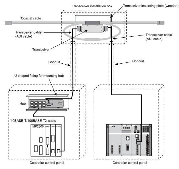
Fig. C.4 Example of Network Equipment Connection in the FL-net System
