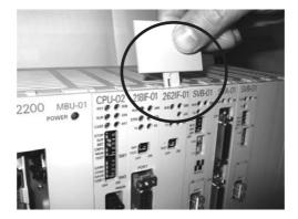
Release the hook on the bottom in the same way and remove the option panel.
