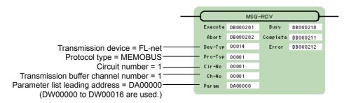
To use the Extended MEMOBUS protocol, the protocol type is set to MEMOBUS. The circuit number is set to the circuit number assigned to the 262IF-01 transmission device. Transmission buffer channel numbers in the same line must all be unique. For details on settings, refer to *6.2.3 Inputs and Outputs for the Message Receive Function* on page 6-18.
