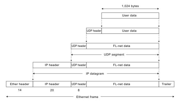
Next, the following shows FL-net data (of one frame) that can be observed on communication lines. In this example, 128-byte cyclic data is transferred.
