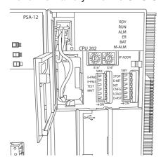
5. Close the cover on the CPU Unit, you turn ON the power supply, and then confirm that the BAT indicator on the CPU Unit is not.
