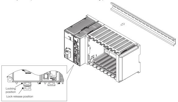
4. Place end plates on both sides of the MP3200 to secure it to the DIN rail.
