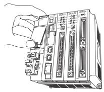
**3.** Securely connect the lead connector of the Battery to the connector in the Base Unit, and insert the Battery into the battery holder.
