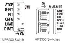
**4.** Set the INIT pin on the mode switch 1 on the CPU Unit/CPU Module according to the register type to load.
