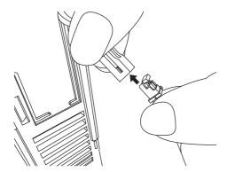
4. Press the connector back into the CPU Unit.
