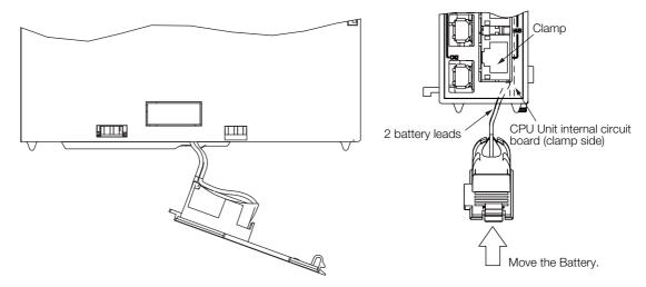
6. Close the battery holder and confirm that the BAT indicator on the CPU Unit is not lit.
