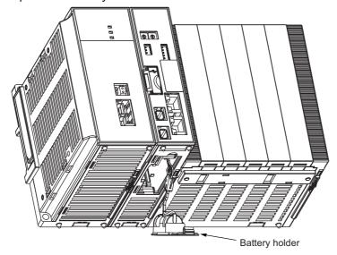
4. Remove the connector on the end of the Battery lead from the connector on the CPU Unit.
