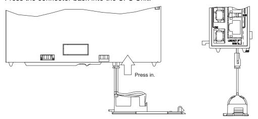
9. Hold the connector, and while pressing it toward the CPU Unit's internal circuit board (the board on the side of the clamp), move the Battery and the battery holder into the CPU Unit.
