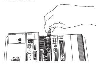
**6.** Hold the Optional Module at the top and bottom and pull it straight out. Hold the edges of the Module and avoid touching the components on the Module.
