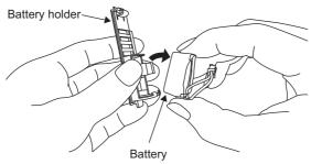
6. Insert the Replacement Battery into the battery holder.
