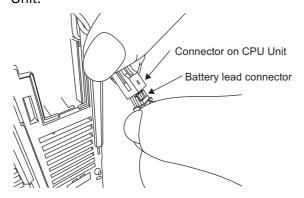
5. Remove the Battery from the battery holder.
