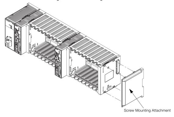
2. In the same way as when mounting to DIN rail, use the rail locks to secure the Rack Support Bracket.
