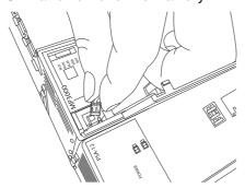
5. Securely connect the lead connector of the replacement Battery to the connector on the CPU Unit and attach the replacement Battery.
