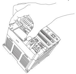
3. Insert the protruding part of the battery cover into the slot on top of the Optional Module panel to unhook the tab. Face the front of the battery cover toward you for this operation.
