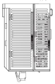
3. Secure the connection by locking the slide locks at both the top and the bottom.
