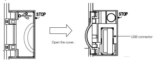
2. Insert the USB memory device into the USB connector.
