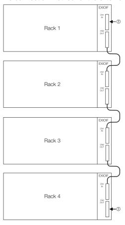
Note: Attach the enclosed dust caps to the unused connectors (① in the above figure).
