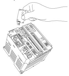
5. Hold the center of the battery cover, and turn it around the round knob while pushing it toward the back to disconnect the Module from the Mounting Base connectors. Then, pull the Module forward.
