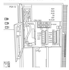
7. Close the cover on the CPU Unit and confirm that the BAT indicator on the CPU Unit is not lit.
