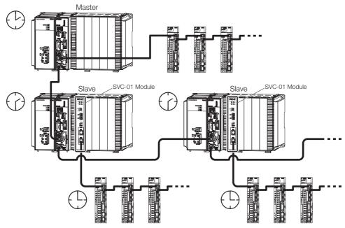
Note: A delay will occur in MECHATROLINK-III communications until the references from the application program in the master reach the slaves. Therefore, the operation of the SERVOPACKs connected to the master will not be synchronized with the operation of the SERVOPACKs connected to the slaves.
