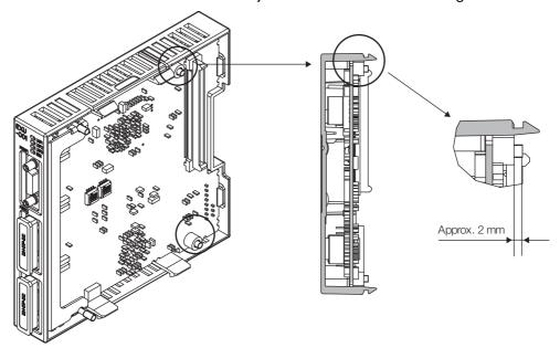
2. As shown in the following figure, insert the four latches (top and bottom) on the Rack Expansion Interface Unit into the Power Supply Unit to mount the Rack Expansion Interface Unit.
