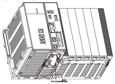
3. Securely connect the lead connector of the Battery to the connector in the CPU Unit.
