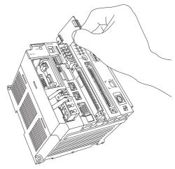
**6.** Hold the Optional Module at the top and bottom and pull it straight out. Hold the edges of the Module and avoid touching the components on the Module.
