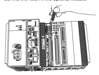
5. Hold the center of the tool, and turn it around the round knob while pushing it toward the back to disconnect the Module from the Mounting Base connectors. Then, pull the Module forward.
