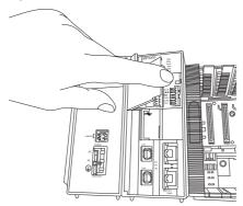
3. Securely connect the lead connector of the Battery to the connector in the CPU Unit.
