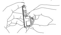
7. Securely connect the lead connector of the Replacement Battery to the connector on the CPU Unit.
