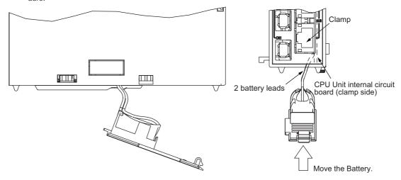
10. Close the battery holder and confirm that the BAT indicator on the CPU Unit is not lit.
