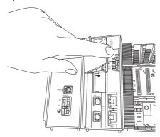
**4.** Remove the connector on the end of the Battery lead from the connector on the CPU Unit and remove the Battery.
