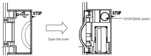
Note: Press and hold this switch for at least 2 seconds to save all of the data to the USB memory. The display will show the progress of saving.
