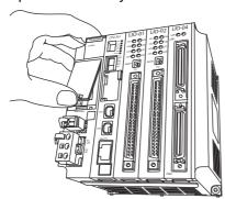
4. Disconnect the lead connector of the Battery from the connector on the Base Unit, and remove the Battery from the battery holder.
