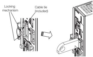
4. Use the cable tie to secure the USB memory into place.
