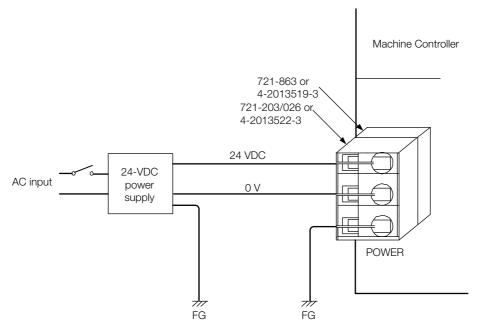
Note: Use an isolating 24-VDC power supply, and install the power supply switch on the AC side of the power supply. If the switch is installed on the 24-VDC side, the inrush current may reach approx. 40 A when the power is turned ON.
