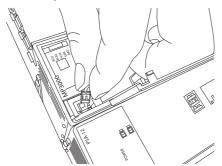
4. Move the Battery into the CPU Unit.
