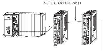
To prevent communications errors, confirm that the connectors are properly inserted.
