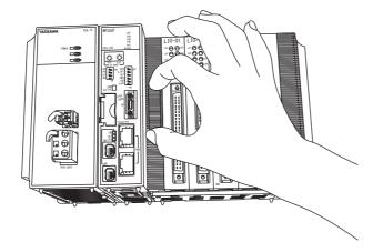
3. Insert the protruding part of the tool into the slot on top of the Optional Module panel to unhook the tab.
