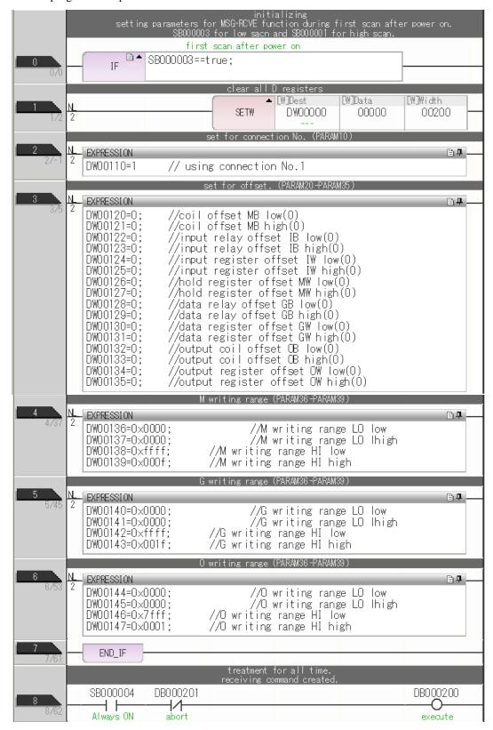
Using the MSG-RCVE Function with the MP3000 as a Slave
