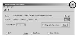
**8.** Open the transfer destination folder to confirm that the .mal file has been created.
