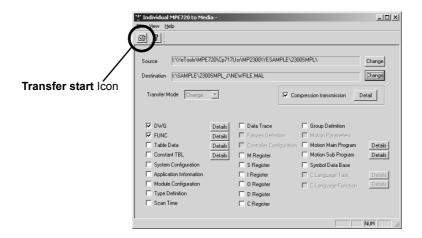
A confirmation message will be displayed. Click the **Yes** Button to start transfer. When the transfer is complete, the **Individual MPE720 to Media** Dialog Box will be displayed again.
