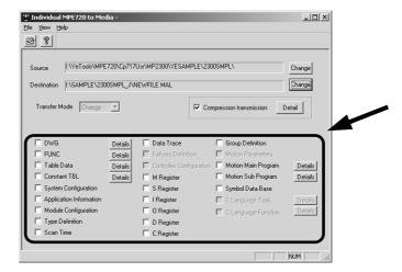
For check boxes with a Details Button, click this button to set the details of the data to be transferred.
