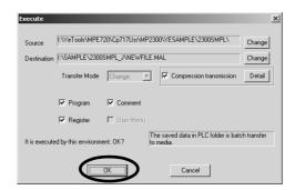
The transfer will start. When the transfer is complete, the All MPE720 to Media Dialog Box will be displayed.
