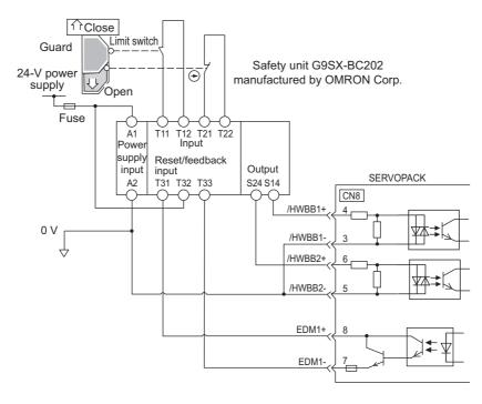
When a guard opens, both of signals, the /HWBB1 and the /HWBB2, turn OFF, and the EDM1 signal turns ON. Since the feedback is ON when the guard closes, the safety unit is reset, and the /HWBB1 and the /HWBB2 signals turn ON, and the operation becomes possible.
