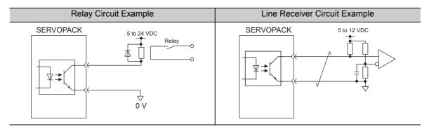
Note: The maximum allowable voltage and current range of the photocoupler output circuit are as follows:
