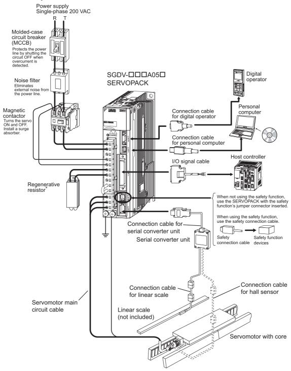
\* Before connecting an external regenerative resistor to the SERVOPACK, refer to 3.6 Connecting Regenerative Resistors.
