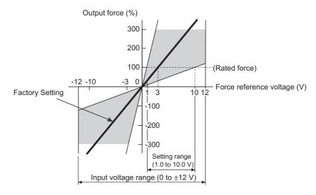
Note: A force reference above the rated force can be applied but it may cause an overload (high load) alarm (A.710) or overload (low load) alarm (A.720) if excessive force is output for a long time. Refer to 9.1.2 Troubleshooting of Alarms.
