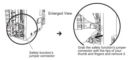
**2.** Connect the safety function device to the safety connector (CN8).
