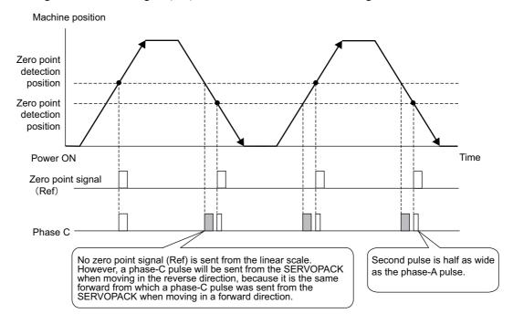
• Passing First Zero Point Signal (Ref) in Reverse Direction and Returning after Power ON
