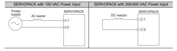
Note 1. Connection terminals for DC reactor  $\ominus 1$  and  $\ominus 2$  are short-circuited at shipment. Remove the lead wire for short-circuit, and connect a DC reactor.
