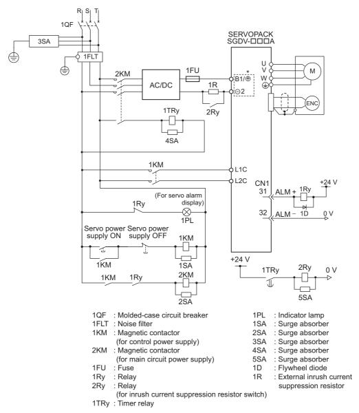
\* Terminal names differ depending on model of SERVOPACK. Refer to (2) DC Power Supply Input Terminals for the Main and Control Circuits.
