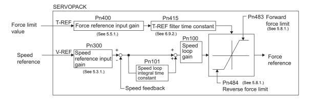
There is no polarity in the input voltage of the analog voltage reference for force limiting. The absolute values of both + and - voltages are input, and a force limit value corresponding to that absolute value is applied in the forward and reverse direction.
