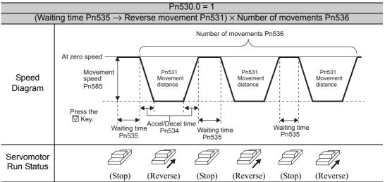
Note: When Pn536 (Number of Times of Program JOG Movement) is set to 0, infinite time operation is enabled. To stop infinite time operation, press the MODE/SET Key (or JOG/SVON Key of digital operator) to turn the servomotor power OFF.
