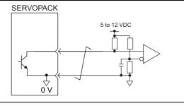
Note: The maximum allowable voltage and current of the open-collector output circuit are as follows:
