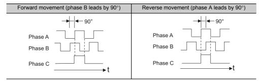
Note: The pulse width for phase C (origin pulse) changes according to the setting of the encoder output resolution (Pn281) and becomes the same as that for phase A.
