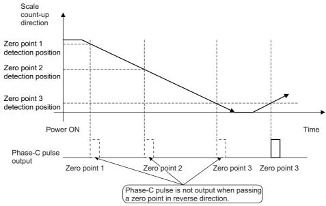
To output the encoder dividing phase-C pulse when moving in the reverse direction, set Pn081 to n.□□□1.
