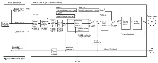
st The reference pulse input multiplication switching function is supported by software version 001A or later.
