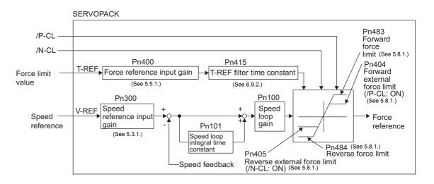
Note: This function cannot be used during force control since the force limit by analog voltage reference is input from T-REF (CN1-9, 10).
