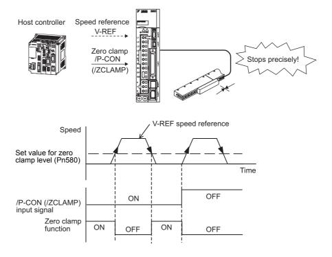
Adjust the position loop gain (Pn102) if the servomotor oscillates in the zero clamp state. If the gain switching function is used, adjusting the 2nd position loop gain (Pn106) is required as well. For details, refer to 6.8.1 Switching Gain Settings.
