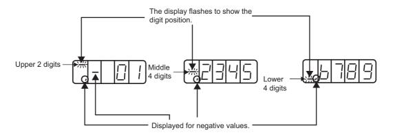
The number of pulses between -2147483648 and 2147483647 is displayed continuously. When the number of pulses is outside this range, the display will change as follows:
