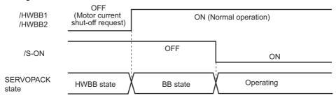
If the /HWBB1 and /HWBB2 signals are OFF and the servo ON signal is ON, the HWBB state will be maintained after the /HWBB1 and /HWBB2 signals are turned ON.
