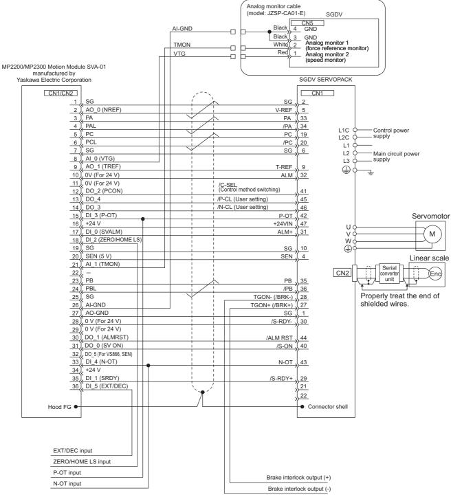
Note 1. Connection cables (model: JEPMC-W2040-□□) to connect the SERVOPACK to the MP2200/MP2300 are prepared by Yaskawa. For details, refer to the *Machine Controller MP2000 Series SVA-01 Motion Module USER'S MANUAL* (Manual No.: SIEP C880700 32).
