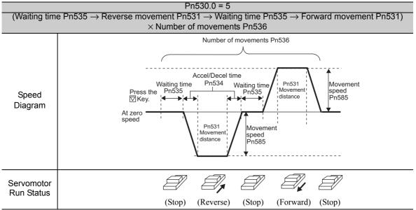
Note: When Pn536 (number of times of program JOG movement) is set to 0, infinite time operation is enabled. To stop infinite time operation, press the MODE/SET Key (or JOG/SVON Key of digital operator) to turn the servomotor power OFF.
