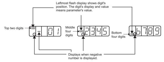
The example below shows how to set the positioning completed width (Pn522) to "0123456789."
