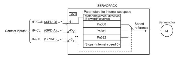
\* When using the external input signal pins as factory settings, the functions of /P-CON, /P-CL, and /N-CL change to the functions of /SPD-D, /SPD-A, and /SPD-B, respectively.
