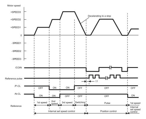
Note 1. The t1 value is not affected by whether the soft start function is used. A maximum delay of 2 ms occurs in loading /P-CL and /N-CL.
