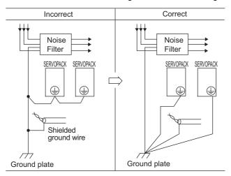
If a noise filter is located inside a control panel, first connect the noise filter ground wire and the ground wires from other devices inside the control panel to the ground plate for the control panel, then ground the plates.
