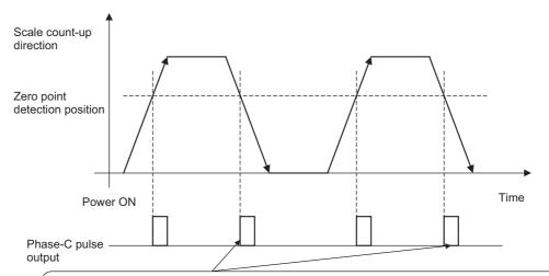
The phase-C pulse is also output when the detection head of the linear scale passes this point in reverse, because the SERVOPACK has recorded the position where the phase-C pulse was originally output when first passing the position in the forward direction.
