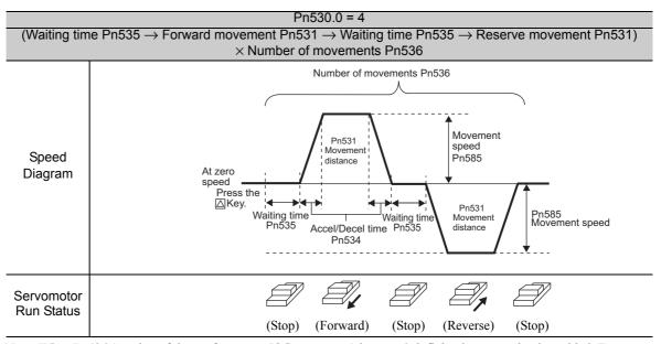
Note: When Pn536 (number of times of program JOG movement) is set to 0, infinite time operation is enabled. To stop infinite time operation, press the MODE/SET Key (or JOG/SVON Key of digital operator) to turn OFF the servomotor power.
