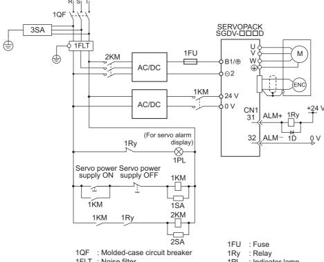
KM : Magnetic contactor(for main circuit power supply)3SA : Surge absorber1D : Flywheel diode
