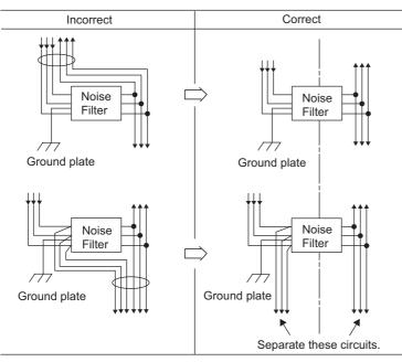
Separate the noise filter ground wire from the output lines. Do not accommodate the noise filter ground wire, output lines and other signal lines in the same
