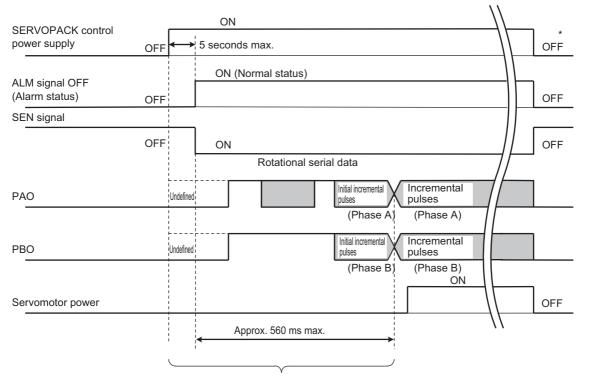
The servomotor will not be turned ON even if /S-ON is turned ON during this interval. \* Turn OFF the SEN signal to turn OFF the control power supply.
