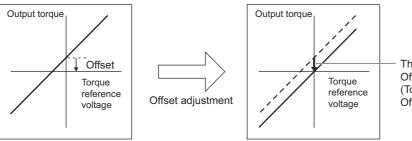
The offset is adjusted in the SERVOPACK. Offset Adjustment Range: -127 to +127 (Torque Reference: -1905 mV to 1905 mV Offset Setting Unit: 15.0 mV)
