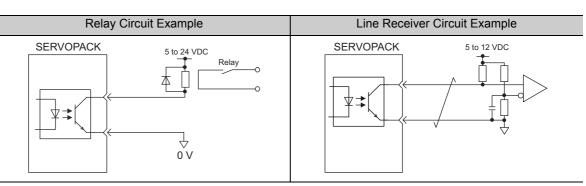
Note: The maximum allowable voltage and the allowable range of current capacity for photocoupler output circuits are as follows.
