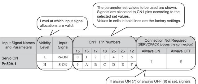
If always ON (7) or always OFF (8) is set, signals will be processed in the SERVOPACK, which will eliminate the need for wiring changes. 3.3.1 Input Signal Allocations
