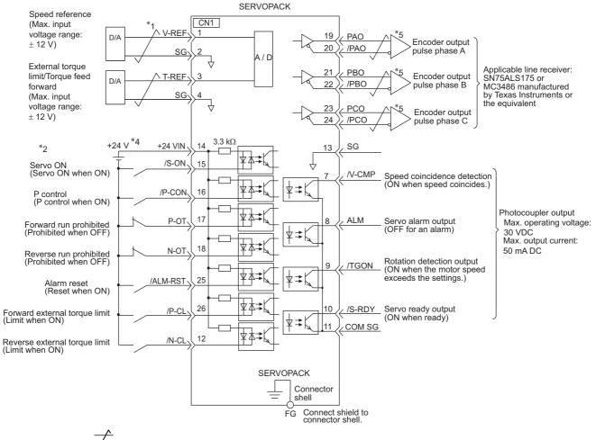
Connection example in speed control is as shown below.
