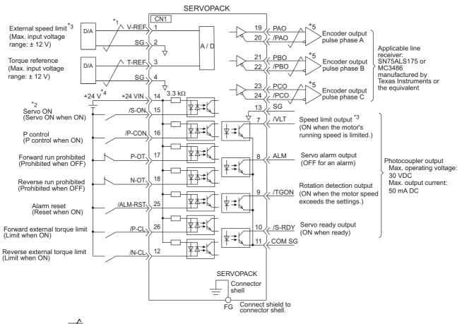
Connection example in torque control is as shown below.
