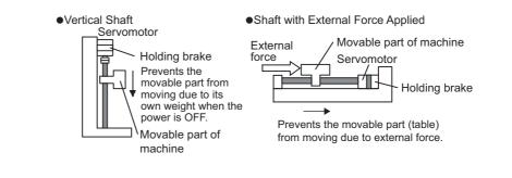
The brake built into the servomotor with brakes is a de-energization brake, which is used only to hold and cannot be used for braking. Use the holding brake only to hold a stopped servomotor.
