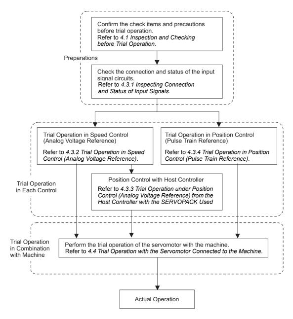
Note: To perform trial operation of a servomotor with a brake, refer to 4.5 Trial Operation of Servomotor with Brakes.
