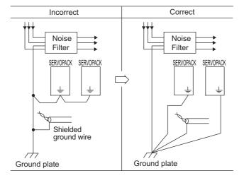
Connect the noise filter ground wire directly to the ground plate. Do not connect the noise filter ground wire to other ground wires.
