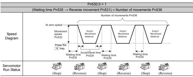
Note: When Pn536 (Number of Times of Program JOG Movement) is set to 0, infinite time operation is enabled. To stop infinite time operation, press the JOG/SVON Key of digital operator to turn OFF the servomotor power.
