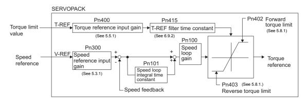
There is no polarity in the input voltage of the analog voltage reference for torque limiting. The absolute values of both + and - voltages are input, and a torque limit value corresponding to that absolute value is applied in the forward and reverse direction.
