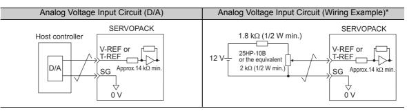
\* This wiring example is for forward operation.
