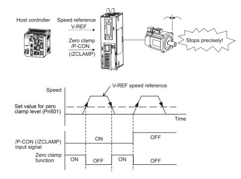
Adjust the position loop gain (Pn102) if the servomotor oscillates in the zero clamp state. If the gain switching function is used, adjusting the 2nd position loop gain (Pn106) is required as well. For details, refer to 6.8.1 *Switching Gain Settings*.
