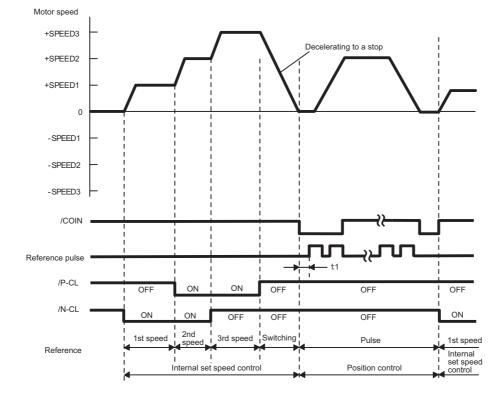
The following diagram describes an operation example for internal set speed control + soft start <=> position control.
