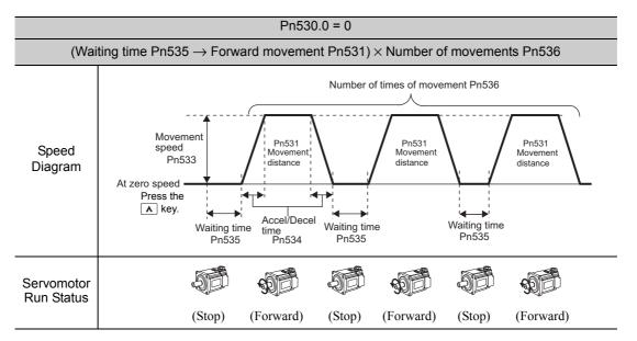
Note: When Pn536 (number of times of program JOG movement) is set to 0, infinite time operation is enabled. To stop infinite time operation, press the JOG/SVON Key of digital operator to turn OFF the servomotor power.
