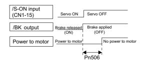
• This parameter changes the brake ON timing while the servomotor is stopped.
