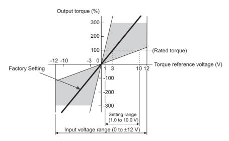
Note: A torque reference above the rated torque can be applied but it may cause an overload (high load) alarm (A.710) or overload (low load) alarm (A.720) if excessive torque is output for a long time. Refer to 9.1.2 Troubleshooting of Alarms.
