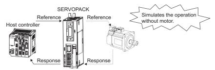
Use Pn00C.0 to enable or disable the test without a motor.
