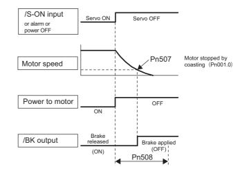
• The servomotor will be limited to its maximum speed even if the value set in Pn507 is higher than the maximum speed.
