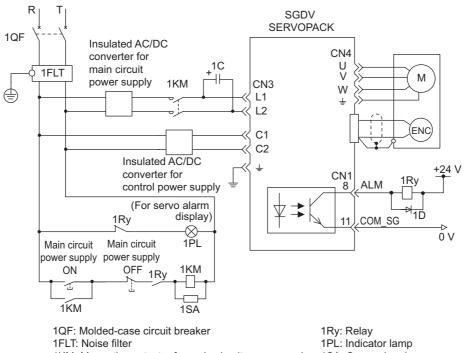
1KM: Magnetic contactor for main circuit power supply 1C: Capacitor (for main circuit power supply) 1SA: Surge absorber 1D: Flywheel diode
