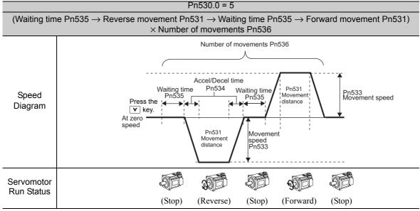
Note: When Pn536 (number of times of program JOG movement) is set to 0, infinite time operation is enabled. To stop infinite time operation, press the JOG/SVON Key of digital operator to turn OFF the servomotor power.
