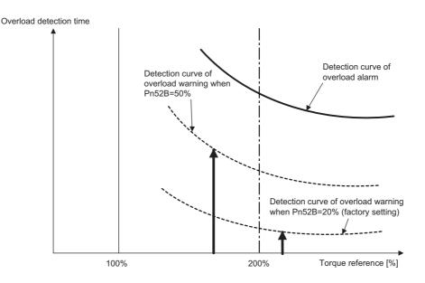
Note: For details, refer to Overload Characteristics listed in the section for the relevant servomotor in the Σ-V Series Product Catalog (Catalog No.: KAEP S80000 42).
