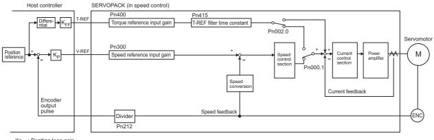
Kp : Position loop gain K<sub>FF</sub> : Feedforward gain
