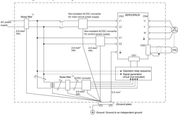
The following is an example of wiring for noise control.
