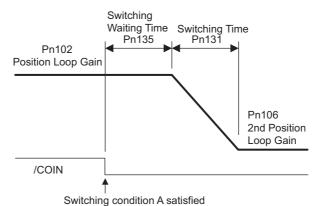
Note: Automatic gain switching is available in the PI and I-P controls (Pn10B).
