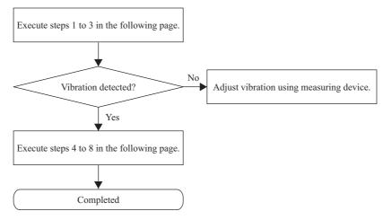
6.7.2 Vibration Suppression Function Operating Procedure
