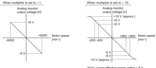
Note: Linear effective range: within ± 8 V Output resolution: 16-bit
