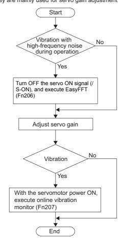
How to use EasyFFT (Fn206) and online vibration monitor (Fn207), when they are mainly used for servo gain adjustment.
