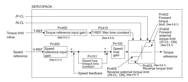
Note: This function cannot be used during torque control since the torque limit by analog voltage reference is input from T-REF (CN1-3, 4).
