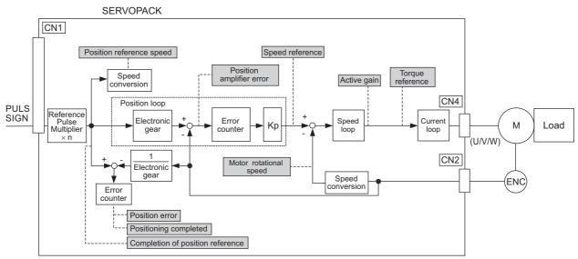
The following signals can be monitored by selecting functions with parameters Pn006 and Pn007. Pn006 is used for analog monitor 1 and Pn007 is used for analog monitor 2.
