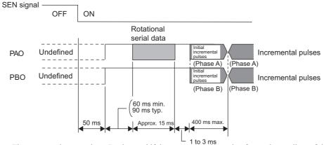
Note: The output pulses are phase-B advanced if the servomotor is turning forward regardless of the setting in Pn000.0.
