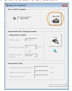
5. Select the instruction (reference) amplitude and the rotation direction in the Measurement condition Area, and then click the Start Button.
