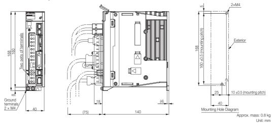
Three-Phase, 200 VAC: SGD7S-2R8A; Single-Phase, 100 VAC: SGD7S-R70F, -R90F, and -2R1F
