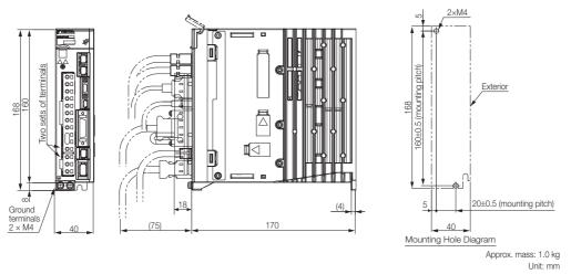
• Three-Phase, 200 VAC: SGD7S-3R8A, -5R5A, and -7R6A; Single-Phase, 100 VAC: SGD7S-2R8F
