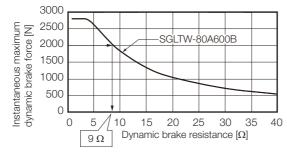
The following figures show the relationship between the instantaneous maximum dynamic brake torque and dynamic brake resistance of the Servomotor.
