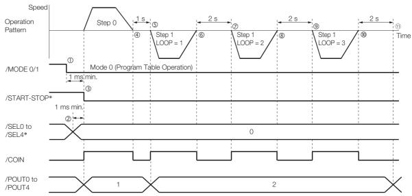
$<sup>\</sup>boldsymbol{*}$  Do not change /SEL0 to /SEL7 for 4 ms after turning ON the /START-STOP signal.
