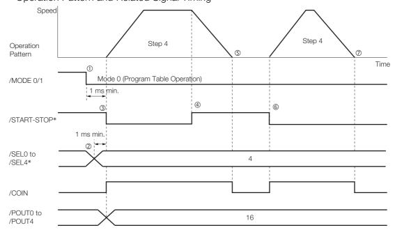
$<sup>\</sup>ast$  Do not change /SEL0 to /SEL7 for 4 ms after turning ON the /START-STOP signal.
