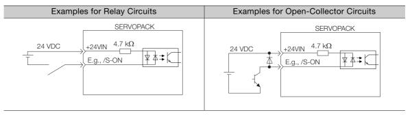
Note: The 24-VDC external power supply capacity must be 50 mA minimum.
