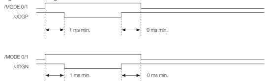
If you have performed homing, turn OFF the /HOME signal, wait for at least 1 ms, and then turn ON the /JOGP or /JOGN signal. When performing jog operation in both directions, allow at least 1 ms between the /JOGP and /JOGN signals. The timing is shown below.
