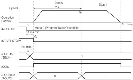
$<sup>\</sup>ast$  Do not change /SEL0 to /SEL7 for 4 ms after turning ON the /START-STOP signal.
