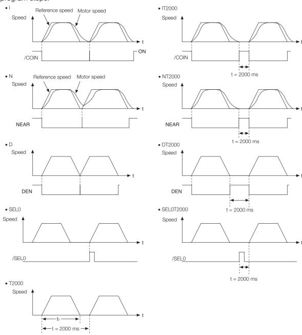
Note: If  $t < t_1$ , an error (E53E) will occur and program table operation will be stopped.
