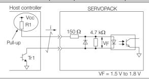
This section describes CN1 connector terminals 40 to 47. The circuits are connected through relay or open-collector transistor circuits. If you connect through a relay, use a low-current relay, If you do not use a low-current relay, a faulty contact may result.
