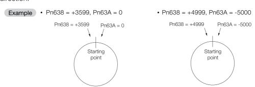
If a rotary table or other device with rotational coordinates is used, but multiturn operation is not possible, use linear coordinates (Pn637 =  $n.\Box\Box\Box\Box$ 0). In this case, Pn638 and Pn63A are for software limits.
