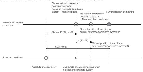
When using the linear type coordinate (Pn637 =  $n.\Box\Box\Box\Box$ 0), set the calculated value in Pn63C.
