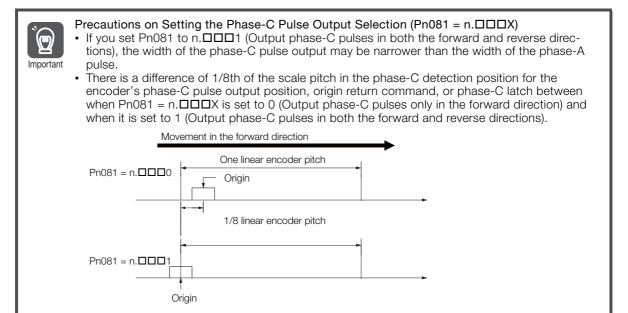
Observe the following precaution if you set Pn081 to n. \$\square\$ (Output phase-C pulses only in the forward direction).
