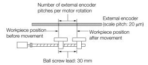
If the external encoder is connected directly to the Servomotor, the setting will be 1,500 (30 mm/0.02 mm = 1,500).
