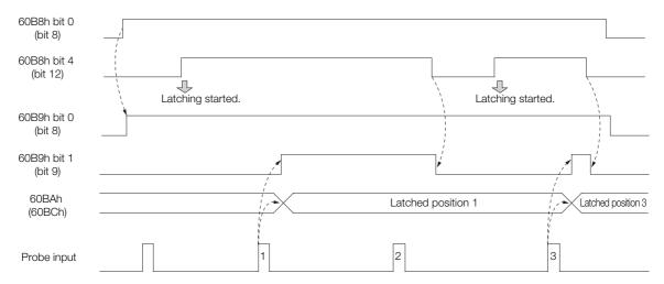
• Continuous Trigger Mode (60B8h bit 1 = 1 or bit 9 = 1)
