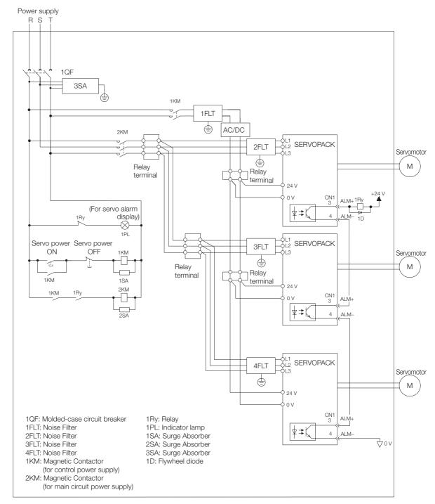
To comply with UL/cUL standards, you must install a branch circuit protective device at the power supply input section to each SERVOPACK. Refer to the following document for details.  $\Sigma$ -7-Series  $\Sigma$ -7S and  $\Sigma$ -7W SERVOPACK with 400 V-Input Power Safety Precautions (Manual No.: TOMP C710828 02)
