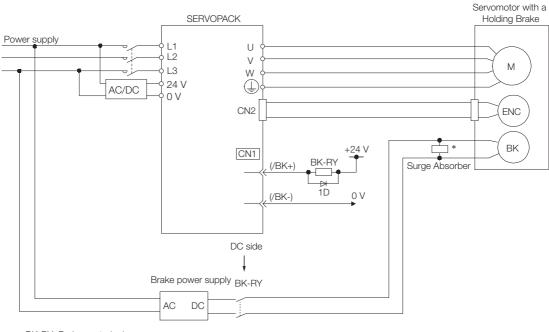
BK-RY: Brake control relay 1D: Flywheel diode
