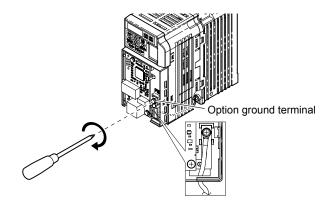
Figure 17 Connect the Ground Wire to the Option
