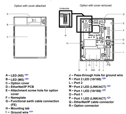
Figure 1 Option Unit Components
