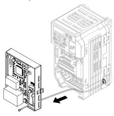
Figure 15 Ground Wire Routing
