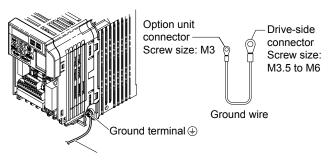
Figure 7 Connect the Ground Wire on an IP20/Open-Chassis Drive
