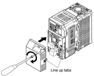
Figure 21 Attach the Option Cover
