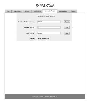
Figure 27 Parameter Access Tab View
