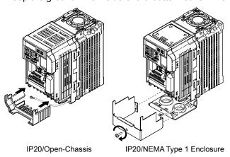
Figure 12 Reattach the Bottom Cover
