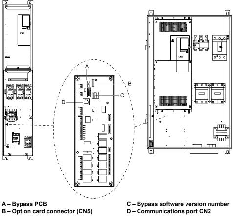
Figure 4 Front View of Bypass PCB
