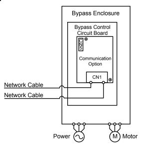
Figure 13 Option Connection Diagram (Dual Port CN1 Connection)
