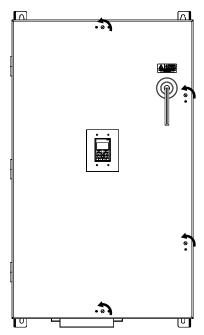
Figure 9 Turn Front Cover Fasteners
