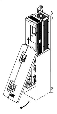
Figure 7 Lift and Remove Front Cover
