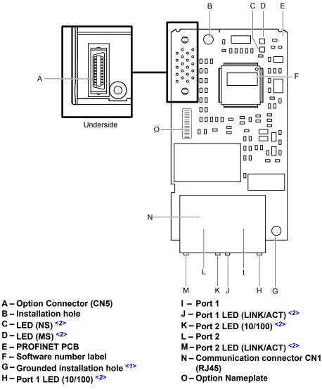
**Figure 3 PROFINET Option Components**
