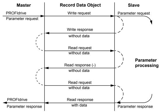
Figure 16 PROFIdrive Acyclic Parameter Access Mechanism Structure
