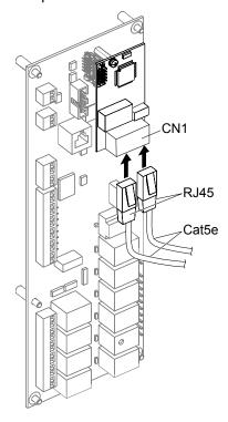
Figure 12 Connect Network Cables to Option
