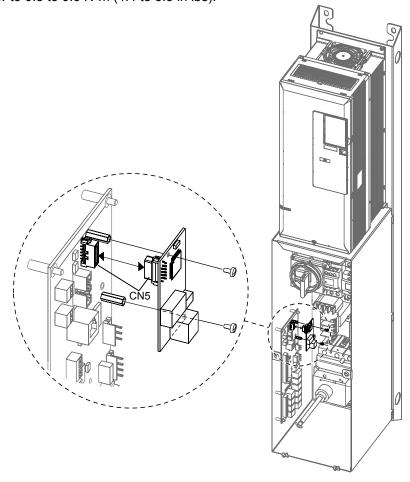
Figure 11 Insert Option into Bypass PCB CN5 Connector Port - Model Z1B1D002
