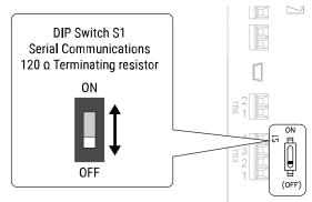
Figure 10.3 Termination Resistor DIP Switch S1
