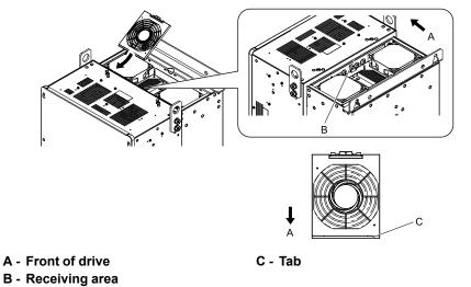
Figure 8.51 Install the Fan Finger Guard
