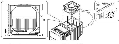
A - Notch on fan C - Front of drive B - Alignment pin on drive
