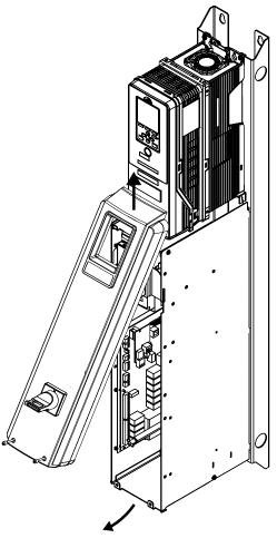
Figure 2.13 Remove the Front Cover
