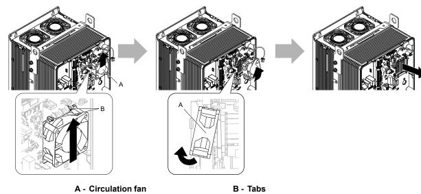
Figure 8.35 Remove the Circulation Fan
