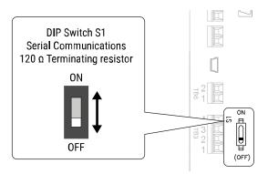
Figure 10.12 Termination Resistor DIP Switch S1
