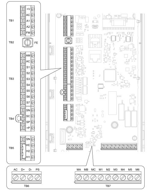
Figure 3.14 Drive Control Circuit Terminal Arrangement
