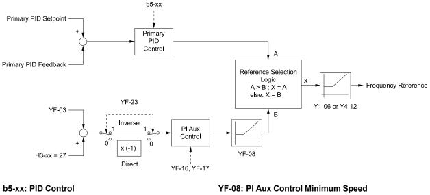
b5-xx: PID Control H3-xx = 27: PI Auxiliary Control Feedback Y1-06: Minimum Speed Y4-12: Thrust Frequency YF-03: PI Aux Control Setpoint YF-08: PI Aux Control Minimum Speed YF-16: PI Auxiliary Control P Gain YF-17: PI Auxiliary Control I Time YF-23: PI Aux Ctrl Output Level Select
