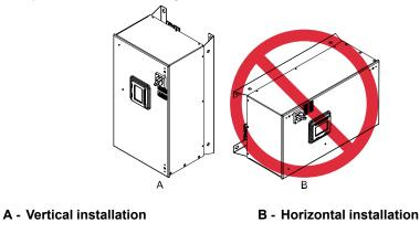
Figure 2.3 Installation Position
