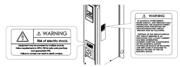
Figure i.2 Narrow Bypass Warning Labels and Locations
