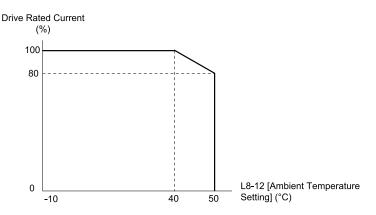
Figure 7.2 Derating for Side-by-Side Mounting (L8-35 = 1)
