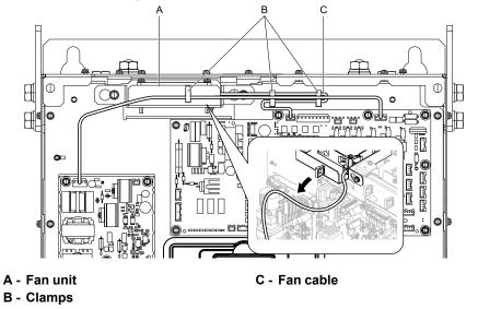
Figure 8.53 Remove the Fan Cables
