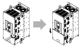
Figure 2.23 Loosen the Terminal Cover Mounting Screws
