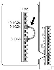
Figure 10.5 Self-Diagnostics Jumper Terminals
