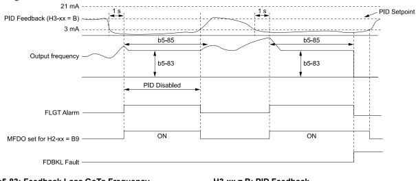
b5-83: Feedback Loss GoTo Frequency b5-85: Feedback Loss GoTo Freq Timeout b5-86: Feedback Loss Start Delay H2-xx = B9: Transducer Loss H3-xx = B: PID Feedback FDBKL Fault: WIRE Break FLGT Alarm: Feedback Loss, Go To Freq b5-83
