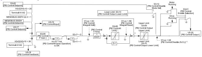
Figure 5.94 PI2 Control Block Diagram
