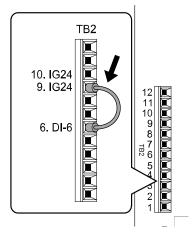
Figure 10.9 Self-Diagnostics Jumper Terminals
