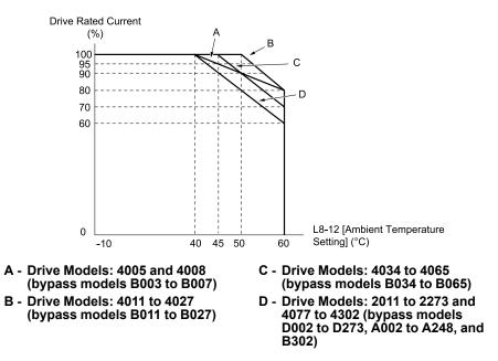
Figure 7.3 Derating for IP20/UL Type 1 (L8-35 = 2)
