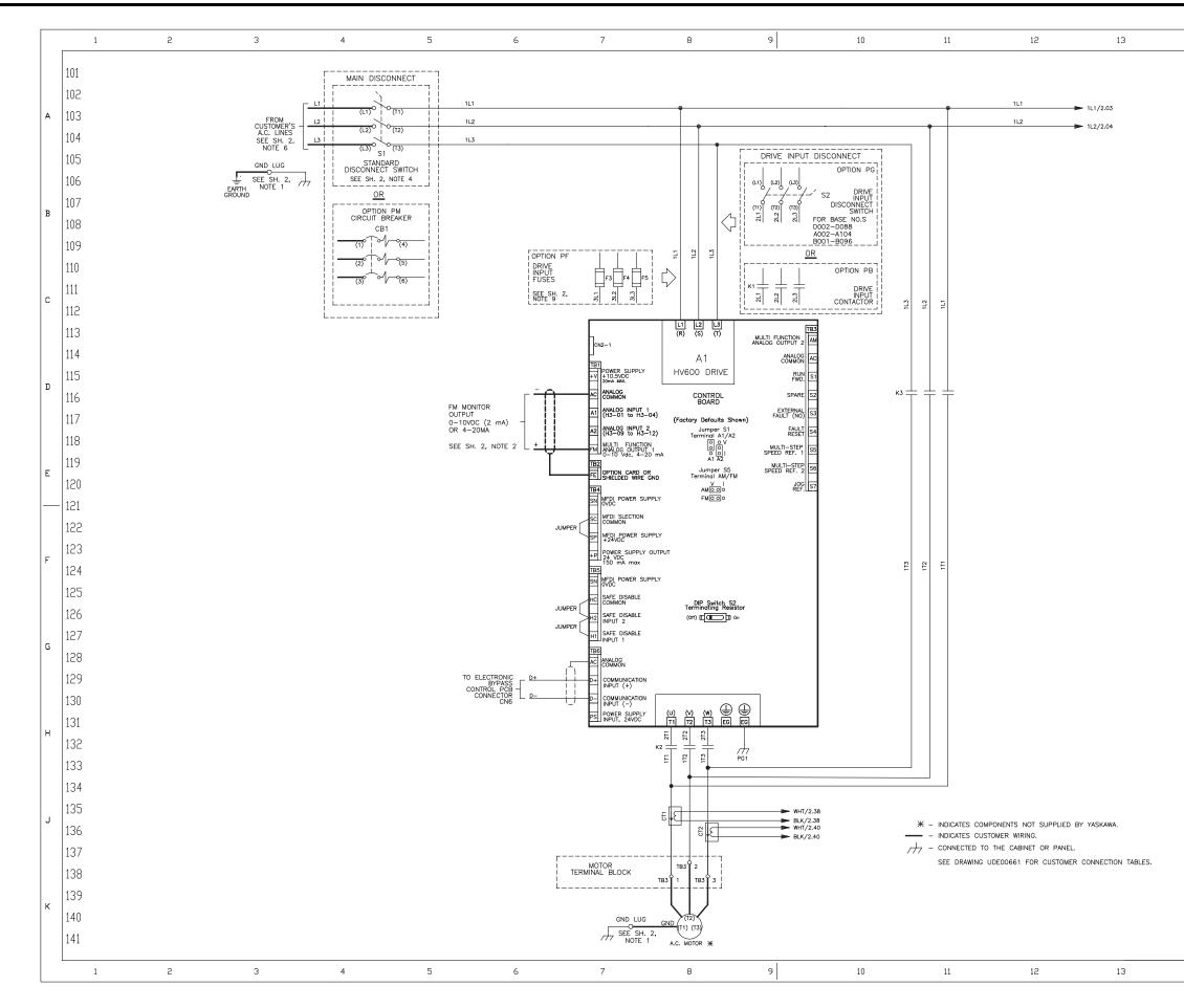
Figure 3.2 Standard Enclosed Bypass Connection Diagram
