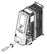
Figure 2.16 Reattach the Front Cover
