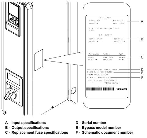
Figure 1.1 Narrow Bypass Nameplate Location Example
