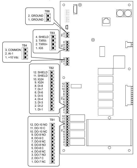
Figure 3.9 Bypass Control Circuit Terminal Arrangement
