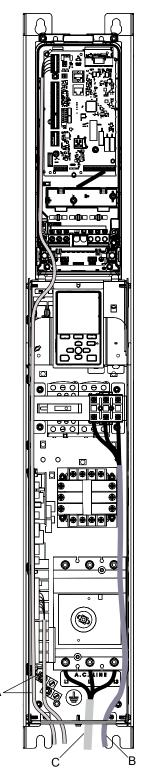
A - Optional drive control wiringC - Main input circuitB - Motor output circuit
