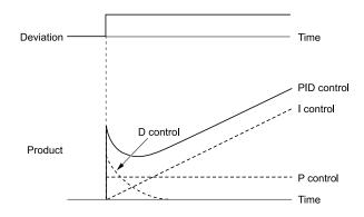
Figure 5.22 PID Control Operation
