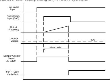
Figure 5.109 Motor Disconnected at Start
