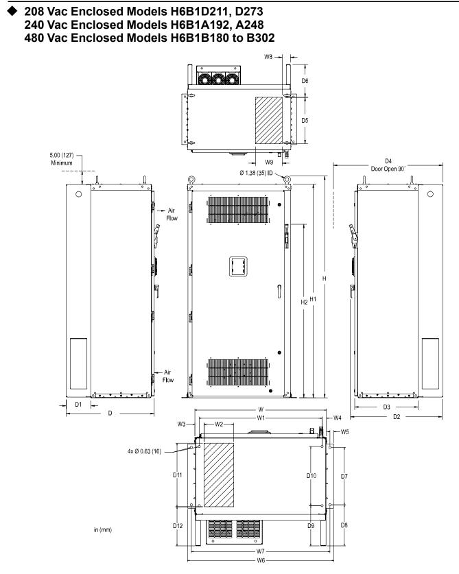
Figure 2.34 Enclosed Exterior and Mounting Dimensions Diagram
