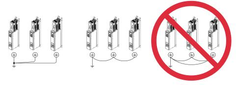
Figure 3.5 Wiring More than One Bypass
