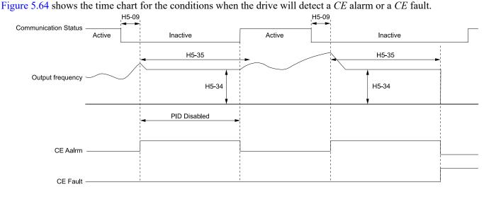
H5-09: CE Detection Time H5-34: Comm Error (CE) Go-To-Frequency H5-35: Comm Error (CE) Go-To-Timeout CE Alarm: Run at H5-34 (CE Go-To-Freq) CE Fault: Serial Communications Error
