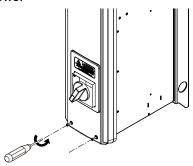
Figure 2.12 Loosen the Front Cover Screws
