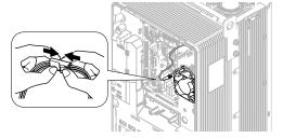
Figure 8.37 Connect the Power Supply Connector
