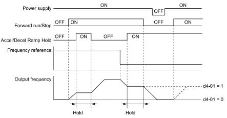
Figure 5.36 Frequency Reference Hold with Accel/Decel Hold Function
