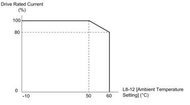
Figure 7.1 Derating for IP20/UL Open Type (L8-35 = 0)
