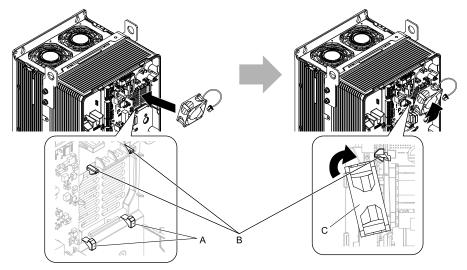
A - Tabs at the bottom of the fan C - Circulation fan B - Tabs at the top of the fan
