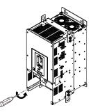
Figure 2.26 Loosen the Front Cover Screws
