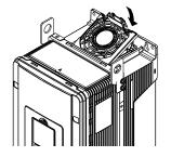
Figure 8.19 Install the Fan Finger Guard
