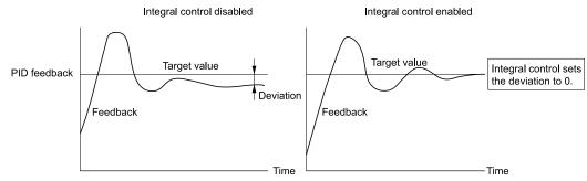
Figure 5.25 Integral Time and Deviation
