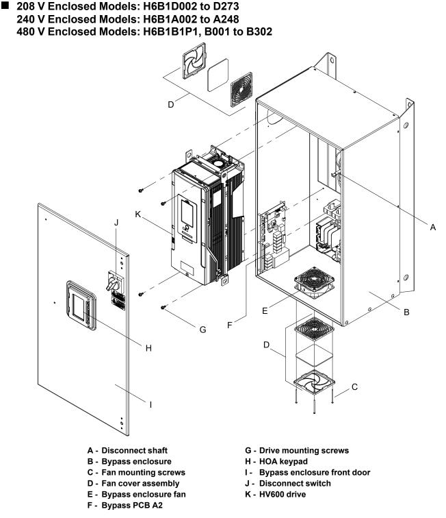
Figure 2.7 Exploded View of Components (Enclosed Model D046 Example)
