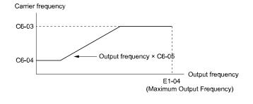
C6-03: Carrier Frequency Upper Limit C6-04: Carrier Frequency Lower Limit
