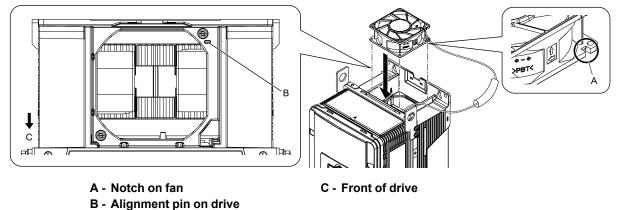
Figure 8.16 Install the Cooling Fan
