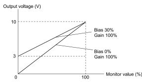
Figure 5.63 Analog Output Gain/Bias Configuration Example 2
