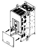
Figure 2.31 Reattach the Terminal Cover
