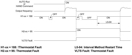
Figure 5.82 Thermostat Fault Behavior
