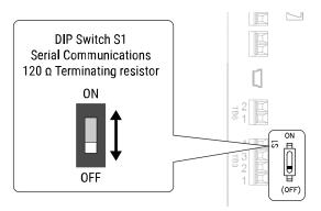
Figure 10.19 Termination Resistor DIP Switch S1
