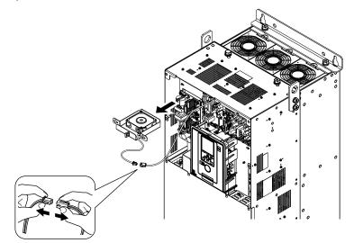
Figure 8.55 Remove the Fan Unit
