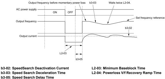
Figure 5.16 Current Detection 2 after a Momentary Power Loss
