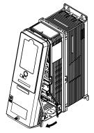
Figure 2.15 Remove the Front Cover
