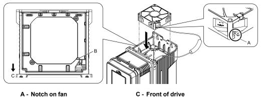
B - Alignment pin on drive
