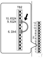
Figure 10.16 Self-Diagnostics Jumper Terminals
