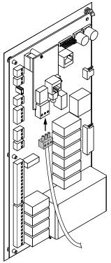
Figure 7.7 Connect Network Cable to Option (SI-W3 LonWorks Example)
