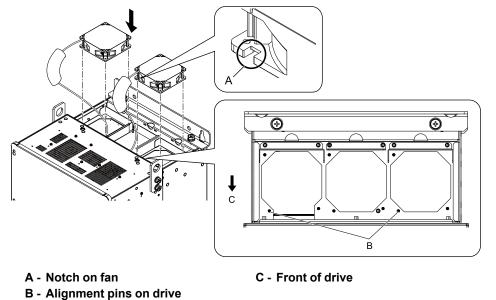
Figure 8.49 Install the Cooling Fans
