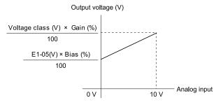
Figure 5.58 Output Voltage Bias through Analog Input
