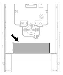
Figure 3.15 Tightening Torque Display Location (Reverse Side of Drive Front Cover)
