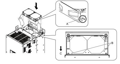
A - Notch on fan B - Alignment pins on drive
