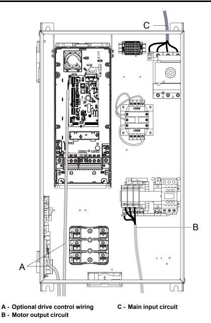
Figure 3.8 Enclosed Bypass Wire Routing Example (Models H6B1D002 to D273, A002 to A248, B1P1, B001 to B302)
