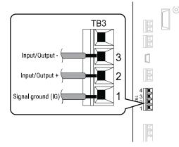
Figure 10.2 Communications Cable Connection Terminal (TB3)
