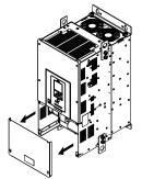
Figure 2.24 Remove the Terminal Cover
