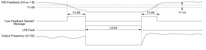
H3-xx = B: PID Feedback L5-04: Interval Method Restart Time Y1-08: Low Feedback Level Y1-09: Low Feedback LvI Fault Dly Time Y1-14: Feedback Hysteresis Level LFB Fault: Low Feedback Sensed
