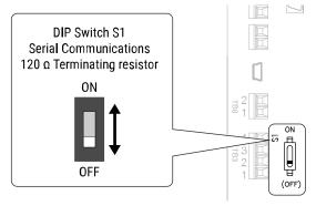
Figure 10.7 Termination Resistor DIP Switch S1
