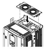
Figure 8.32 Install the Fan Finger Guard
