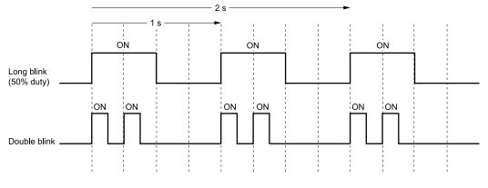
Figure 4.3 AUTO LED and HAND LED Timing Status
