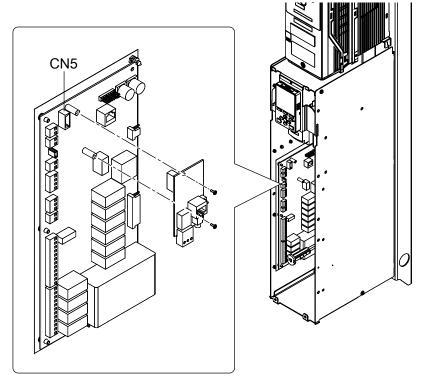
Figure 7.6 Insert Option into Bypass PCB CN5 Connector Port
