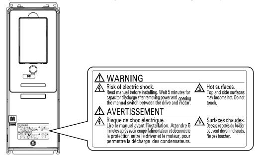
Figure i.1 Drive Warning Label Content and Location
