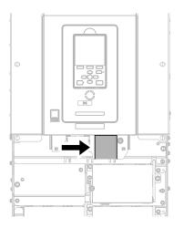
Figure 3.16 Tightening Torque Display Location (Lower Front Side of Drive Front Cover)
