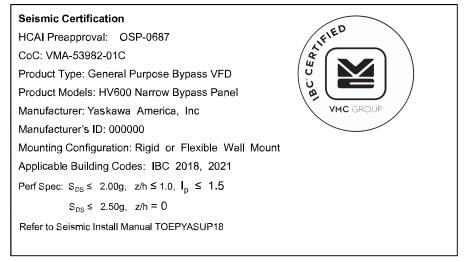
Figure 11.2 Seismic Certification Label Example for Bypasses
