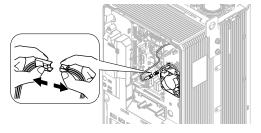
Figure 8.34 Disconnect the Connector
