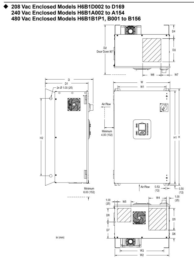
Figure 2.33 Enclosed Exterior and Mounting Dimensions Diagram
