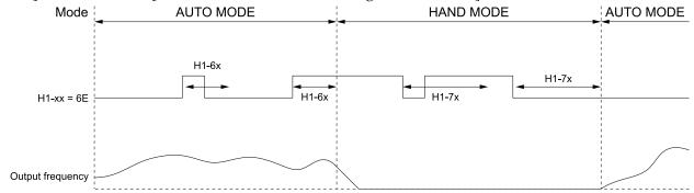
Figure 5.39 Example of ON-Delay and OFF-Delay Timers
