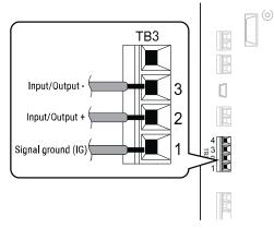
Figure 10.18 Communications Cable Connection Terminal (TB3)
