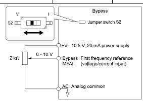
Figure 5.1 Example of Setting the Frequency Reference with a Voltage Signal to the Bypass MFAI
