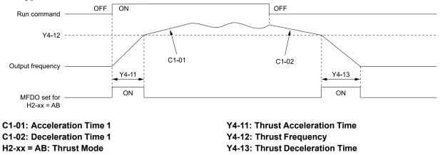
Figure 5.100 Thrust Frequency
