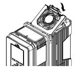
Figure 8.8 Install the Fan Finger Guard
