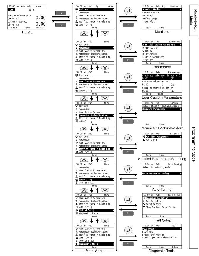
Figure 4.5 Keypad Functions and Display Levels
