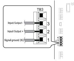
Figure 10.11 Communications Cable Connection Terminal (TB3)
