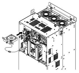
Figure 8.60 Install the Fan Unit
