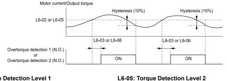
L6-02: Torque Detection Level 1 L6-03: Torque Detection Time 1
