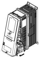
Figure 2.21 Remove the Front Cover
