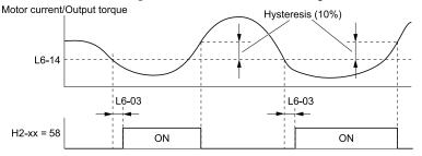
H2-xx = 58: UL6 Underload Detected L6-03: Torque Detection Time 1 L6-14: Motor Underload Level @ Min Freq
