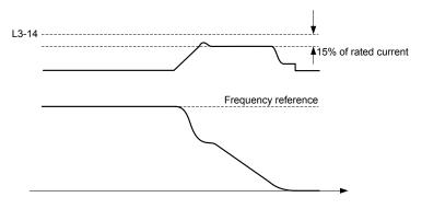
Figure 5.43 Deceleration for Current Limit
