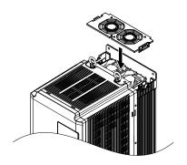
Figure 7.9 Reattach the Fan Guard
