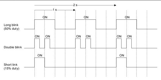
Figure 4.3 AUTO LED and HAND LED Timing Status
