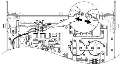
Figure 7.34 Unplug the Relay Connector
