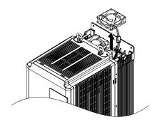
Figure 7.4 Remove the Cooling Fan Cartridge
