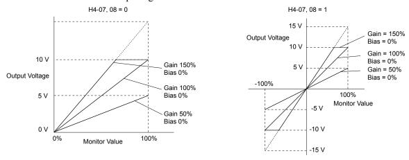
Figure 5.37 Analog Output Gain and Bias Setting Example 1 and 2
