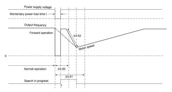
Figure 5.7 Speed Search from Forward Run Command (0 ≤ t < b3-50)
