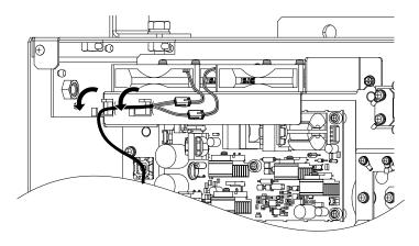
Figure 7.33 Unlock the Cable Hooks
