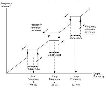
Figure 5.17 Jump Frequency Operation
