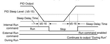
Figure 5.13 PID Sleep Operation
