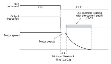
Figure 5.2 DC Injection Braking to Stop
