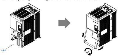
Figure 3.23 Reattaching the Terminal Cover
