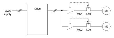
MC1, MC2: Magnetic contactors L10, L20: Thermal relays
