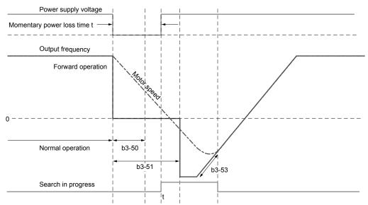
Figure 5.8 Continuous Baseblock (b3-50 ≤ t < b3-51)
