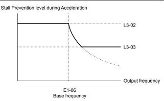
Figure 5.41 Stall Prevention Level and Limit During Acceleration
