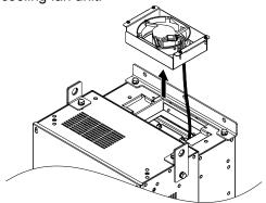
Figure 7.25 Remove the Cooling Fan Unit
