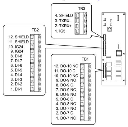
Figure 3.18 Control Circuit Terminal Board A2 Arrangement
