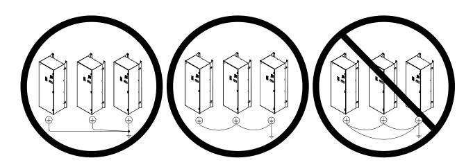
Figure 3.9 Ground Wiring for Multiple Bypass Units
