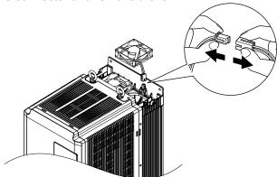
Figure 7.5 Disconnect the Cooling Fan
