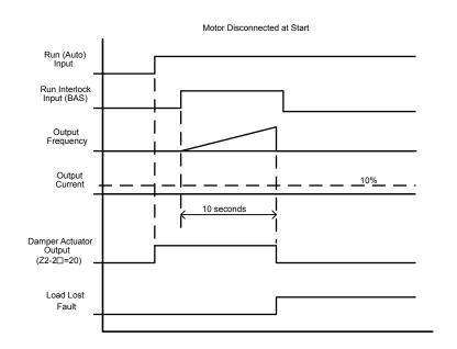
Figure 5.59 Motor Disconnected at Start
