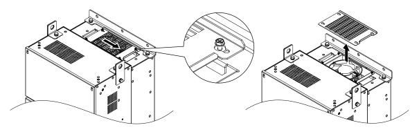
Figure 7.23 Remove the Fan Guard
