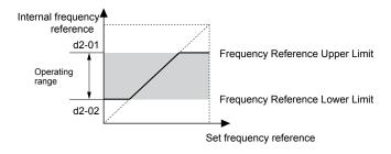
Figure 5.16 Frequency Reference: Upper and Lower Limits
