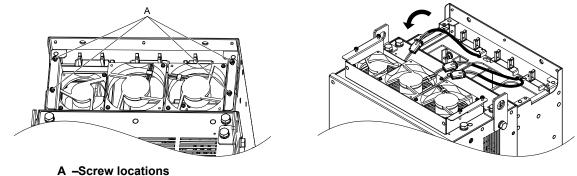
Figure 7.13 Remove the Cooling Fan Unit
