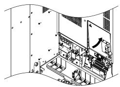
Figure 3.29 Remove the Front Cover (Drive Models 2□0154 to 2□0248 and 4□0156 to 4□0930)
