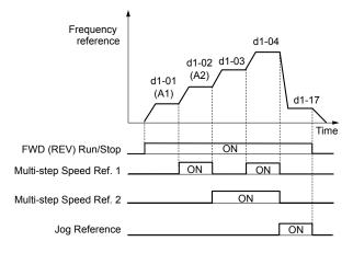
Figure 5.15 Preset Reference Timing Diagram
