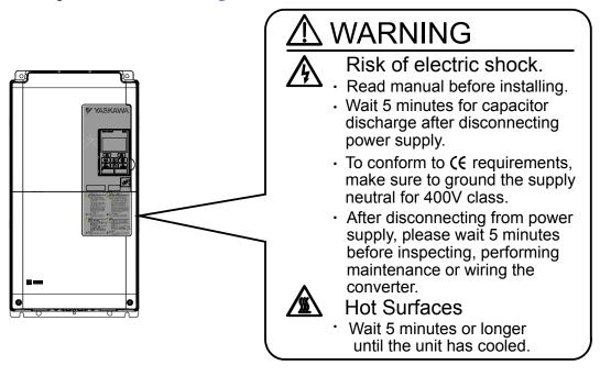
Figure i.1 Warning Information Example and Position
