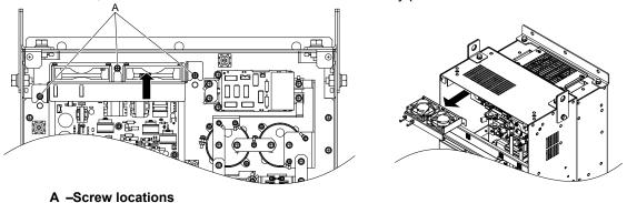
Figure 7.35 Remove the Circulation Fan
