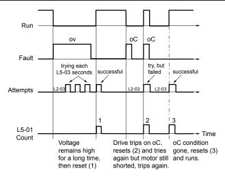
Figure 5.46 Automatic Restart Timing Diagram
