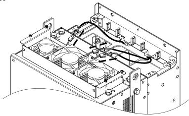
Figure 7.14 Unplug the Relay Connectors
