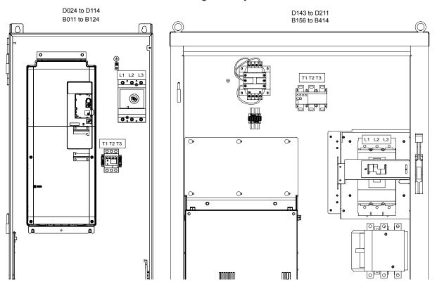
Figure 3.7 Main Circuit Terminal Block Configuration
