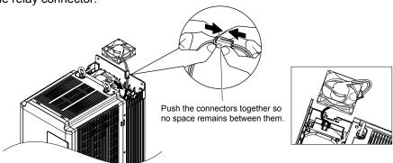
Figure 7.6 Plug the Relay Connector
