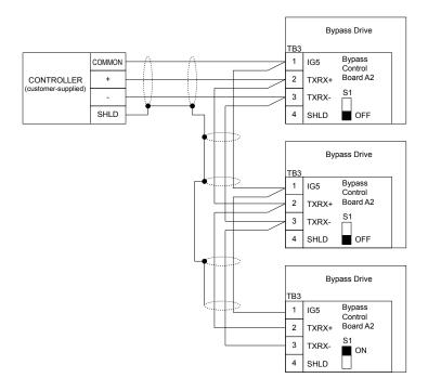
Figure F.3 Connection Diagram for Multiple Connections
