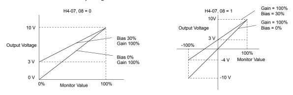
Figure 5.38 Analog Output Gain and Bias Setting Example 3
