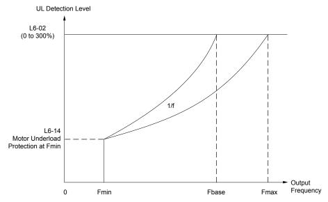
Figure 5.49 Motor Underload Protection
