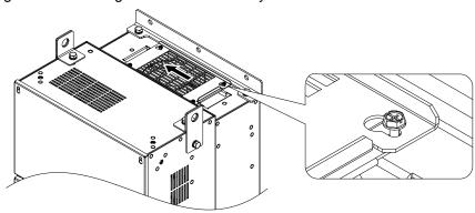
Figure 7.31 Reattach the Fan Cover
