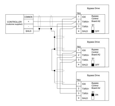
Figure E.2 Connection Diagram for Multiple Connections
