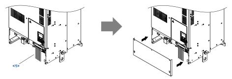
Figure 3.26 Reattaching the Terminal Cover
