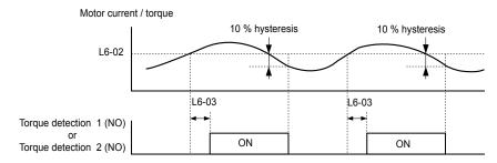
Figure 5.47 Overtorque Detection Operation
