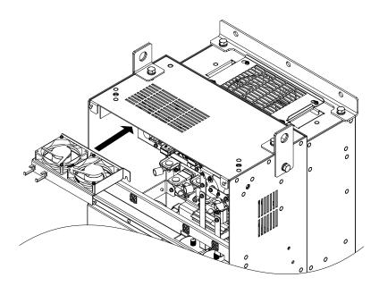
Figure 7.36 Installing the Circulation Fan
