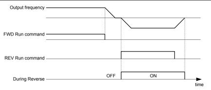
Figure 5.30 Reverse Direction Output Example Time Chart
