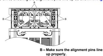
Figure 7.7 Install the Cooling Fan
