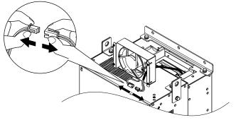
Figure 7.26 Unplug the Relay Connector
