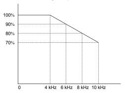
Figure A.1 Carrier Frequency Derating
