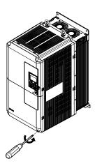
Figure 3.21 Removing the Terminal Cover
