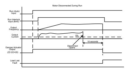
Figure 5.60 Motor Disconnected During Run
