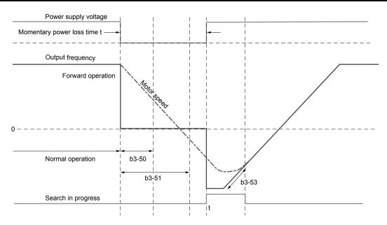
Figure 5.9 Speed Search in Direction Opposite to Direction Command (b3-51 ≤ t)
