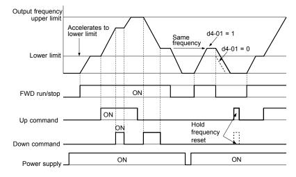
Figure 5.18 Up/Down Command Operation
