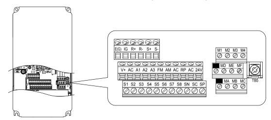
Figure 3.19 Control Circuit Terminal Arrangement
