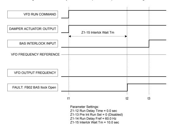
Figure 5.56 Run Delay with Preset Speed Example: BAS Interlock Wait Time Fault
