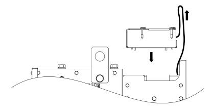
Figure 7.18 Install the Cooling Fan Unit
