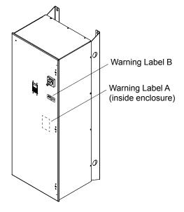
Figure i.4 Bypass Warning Label Locations
