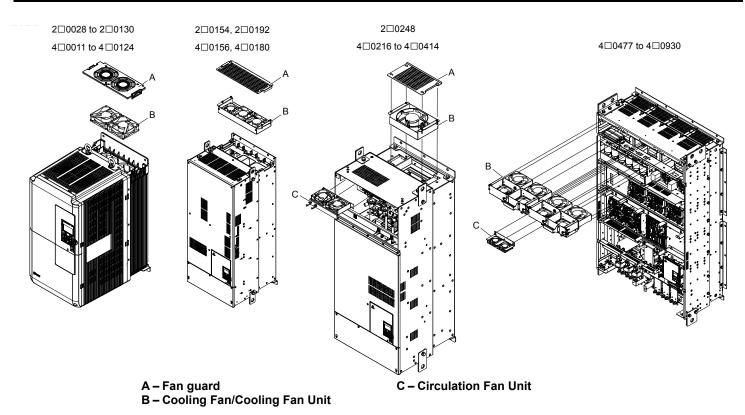
Figure 7.2 Cooling Fan Component Names
