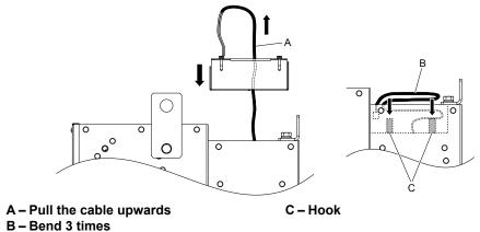
Figure 7.29 Install the Cooling Fan
