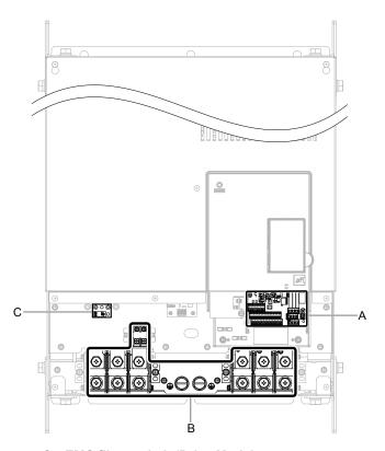
C – EMC filter switch (Drive Models ZUDEDDDD and ZUDWDDD)
