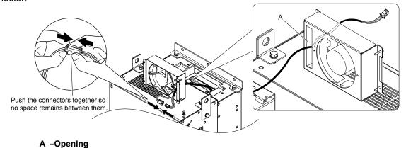
Figure 7.27 Attach the Relay Connector
