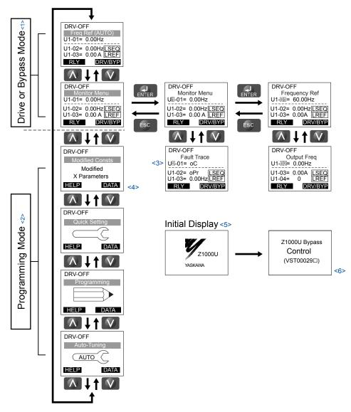
Figure 4.5 HOA Keypad Menu and Screen Structure
