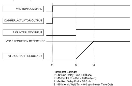
Figure 5.55 Run Delay with Preset Speed Example: Default Setting
