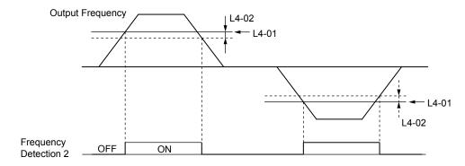
Figure 5.25 Frequency Detection 2 Time Chart
