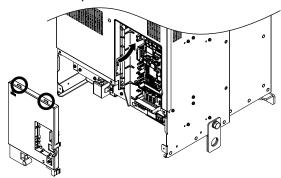
Figure 3.30 Reattach the Front Cover (Drive Models 2□0154 to 2□0248 and 4□0156 to 4□0930)
