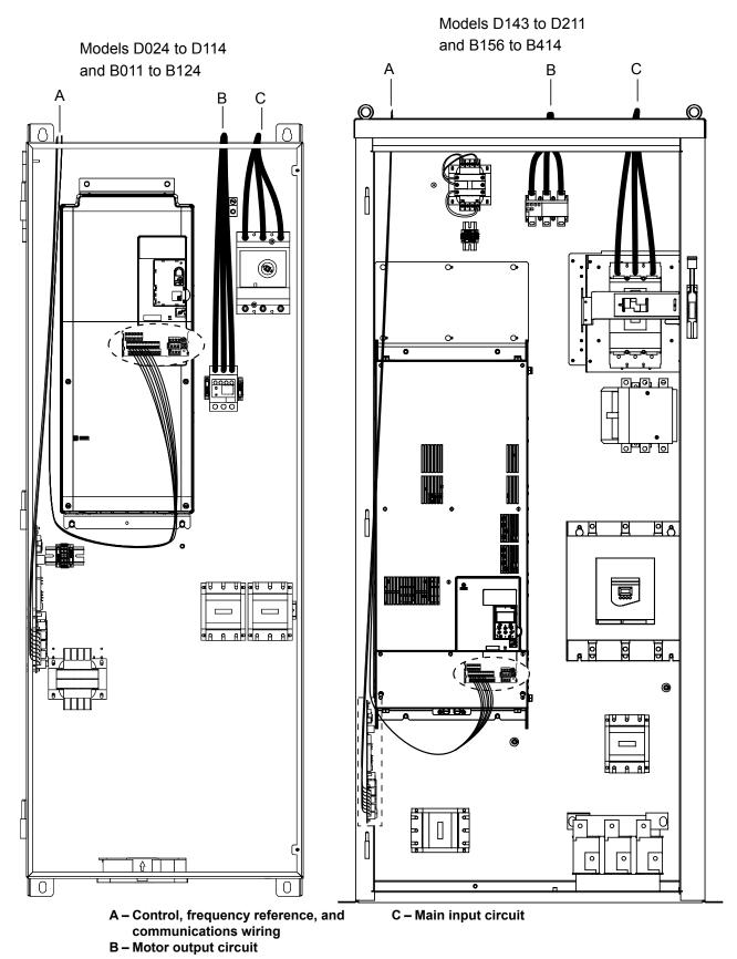
Figure 3.17 Bypass Wire Routing Example
