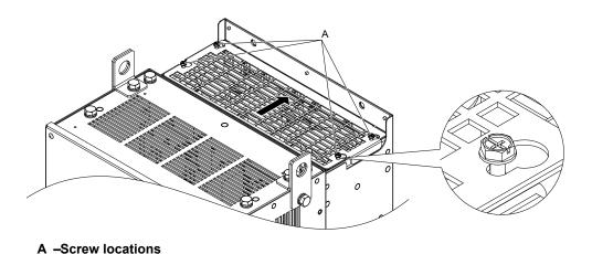
Figure 7.21 Reattach the Fan Guard
