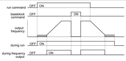
Figure 5.31 During Frequency Output Time Chart
