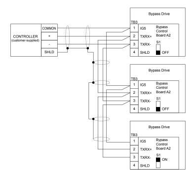
Figure D.3 Connection Diagram for Multiple Connections
