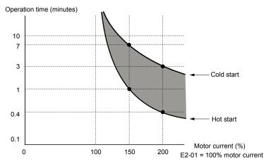
Figure 5.40 Motor Protection Operation Time
