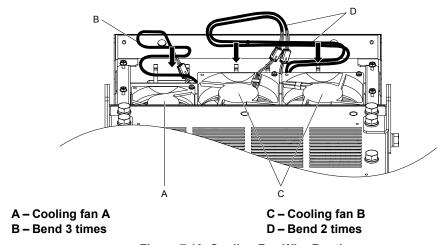
Figure 7.19 Cooling Fan Wire Routing
