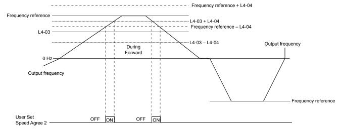
Figure 5.27 User-Set Speed Agree 2 Example with a Positive L3-04 Value
