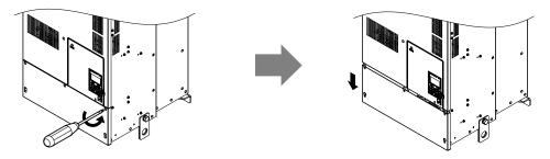
Figure 3.24 Removing the Terminal Cover
