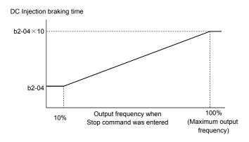
Figure 5.3 DC Injection Braking Time Depending on Output Frequency
