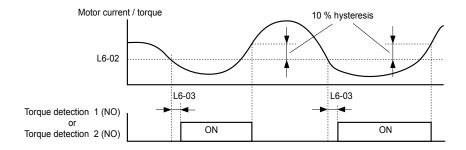
Figure 5.48 Undertorque Detection Operation
