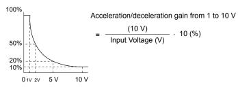
Figure 5.34 Accel/Decel Time Gain with Analog Input Terminal
