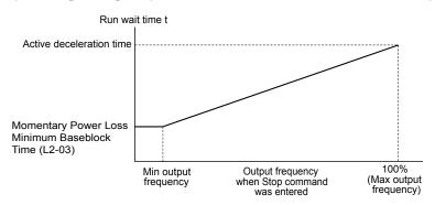
Figure 5.5 Run Wait Time Depending on Output Frequency
