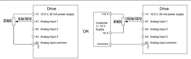
Figure 5.53 Setting the Frequency Reference as a Voltage Signal at Terminal A1
