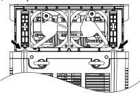
Figure 7.8 Relay Connector Placement
