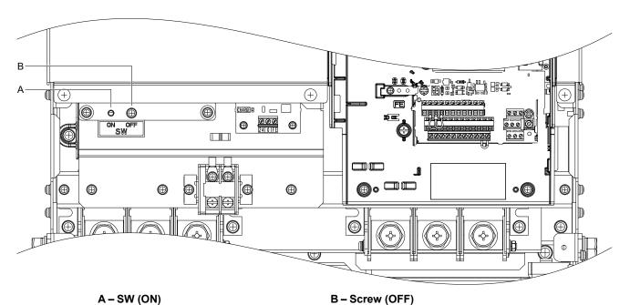
Figure 3.14 EMC Filter Switch Location (Models 2E0154, 2W0154, 2E0192, 2W0192, 4E0156, 4W0156, 4E0180, and 4W0180)
