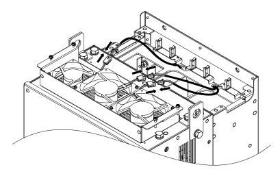
Figure 7.15 Plug the Relay Connectors
