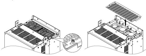
Figure 7.11 Remove the Fan Guard
