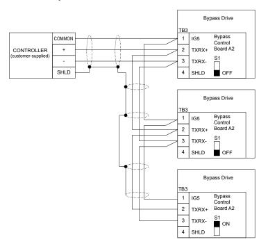
Figure C.3 Connection Diagram for Multiple Connections
