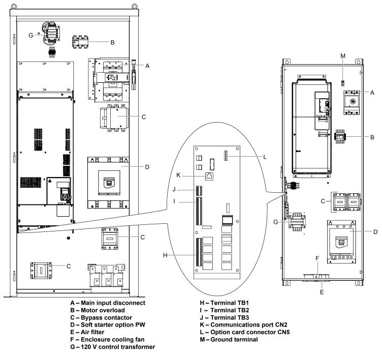
Figure 1.6 Interior View of Bypass Unit
