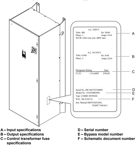
Figure 1.3 Bypass Nameplate Information Example
