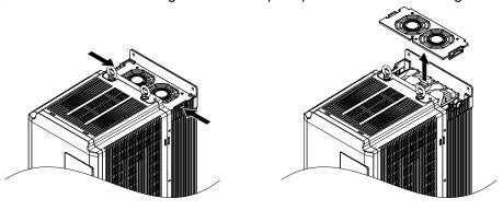
Figure 7.3 Remove the Fan Guard
