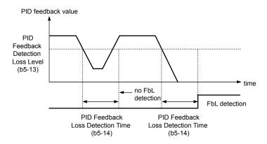
Figure 5.12 PID Feedback Loss Detection
