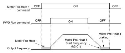
Figure 5.19 Motor Pre-Heat 1 Input Timing Diagram
