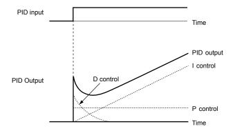
Figure 5.10 PID Operation
