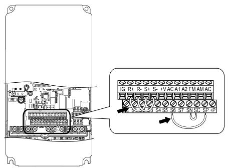
Figure B.7 Terminal Connections for Communication Self-Diagnostics
