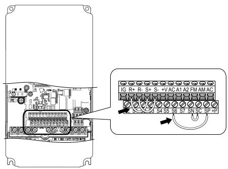
Figure E.8 Terminal Connections for Communication Self-Diagnostics
