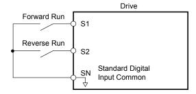
Figure 1.37 Example Wiring Diagram for 2-Wire Sequence
