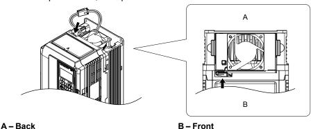
Figure 2.7 Connect the Cooling Fan Power Supply Connectors: 5A0006 to 5A0032
