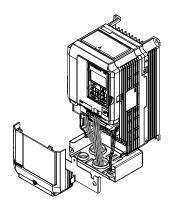
Figure 2.23 Remove the Terminal Cover
