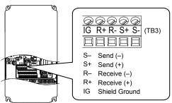
Figure B.2 Serial Communications Cable Connection Terminal (TB3)
