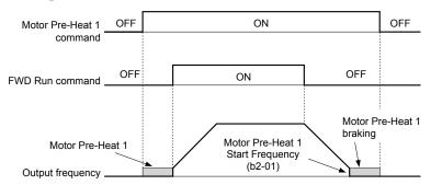
Figure 1.38 Motor Pre-Heat 1 Input Timing Diagram
