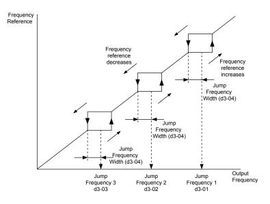
Figure 1.26 Jump Frequency Operation
