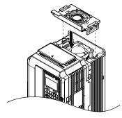
Figure 2.8 Reattach the Fan Finger Guard: 5A0006 to 5A0032
