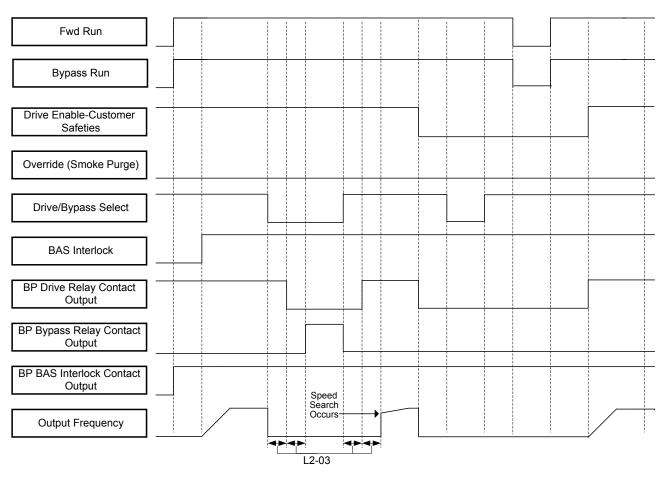
Figure 1.77 Transfer to Bypass and Safety Circuit
