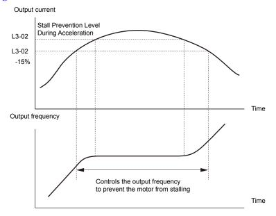
Figure 1.61 Stall Prevention During Acceleration for Induction Motors
