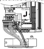
Figure 2.25 Remove the Terminal Board
