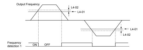
Figure 1.43 Frequency Detection 1 Time Chart
