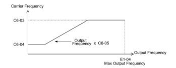
Figure 1.22 Carrier Frequency Changes Relative to Output Frequency
