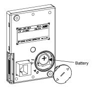
Figure 2.2 Install the Battery
