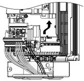
Figure 2.27 Install the Terminal Board
