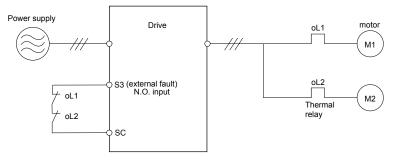
Figure 1.57 Example of Protection Circuit Design for Multiple Motors
