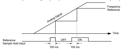
Figure 1.36 Analog Frequency Reference Sample/Hold
