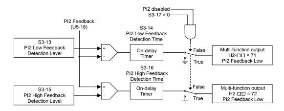
Figure 1.76 PI Low Feedback Detection Level
