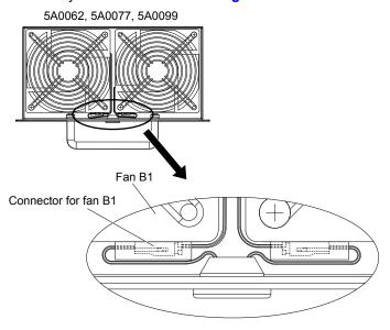
Figure 2.18 Cooling Fan Wiring: 5A0062 to 5A0099
