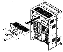
Figure 2.16 Remove the Fan Unit: 5A0062 to 5A0242
