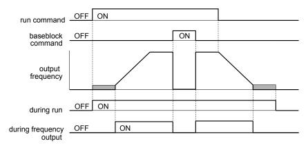
Figure 1.49 During Frequency Output Time Chart
