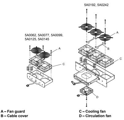
Figure 2.17 Fan Unit Disassembly: 5A0062 to 5A0242
