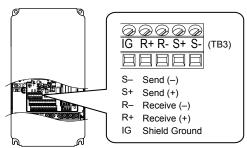
Figure D.2 Serial Communications Cable Connection Terminal (TB3)
