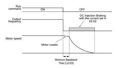
Figure 1.4 DC Injection Braking to Stop
