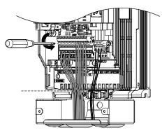
Figure 2.24 Unscrew the Terminal Board and Remove the Bottom Cover
