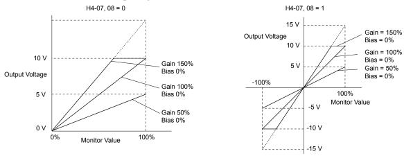
Figure 1.55 Analog Output Gain and Bias Setting Example 1 and 2
