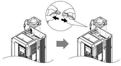
Figure 2.5 Remove the Cooling Fan: 5A0006 to 5A0032
