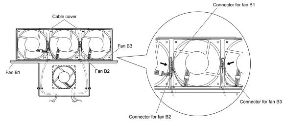
Figure 2.20 Cooling Fan Wiring: 5A0192 and 5A0242
