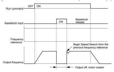
Figure 1.32 Baseblock Operation During Run
