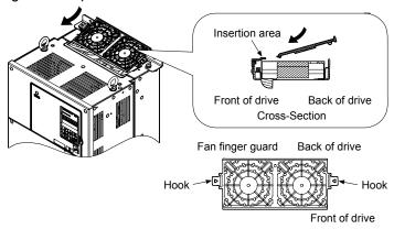
Figure 2.13 Reattach the Fan Cover: 5A0041 and 5A0052
