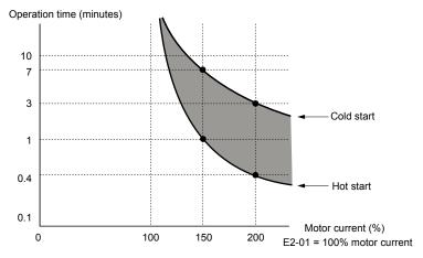
Figure 1.58 Motor Protection Operation Time
