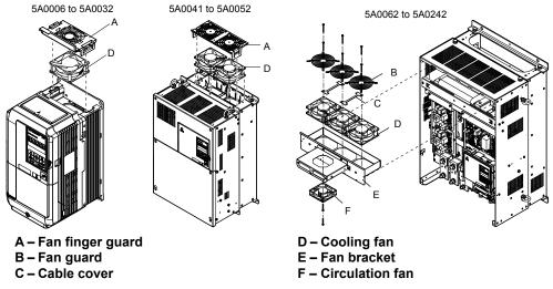
Figure 2.3 Cooling Fan Components
