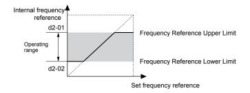
Figure 1.25 Frequency Reference: Upper and Lower Limits
