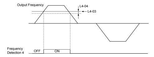
Figure 1.48 Frequency Detection 4 Example with Positive L3-04 Value
