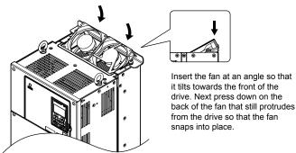
Figure 2.12 Install the Cooling Fan: 5A0041 and 5A0052
