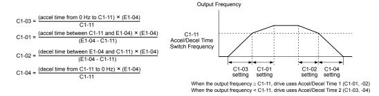
Figure 1.20 Accel/Decel Time Switching Frequency
