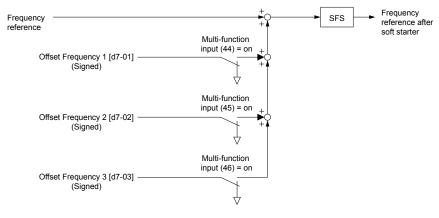
Figure 1.28 Offset Frequency Operation
