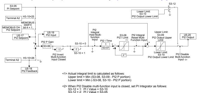
Figure 1.75 Pl2 Block Diagram
