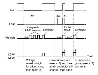
Figure 1.67 Automatic Restart Timing Diagram
