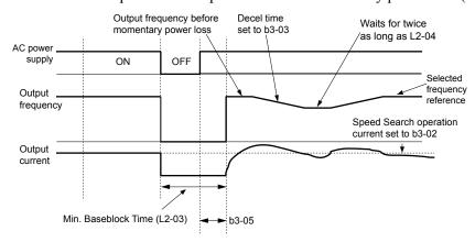
Figure 1.10 Current Detection Speed Search after Power Loss
