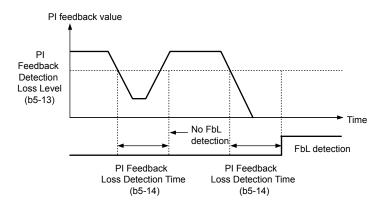
Figure 1.17 PI Feedback Loss Detection
