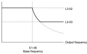
Figure 1.63 Stall Prevention Level and Limit During Acceleration
