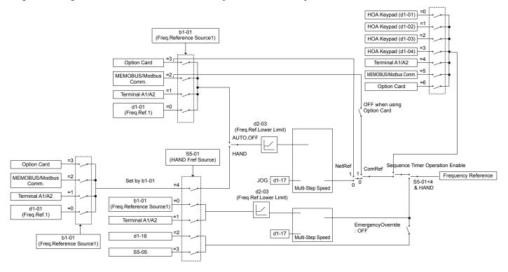
Figure 1.23 Frequency Reference Setting Hierarchy
