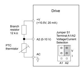
Figure 1.59 Connection of a Motor PTC
