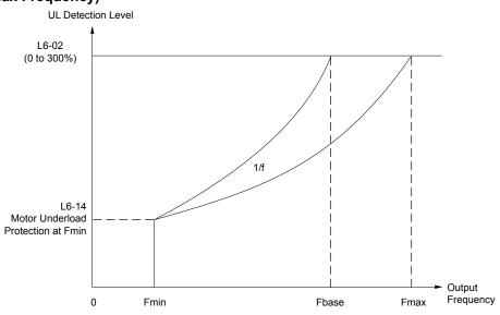
Figure 1.70 Motor Underload Protection
