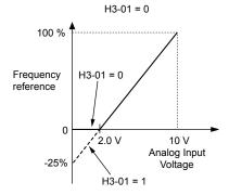
Figure 1.51 Frequency Reference Setting by Analog Input with Negative Bias
