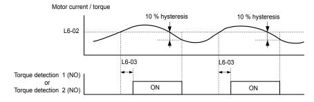
Figure 1.68 Overtorque Detection Operation
