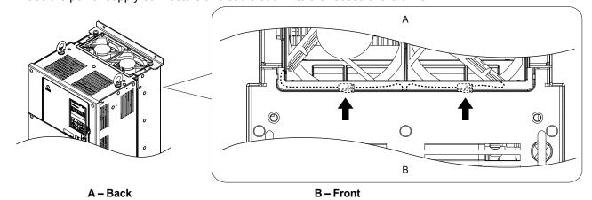
Figure 2.11 Cooling Fan Power Supply Connectors: 5A0041 and 5A0052
