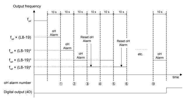
Figure 1.71 Output Frequency Reduction During Overheat Alarm
