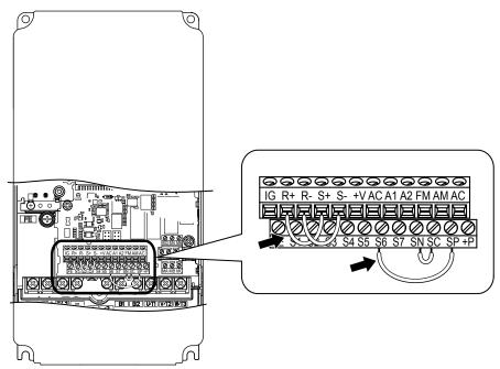
Figure D.7 Terminal Connections for Communication Self-Diagnostics
