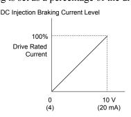
Figure 1.53 DC Injection Braking Current Using an Analog Input Terminal
