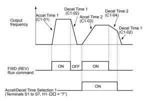
Figure 1.19 Timing Diagram of Accel/Decel Time Change
