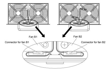
Figure 2.19 Cooling Fan Wiring: 5A0125 and 5A0145
