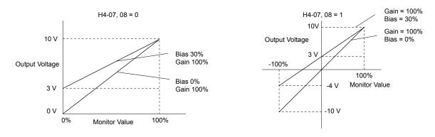
Figure 1.56 Analog Output Gain and Bias Setting Example 3
