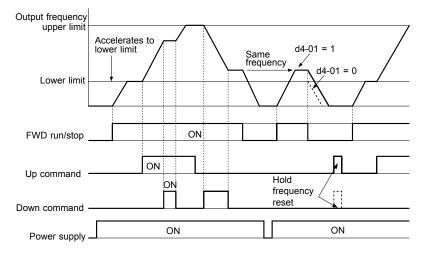
Figure 1.33 Up/Down Command Operation
