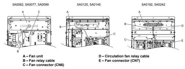
Figure 2.15 Cooling Fan Replacement: Fan Unit and Connectors
