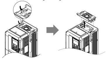
Figure 2.4 Remove the Cooling Fan Finger Guard: 5A0006 to 5A0032
