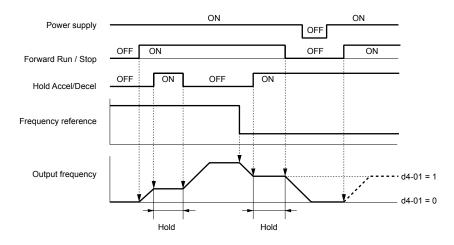
Figure 1.27 Frequency Reference Hold with Accel/Decel Hold Function
