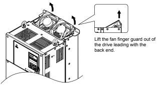
Figure 2.10 Remove the Cooling Fan: 5A0041 and 5A0052
