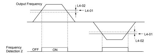
Figure 1.44 Frequency Detection 2 Time Chart
