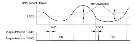
Figure 1.69 Undertorque Detection Operation
