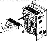
Figure 2.21 Install the Cooling Fan Unit: 5A0062 to 5A0242
