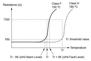
Figure 1.60 Motor PTC Characteristics
