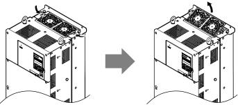
Figure 2.9 Remove the Cooling Fan Finger Guard: 5A0041 and 5A0052
