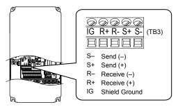
Figure E.2 Serial Communications Cable Connection Terminal (TB3)
