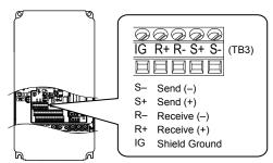
Figure C.1 Serial Communications Cable Connection Terminal (TB3)
