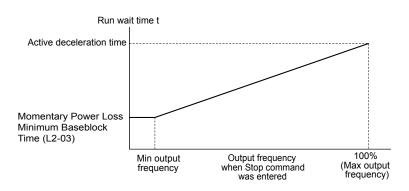
Figure 1.7 Run Wait Time Depending on Output Frequency
