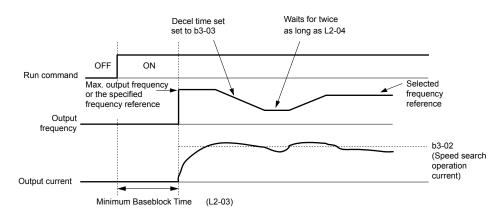
Figure 1.11 Current Detection Speed Search at Start or Speed Search Command by Digital Input
