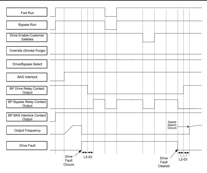
Figure 1.80 Transfer on Fault
