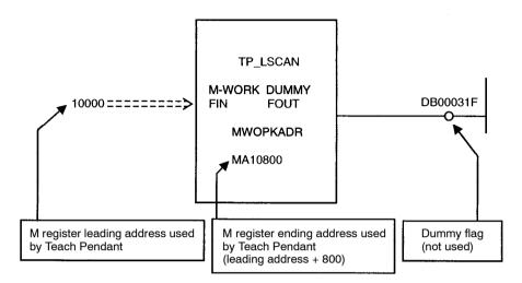
Figure 1.4 TP\_LSCAN Setting Example
