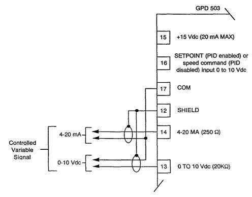
Figure 4. Transducer Wiring For PID Function
