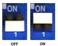
Figure 1.5 – Termination Switch
