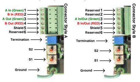
Figure D.1 - PROFIBUS-DP Option Connections
