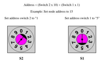
Figure 1.4 - Setting the PROFIBUS-DP Option Node Address
