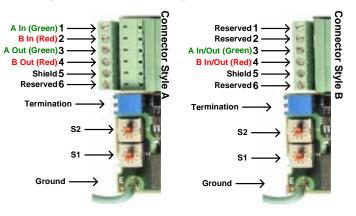
Figure 1.3 – PROFIBUS-DP Option Connections
