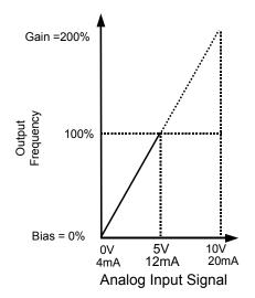
Fig 5.25 Output Frequency as Commanded via Analog Input with Increased Gain Setting
