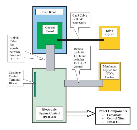
Fig 2.11 E7N Electronic Control Interconnection of Components
