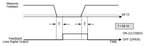
Fig 5.17 Loss of PI Feedback Feature
