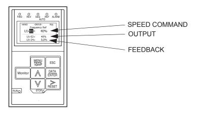
Fig 5.15 Drive Display for PI Control, HAND Mode
