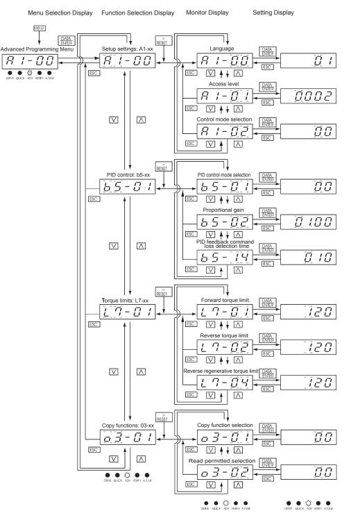
Fig 3.6 Operations in Advanced Programming Menu
