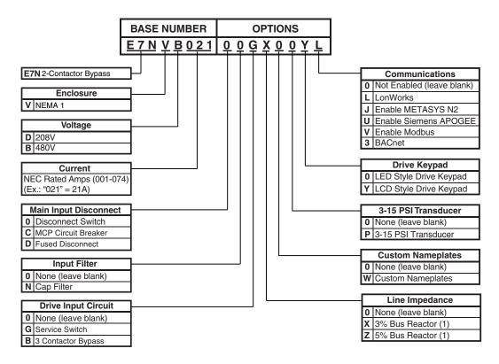
Fig 1.3 Bypass Unit Model Number
