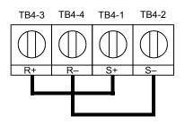
Fig D.3 RS-485 Communication Connection
