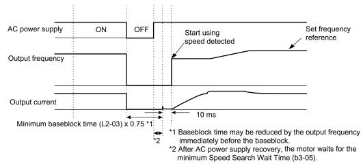
Fig 5.8 Speed Search (Estimated Speed Method) after momentary power loss where the power loss time is less than the minimum baseblock time
