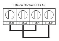
Fig 2.8 RS-485 Communication Connection
