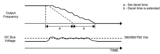
Fig 5.32 Time Chart for Stall Prevention During Deceleration
