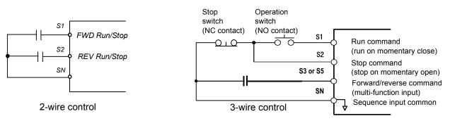
Fig 5.1 2 & 3-Wire Control Wiring Examples
