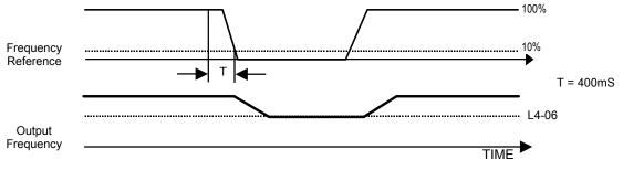
Fig 5.34 Loss of Frequency Reference Timing Diagram
