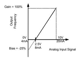
Fig 5.26 Output Frequency with Reduced Bias Setting
