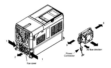
Fig 7.4 Cooling Fan Replacement Procedure
