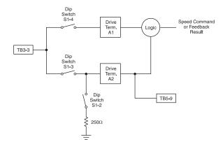
Fig 2.5 Analog Input PCB A2 Configuration
