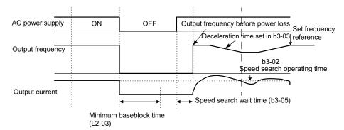
Fig 5.12 Speed Search (Current Detection Method) after momentary power loss where the power loss time exceeds the minimum baseblock time
