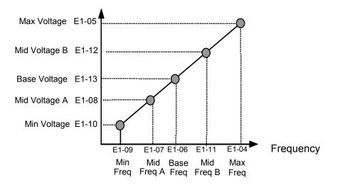
Fig 5.23 Custom V/f Pattern Programming Curve
