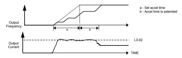
Fig 5.31 Time Chart for Stall Prevention During Acceleration
