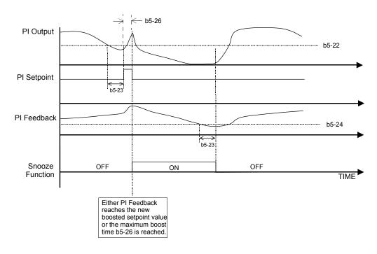
Fig 5.19 Snooze Function Operation
