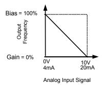
Fig 5.27 Output Frequency with Inverted Gain and Bias Settings
