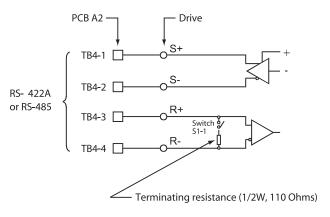
Fig 2.7 Terminating Resistor
