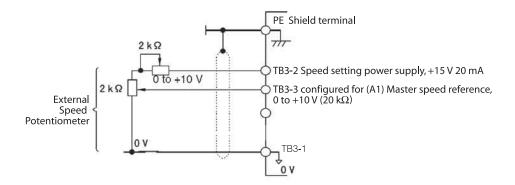
Fig 2.6 Analog Input Terminal Configuration
