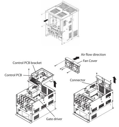
Fig 7.5 Cooling Fan Assembly Replacement Procedure
