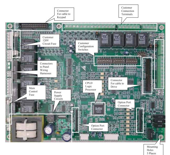
Fig 6.1 Electronic Bypass Control Board Layout
