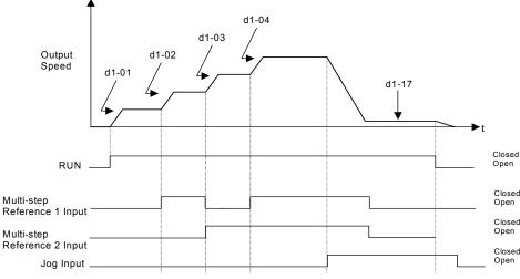
Fig 5.20 Preset Reference Timing Diagram example
