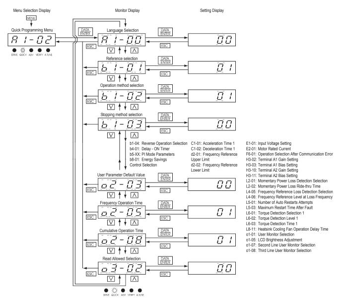
Fig 3.5 Operations in Quick Programming Menu
