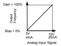
Fig 5.24 Output Frequency as Commanded Via Analog Input
