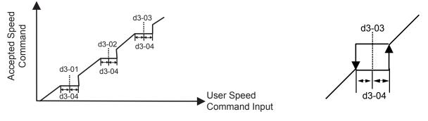
Fig 5.22 Jump Frequency Characteristics
