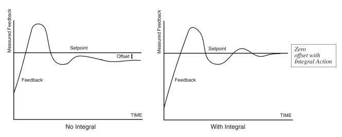
Fig 5.16 PID Feedback Response Characteristics
