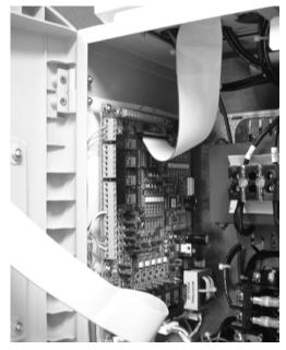
Fig 2.4 TB1 Control Terminal Locations, All Models
