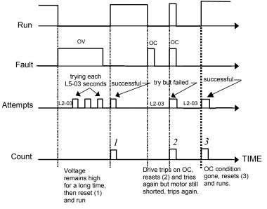
Fig 5.35 Automatic Restart Timing Diagram
