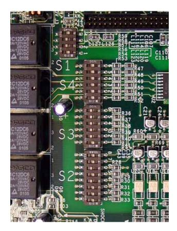
DIP Switches are "ON" when moved toward the enclosure door.
