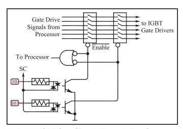
Safe-Off Circuitry Blocks the IGBT Gate Signals Through Two Separate Hardware Channels
