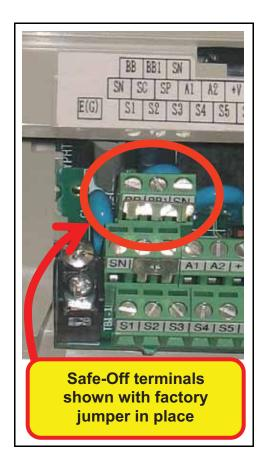
The time from opening either Safe-Off input until the drive output is switched off is less than 10 milliseconds.
