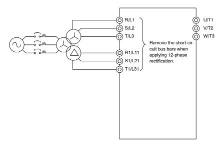
Fig 3.6 Wiring when Applying 12-phase Rectification
