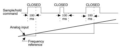
Fig 7.34 Analog Frequency Reference Sample/Hold
