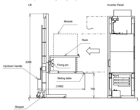
1. Adjust the rack height using the up/down handle of the Module draw-out lift.
