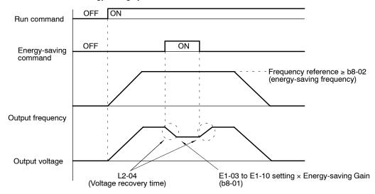
Fig 7.17 Time Chart for Energy-saving Operation
