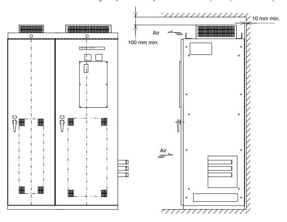
Fig 2.9 Installation Orientation and Space for VS-616G5 Inverters
