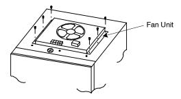
Fig 10.3 Removal of In-panel Ventilation Fan Unit
