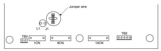
Fig 7.10 Jumper Wire Mounting Location on Control Board
