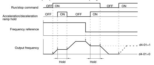
Fig 7.31 Acceleration/Deceleration Ramp Hold
