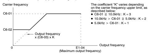
Fig 7.26 Setting the Carrier Frequency
