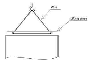
Fig 2.3 Bad Lifting Example
