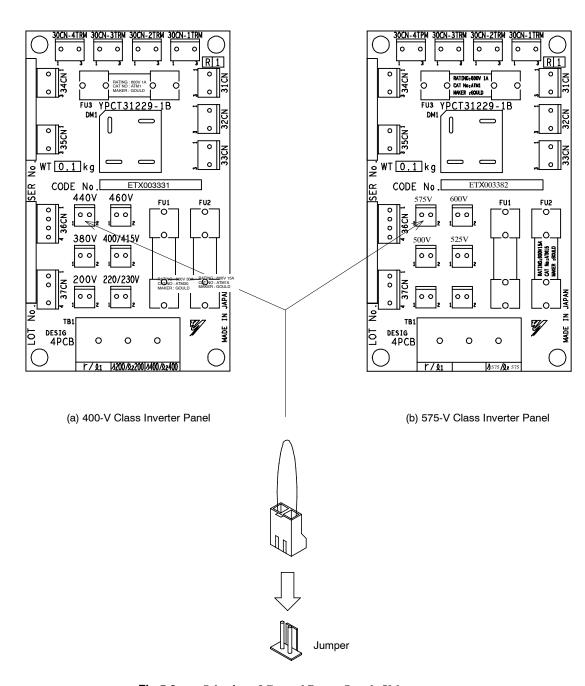
Fig 5.3 Selection of Control Power Supply Voltage
