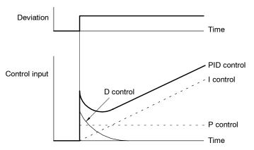
Fig 7.21 PID Control Operations
