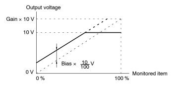
Fig 7.41 Monitor Output Adjustments
