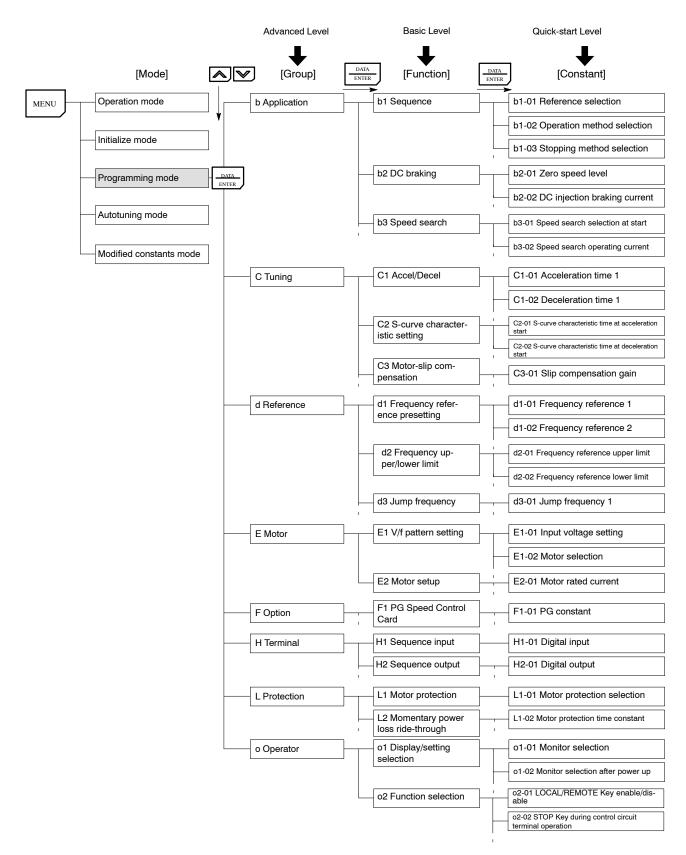
Fig 4.11 Display Structures for Different Access Levels
