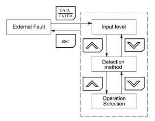
Fig 7.35 Setting Procedure for External Fault Function
