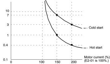
Fig 7.42 Motor Protection Operating Time
