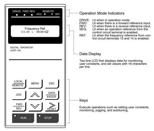
Fig 1.3 Digital Operator Component Names and Functions
