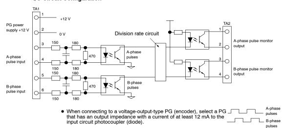
Fig 3.13 I/O Circuit Configuration of the PG-B2
