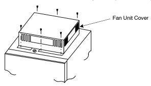
Fig 10.2 In-panel Ventilation Fan Mounted on Ceiling
