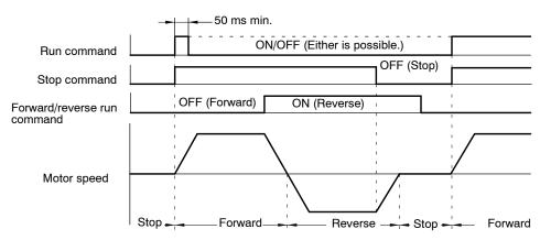
Fig 6.9 Timing Chart for 3-wire Sequence
