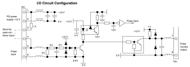
Fig 3.11 I/O Circuit Configuration of the PG-A2
