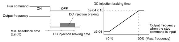
After the stop command is input and the minimum baseblock time (L2-03) has elapsed, DC injection braking is applied and the motor stopped.
