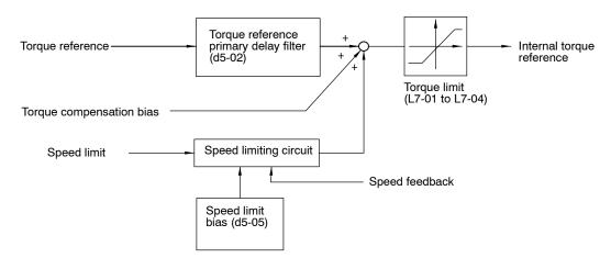
Fig 7.9 Torque Control Block Diagram
