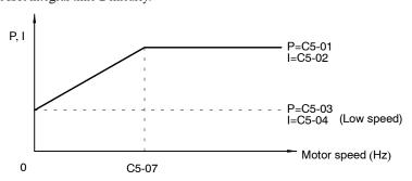
If C5-07 is set to 0.0, ASR proportional gain 1 and ASR integral time 1 are used for the proportional gain and integral time at all frequencies.
