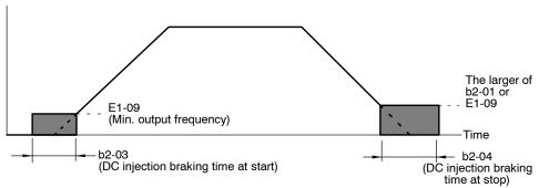
Fig 7.18 DC Injection Braking Timing Chart
