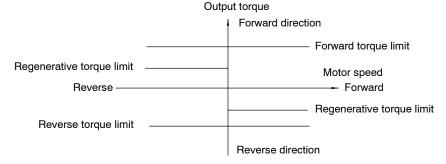
Fig 7.2 Limiting Torque with Analog Inputs
