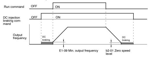
Fig 7.37 Timing Chart for DC Injection Braking Command
