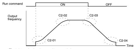
Fig 7.24 Setting S-curve Characteristics
