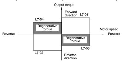
Fig 7.14 Torque Limit Function
