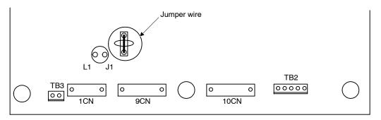
Fig 6.1 Jumper Wire Location on Control Board
