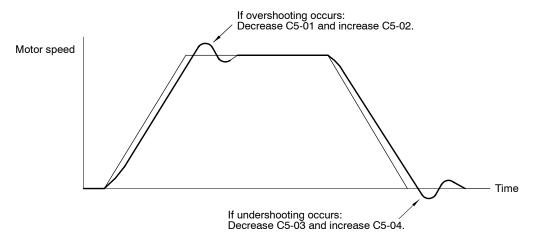
Fig 6.24 Gain Adjustments
