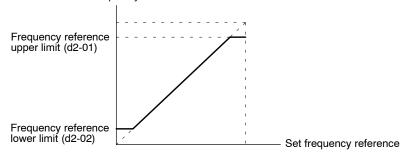
Fig 7.27 Upper and Lower Limits of the Frequency Reference
