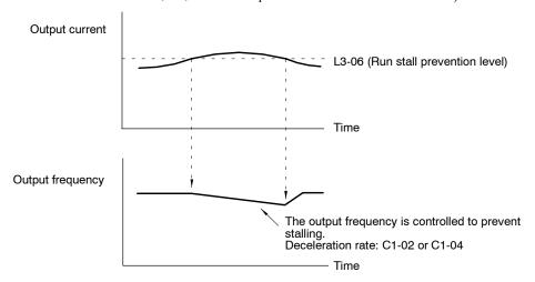
Fig 7.46 Run Stall Prevention Function: L3-05 = 1 or 2
