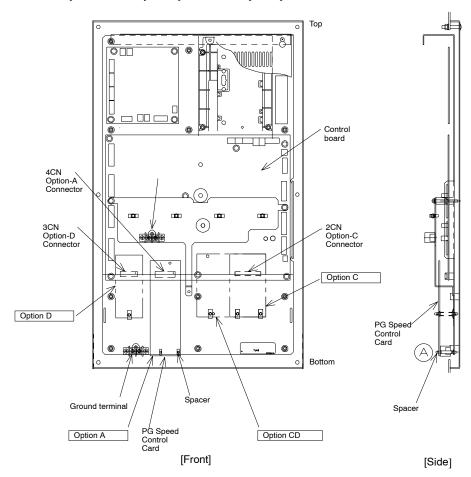
Fig 3.8 Installing a PG Speed Control Card
