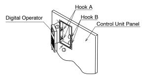
Fig 2.11 Mounting the Digital Operator
