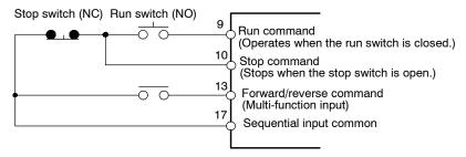
Fig 6.8 3-wire Sequence Wiring Example
