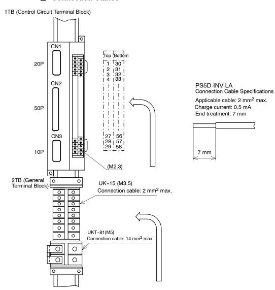
Fig 3.2 Connection Cables
