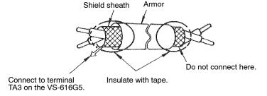
Fig 3.18 Processing the Ends of Twisted-pair Cables
