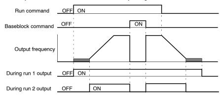
Fig 7.39 Timing Chart for "During RUN" Output
