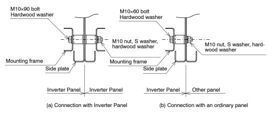
Fig 2.6 Side-by-side Connection Joint
