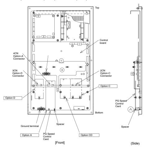
Fig 7.29 Installing a PG Speed Control Card
