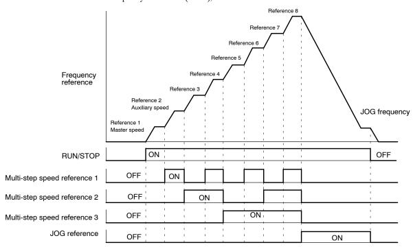
Fig 6.10 Timing Chart for Multi-step Speed and JOG References
