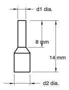
Fig 3.16 Straight Solderless Terminal Sizes
