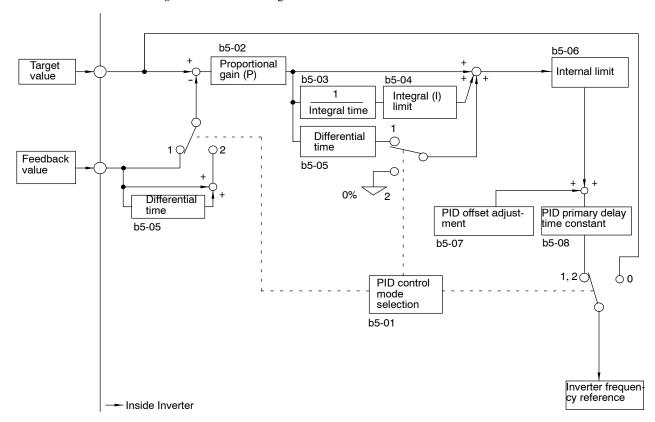
Fig 7.22 Block Diagram for PID Control in Inverter
