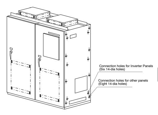
Fig 2.5 Inverter Panel Side-by-side Connection
