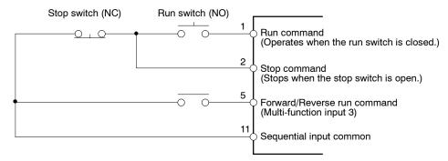
Fig 4.9 Example of Wiring for 3-wire Sequential Operation
