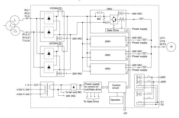
Fig 3.4 Main Circuit Configuration (CIMR-G5A4800)
