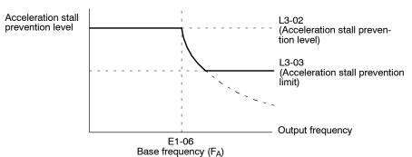
Note When the motor is used in the high-speed range, the acceleration stall prevention level is automatically lowered to provide smoother acceleration.
