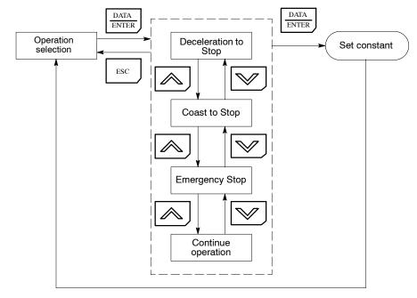
**Fig 7.36** Procedure to Change Constant Settings
