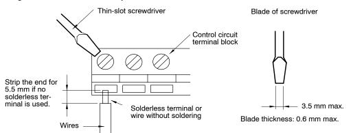
Fig 3.17 Connecting Wires to Terminal Block
