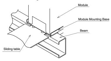
Fig 10.15 Sliding Table Insertion
