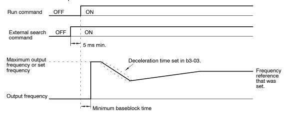
Fig 7.38 Timing Chart for the External Search Command
