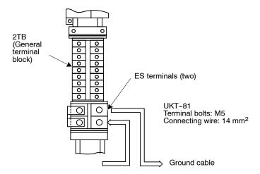
Fig 3.22 Connection of Ground Cable for Control Signals
