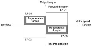
Fig 7.1 Torque Limit Function
