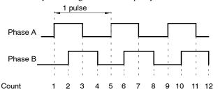
Factor of 4: By counting the rising and falling edges of phase A this method has four times the resolution of the PG.
