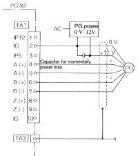
Fig 3.20 PG-X2 Connection Example
