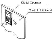
Fig 2.10 Removing the Digital Operator
