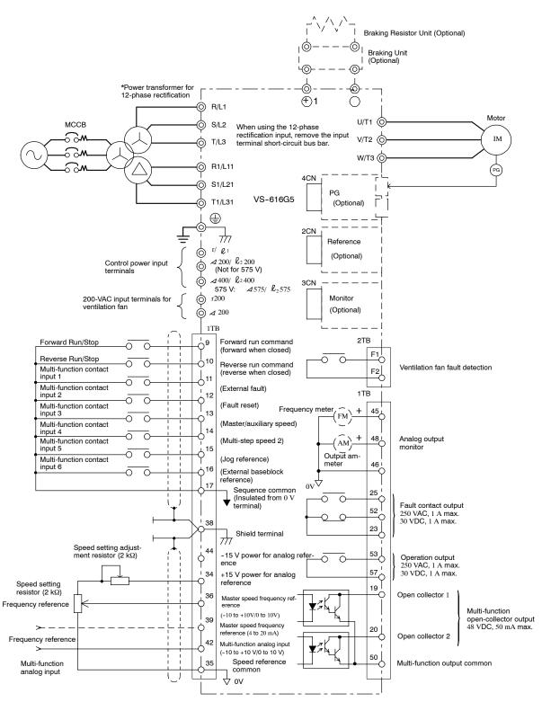
Note (1) Double circles indicate main circuit terminals and single circles indicate control circuit terminals.
