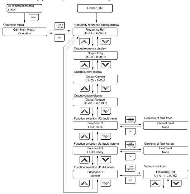
Fig 4.6 Operations in Operation Mode
