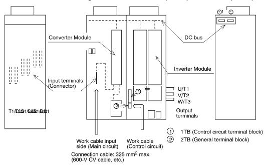
**Note** The main circuit terminals on the output side are provided as bus bar terminals on the side surface. Connections are normally made to the output terminal block on the right side.
