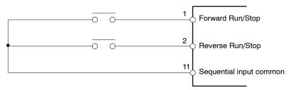
Fig 4.8 Example of Wiring for 2-wire Sequential Operation
