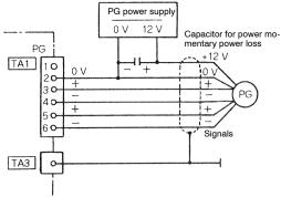
Fig 3.19 PG-B2 Connection Example
