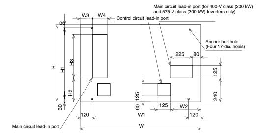
Fig 2.7 Tightening Anchor Bolts
