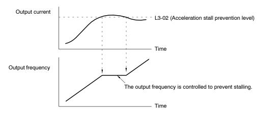
Fig 7.43 **Acceleration Stall Prevention Function: L3-01 = 1**
