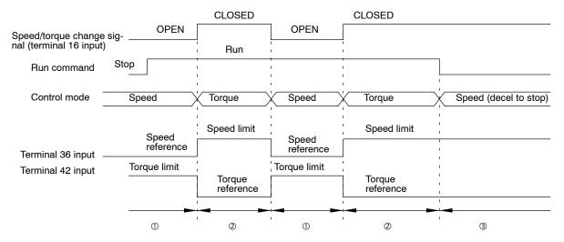
Fig 7.13 Switching between Speed and Torque Control
