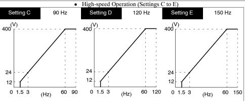
The voltages above are for 400-V Class Inverters. Multiply the voltages by approx. 1.5 for 575-V Class Inverters.
