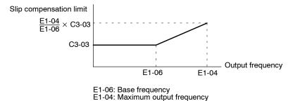
Fig 7.25 **Slip Compensation Limit**
