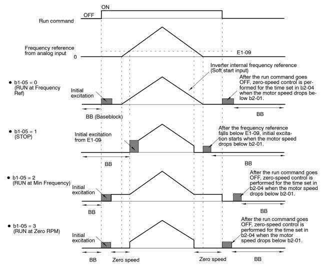
Fig 6.13 Settings for Initial Excitation and Zero-speed Control
