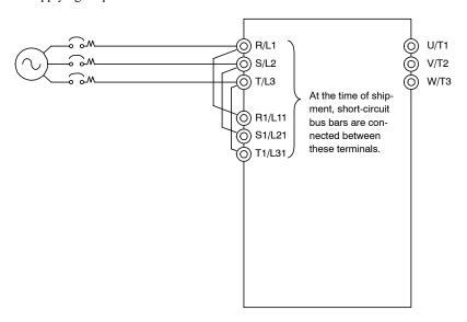
Fig 3.5 Short-circuit Bus Bar Connections
