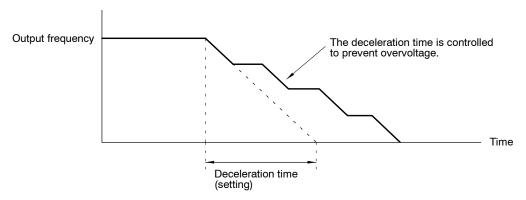
Fig 7.45 Deceleration Stall Prevention Function: L3-04 = 1
