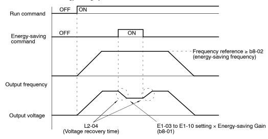
Fig 7.4 Time Chart for Energy-saving Operation
