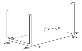
Fig 2.4 Lifting Bar Insertion Locations
