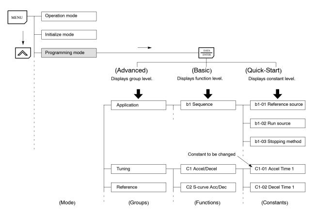
Fig 1.1 Access Level Structure
