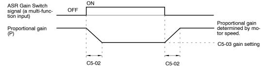
The gain is changed linearly in integral time 1 (C5-02). The integral time setting isn't switched.
