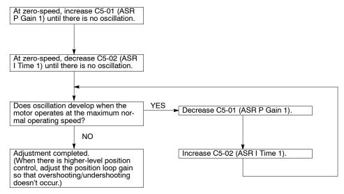
Fig 6.17 Gain Adjustment Procedure
