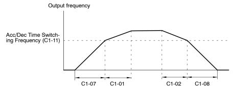
Acceleration/Deceleration Times 1 (C1-01 and C1-02) are used when the output frequency  $\geq$  C1-11 Acceleration/Deceleration Times 4 (C1-07 and C1-08) are used when the output frequency < C1-11
