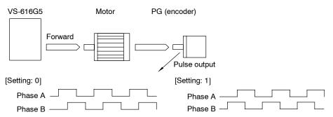
Forward rotation in a typical motor (applicable Yaskawa PG: made by Thermtac):
