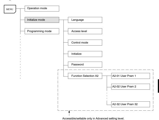
Fig 4.7 Structure of Initialize Mode User Constants
