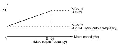
Fig 6.22 Minimum Output Frequency Gain Settings
