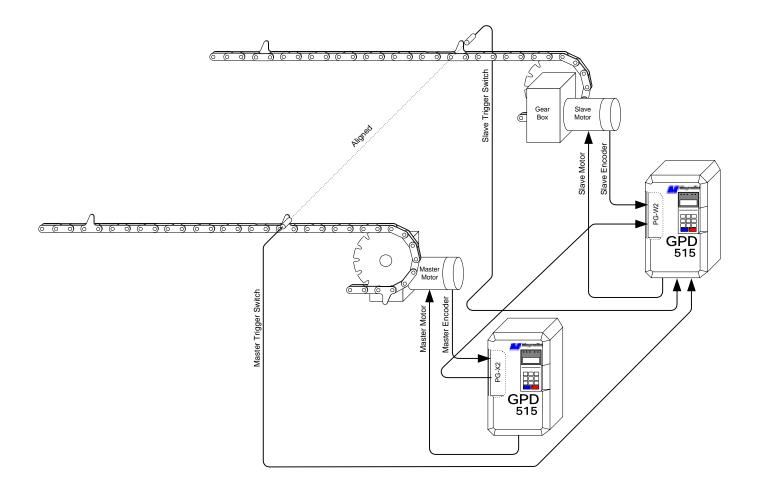
This example shows two pusher chains. Each chain is mechanically isolated from the other. The master and slave trigger switches are placed in line providing an alignment position for the pushers. The pusher's leading edge will activate the switches as they pass.
