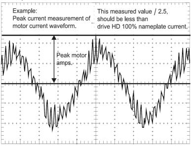
Figure 5.1 Measuring Peak Current
