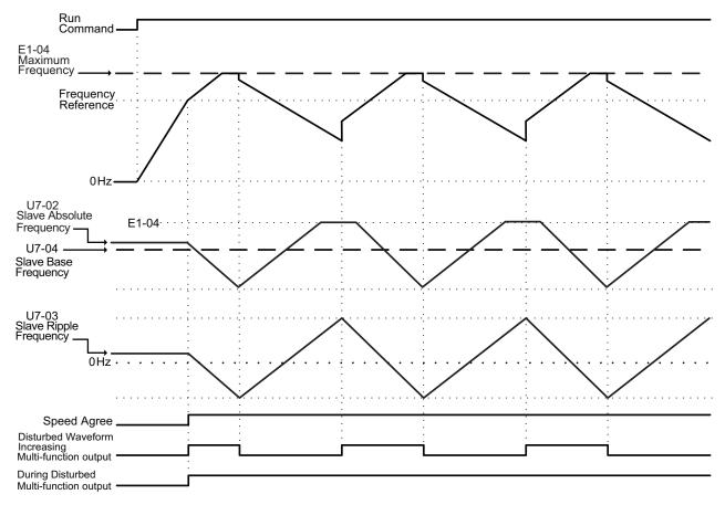
Figure 3 Traverse Mode Operation Outside of Max Output Frequency Parameter E1-04 / E3-04
