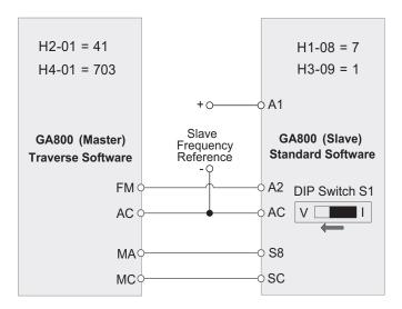
Figure 1 Software and Hardware Configuration for GA800 Traverse
