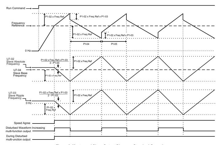
Figure 2 Master and Slave Output Diagram: Standard Operation
