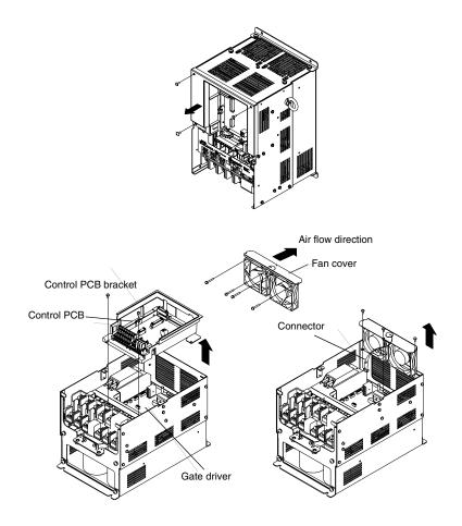
Fig 7.2 Cooling Fan Assembly Replacement Procedure
