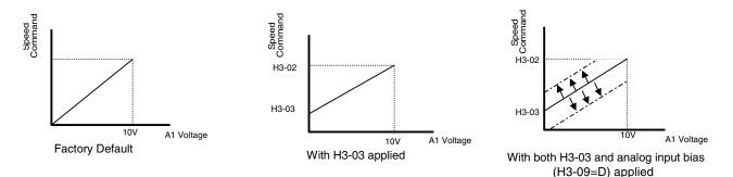
Fig. 30 Frequency Bias 2 Applied to Analog Speed Command
