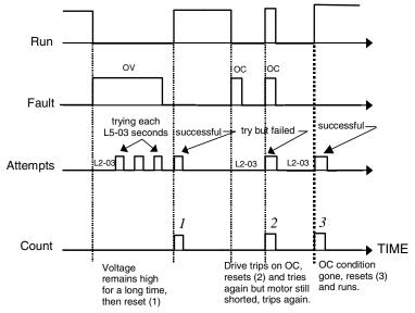
Fig. 37 Automatic Restart Timing Diagram
