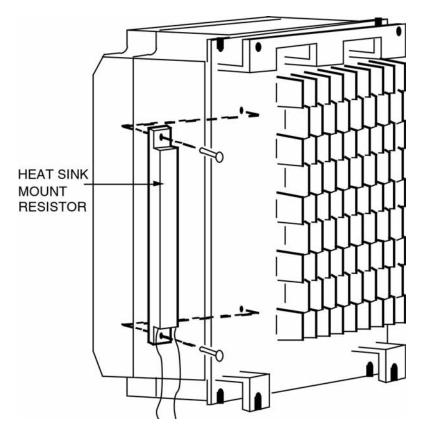
Fig 2.5 Attaching Heat Sink Mount Resistor on Heat Sink
