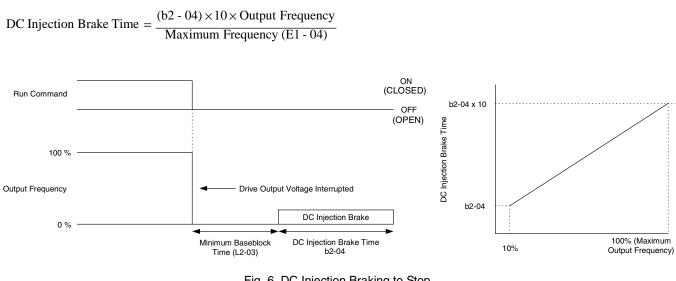
Fig. 6 DC Injection Braking to Stop
