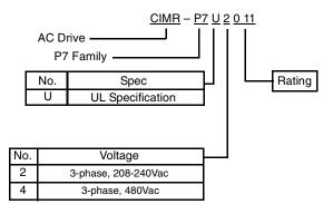
Fig 1.2 Drive Model Number Structure
