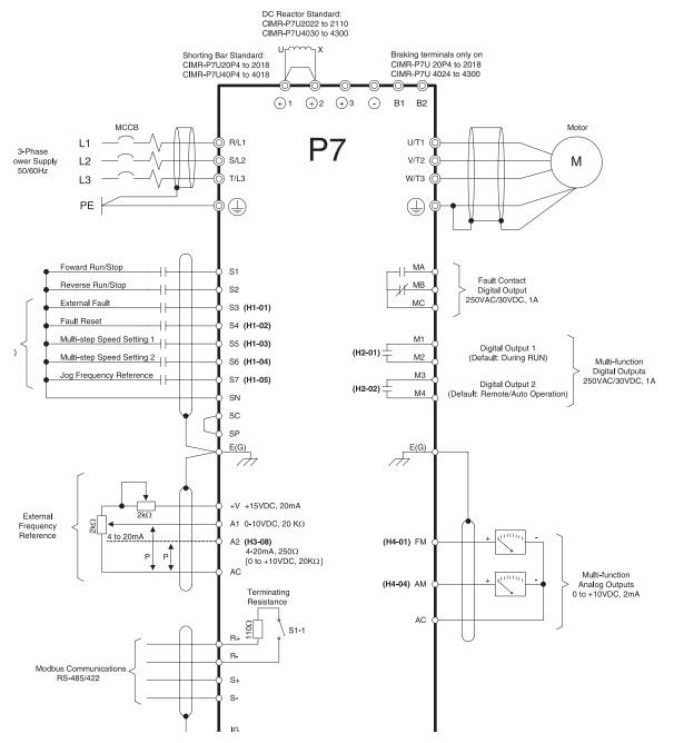
Fig 2.12 Terminal Connections
