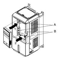
Fig 1.14 Mounting the Digital Operator
