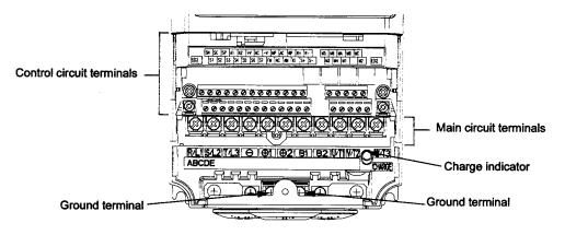
Fig 1.5 Terminal Arrangement (Terminal Cover Removed)
