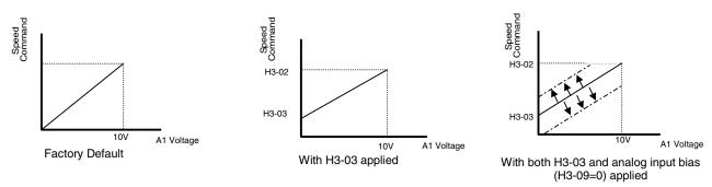
Fig. 29 Frequency Bias Applied to Analog Speed Command
