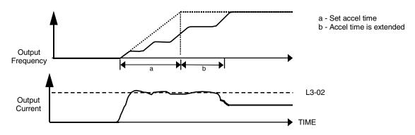
Fig. 33 Time Chart for Stall Prevention During Acceleration
