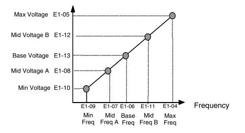
Fig. 22 Custom V/f Pattern Programming Curve
