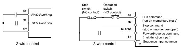
Fig. 1, 2 & 3-Wire Control Wiring Examples
