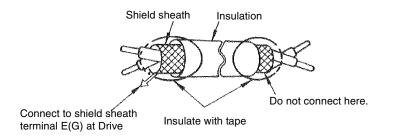
Fig 2.13 Preparing the Termination of Shielded Twisted-pair Cables
