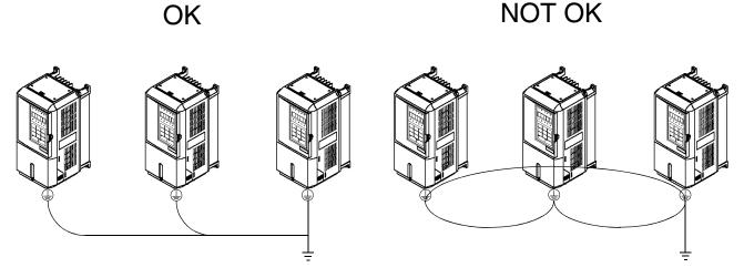
Fig 2.2 Ground Wiring Examples
