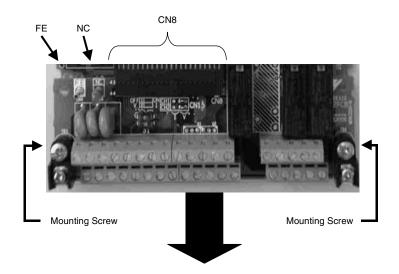
Fig 7.3 Terminal Card Removal Procedure
