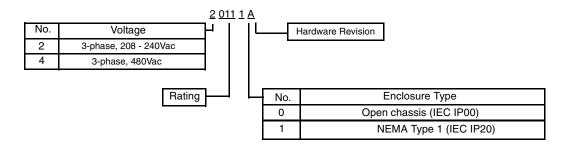
Fig 1.3 SPEC Number Structure
