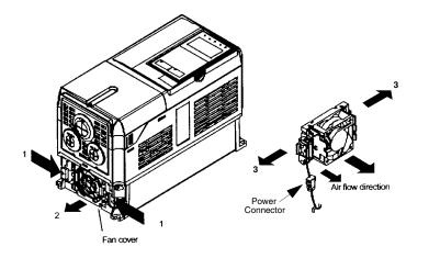
Fig 7.1 Cooling Fan Replacement Procedure
