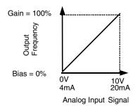
Fig. 23 Output Frequency as Commanded Via Analog Input
