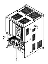
Fig 1.13 Removing the Front Cover
