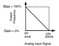
Fig. 26 Output Frequency with Inverted Gain and Bias Settings
