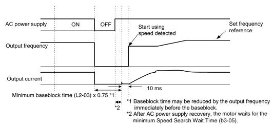
Fig. 10 Speed Search (Estimated Speed Method) after momentary power loss where the power loss time is less than the minimum baseblock time
