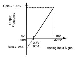
Fig. 25 Output Frequency with Reduced Bias Setting
