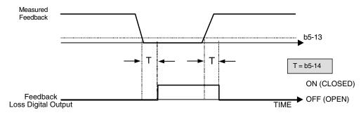
Fig. 17 Loss of PI Feedback Feature
