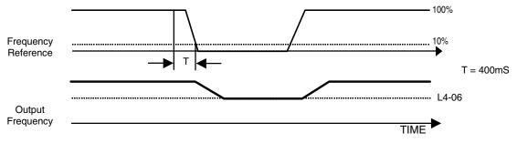
Fig. 36 Loss of Frequency Reference Timing Diagram
