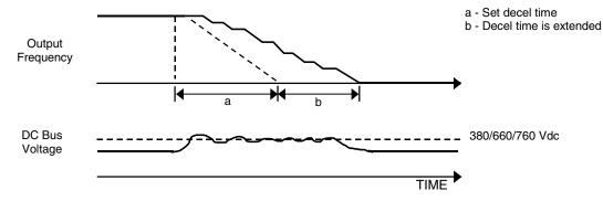
Fig. 34 Time Chart for Stall Prevention During Deceleration
