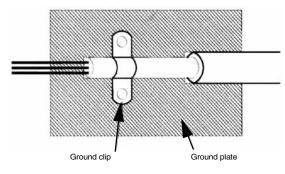
Fig G.1 Grounding Surface Layout
