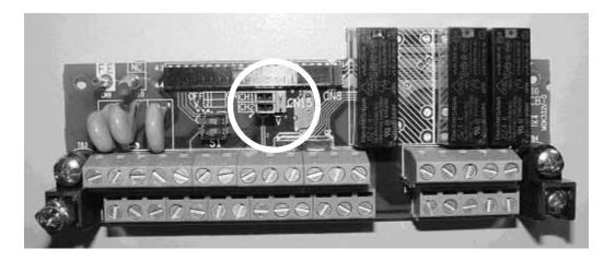
Fig 2.11 Shunt Connector CN15 Location
