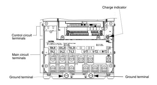
Fig 1.7 Terminal Arrangement (Terminal Cover Removed)
