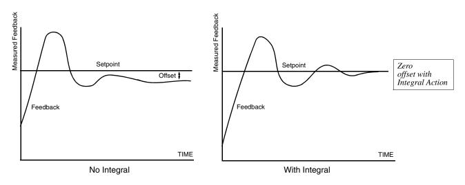
Fig. 16 PID Feedback Response Characteristics
