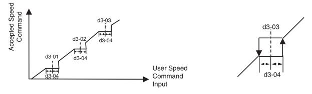
Fig. 21 Jump Frequency Characteristics
