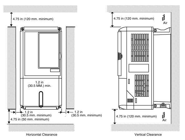
Fig 1.8 Drive Installation Orientation and Clearance
