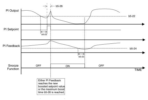
Fig. 19 Snooze Function Operation
