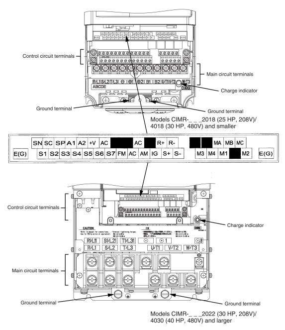
Fig 2.1 Control Circuit Terminal Layout
