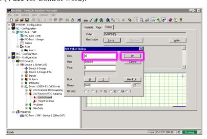
4. Force Fault Reset (128 dec for Control word).
