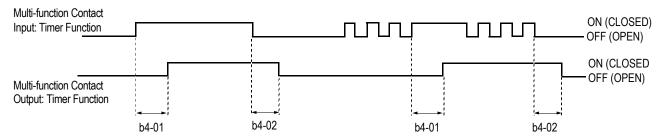
Figure 20 Timing Diagram of Timer Function
