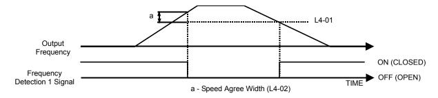
Figure 53 Freq Detect 1 Timing Diagram
