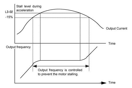
Figure 90 Detailed Time Chart for Stall Prevention During Acceleration
