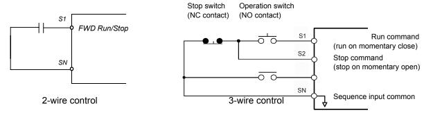
Figure 1 2 & 3-Wire Control Wiring Examples
