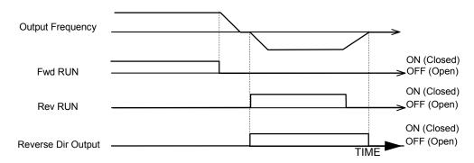
Figure 58 Reverse Direction Timing Diagram
