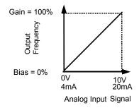
Figure 61 Output Frequency as Commanded Via Analog Input
