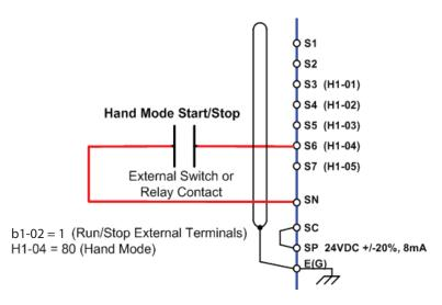
Figure 42 Connection Diagram for External Hand Mode Contact (b1-02 = 1)
