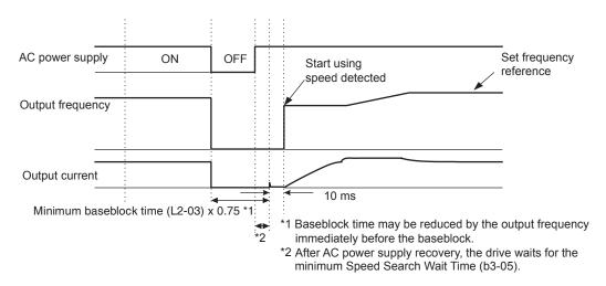
Figure 15 Speed Search (Estimated Speed Method) after momentary power loss where the power loss time is less than the minimum baseblock time
