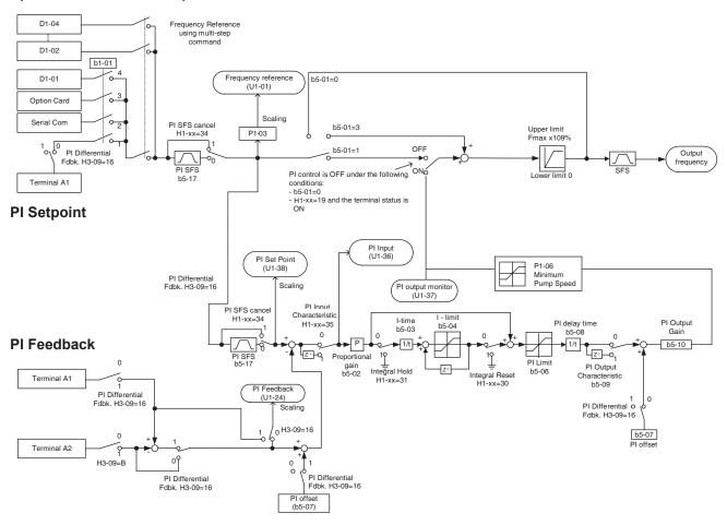
Figure 21 Pl Block Diagram
