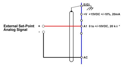
Figure 4 External Analog Signal Setpoint Reference
