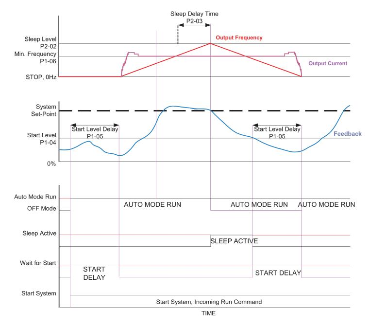
Figure 105 Sleep Function Based on Output Current
