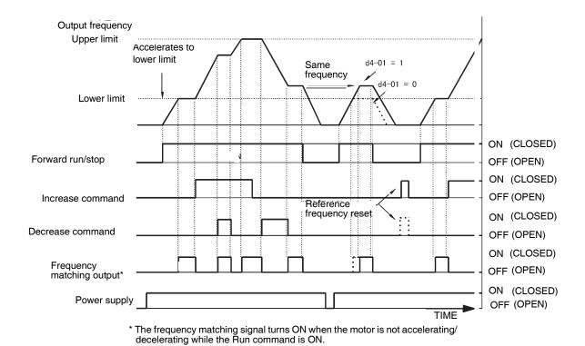
Figure 37 Floating Point Control Time Chart
