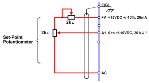
Figure 3 Setpoint Potentiometer Connection Diagram
