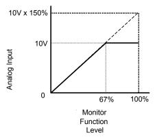
Figure 74 Analog Output gain Setting Adjustment
