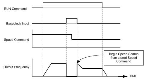
Figure 35 External Baseblock Characteristics
