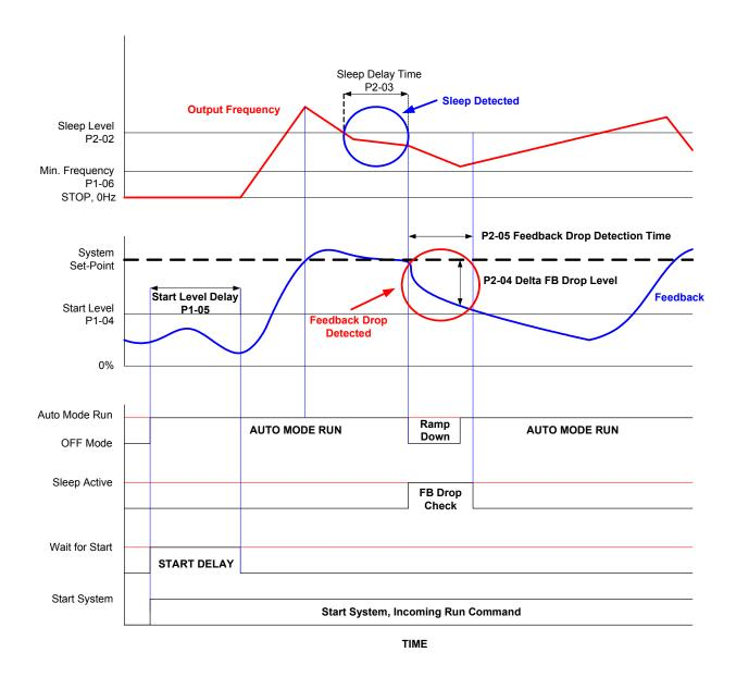
Figure 107 No-Flow Detection During Deceleration
