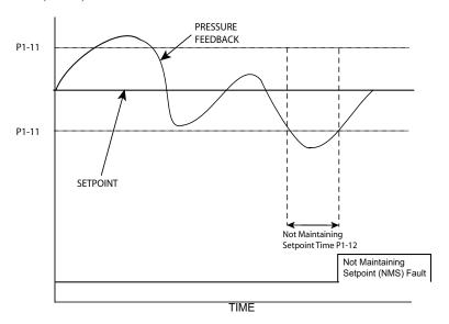
Figure 102 Not Maintaining Setpoint (NMS) Fault
