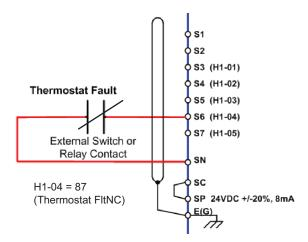
Figure 51 Wiring Diagram
