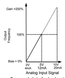
Figure 62 Output Frequency as Commanded via Analog Input with Increased Gain Setting
