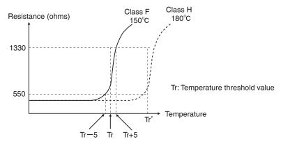
Figure 69 PTC Thermistor Temperature-Resistance Value Characteristics
