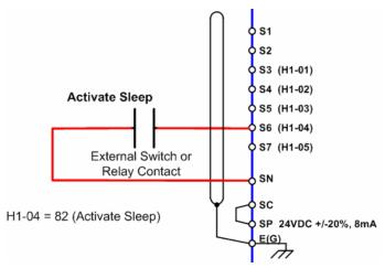
Figure 44 Wiring Diagram
