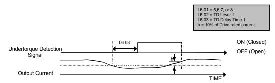
Figure 55 Trg Det 1 N.O. Timing Diagram
