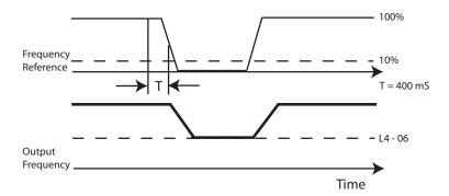
Figure 94 Loss of Frequency Reference Timing Diagram
