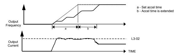
Figure 91 Time Chart for Stall Prevention During Acceleration
