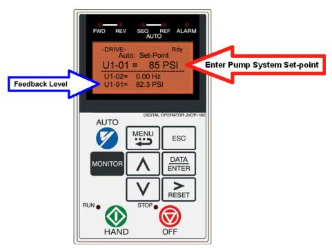
Figure 2 Digital Operator Auto Setpoint
