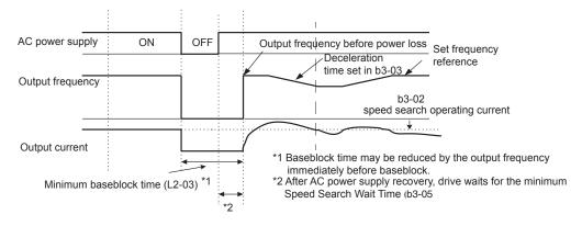
Figure 18 Speed Search (Current Detection Method) after momentary power loss where the power loss time is less than the minimum baseblock time
