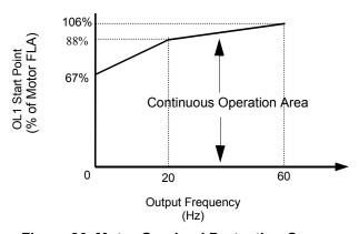
Figure 86 Motor Overload Protection Curve
