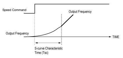
Figure 25 S-curve Characteristic Timing Diagram
