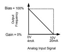
Figure 64 Output Frequency with Inverted Gain and Bias Settings
