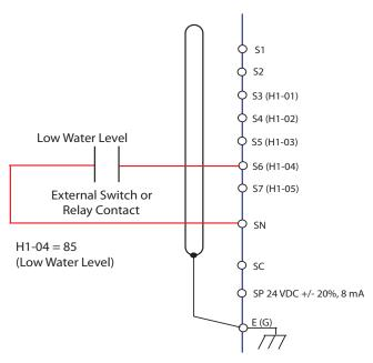
Figure 49 Wiring Diagram
