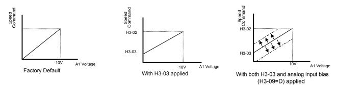
Figure 68 Frequency Bias 2 Applied to Analog Speed Command
