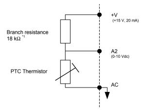
\*1 The resistance value of 18 k $\Omega$  is only valid for using a 3-phase PTC with the characteristics shown in the figure on following page.
