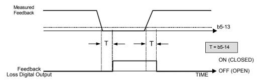
Figure 23 Loss of PI Feedback Feature
