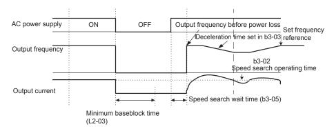
Figure 19 Speed Search (Current Detection Method) after momentary power loss where the power loss time exceeds the minimum baseblock time
