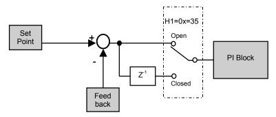
Figure 40 PI Error signal Inversion Block Diagram
