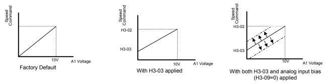
Figure 67 Frequency Bias Applied to Analog Speed Command
