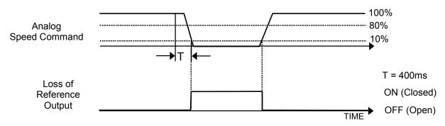
Figure 56 Loss of Reference Function Characteristics
