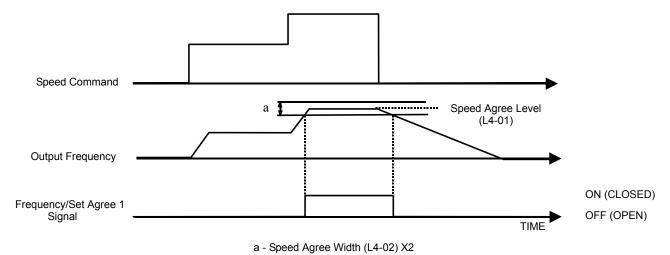
Figure 52 Fref/Set Agree 1 Timing Diagram
