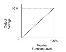
Figure 73 Analog Output Signal Level as a Function of the Monitor Value
