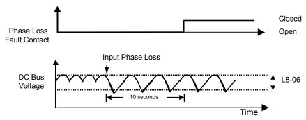
Figure 98 Input Phase Loss Detection Diagram
