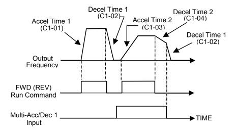
Figure 34 Multi-Accel/Dec Timing Diagram
