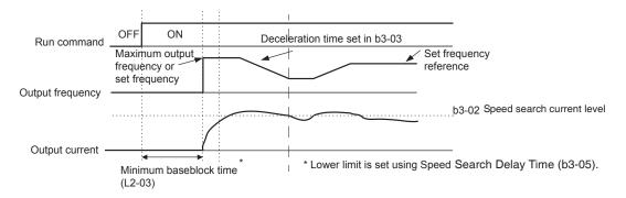
Figure 17 Speed Search (Current Detection Method) at Startup
