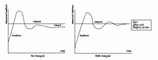
Figure 137 PI Feedback Response Characteristics
