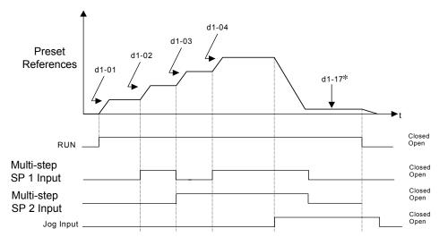
Figure 28 Setpoint and Jog Reference Timing Diagram
