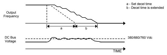
Figure 92 Time Chart for Stall Prevention During Deceleration
