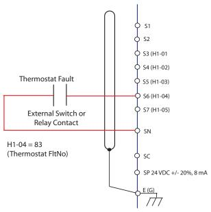
Figure 47 Wiring Diagram
