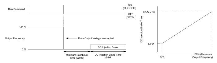
Figure 11 DC Injection Braking to Stop
