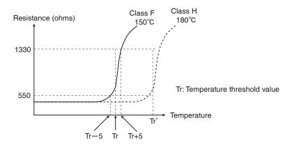
Figure 89 PTC Thermistor Temperature-Resistance Value Characteristics
