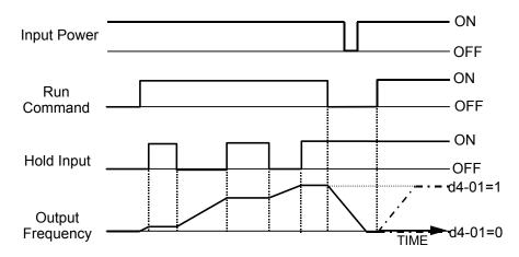
Figure 36 Accel/Dec RampHold Function Timing Diagram
