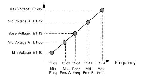
Figure 31 Custom V/f Pattern Programming Curve
