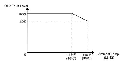
Figure 100 Ambient Temperature Derating Curve
