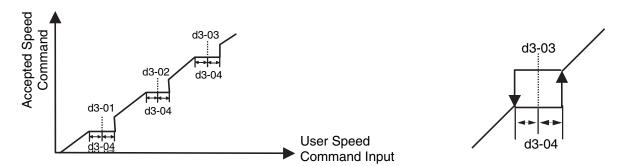
Figure 30 Jump Frequency Characteristics
