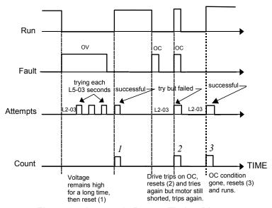
Figure 95 Automatic Restart Timing Diagram
