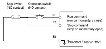
Figure 32 Terminal Configuration for 3-Wire Control
