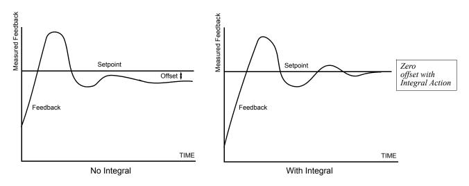
Figure 22 PI Feedback Response Characteristics
