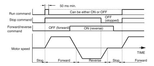
Figure 33 3-Wire Control Timing Diagram
