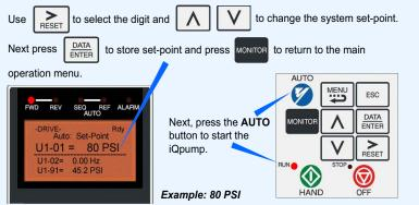
iQpump automatically starts in Auto Mode when the feedback signal level falls below the programmed level in parameter P1-04 for the specified time in P1-05.
