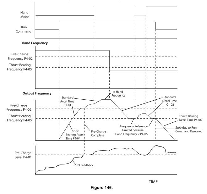
Thrust Bearing Mode and Pre-Charge Function with Alternating Auto and Hand Mode.
