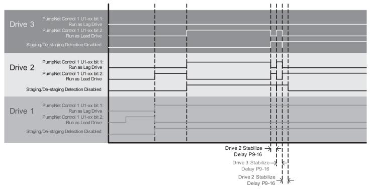
Figure 191. Stabilize Active Time and Off Delay
