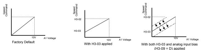
Figure 79. Frequency Bias 2 Applied to Analog Speed Command
