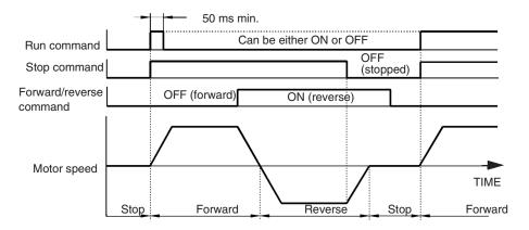
Figure 40. 3-Wire Control Timing Diagram
