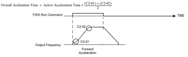
Figure 33. S-Curve Characteristic Timing Diagram
