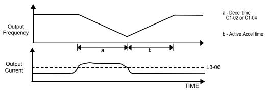
Figure 103. Time Chart for Stall Prevention Level During Running
