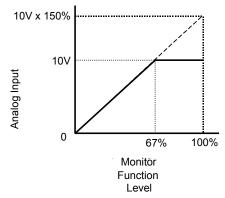
Figure 84. Analog Output gain Setting Adjustment
