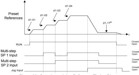
Figure 35. Setpoint and Jog Reference Timing Diagram
