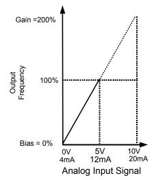
Figure 73. Output Frequency as Commanded via Analog Input with Increased Gain Setting
