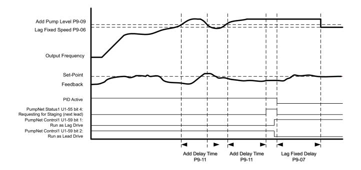
Figure 184. Drive Requests for a New Lead Drive using Output Frequency (P9-08 = 0)
