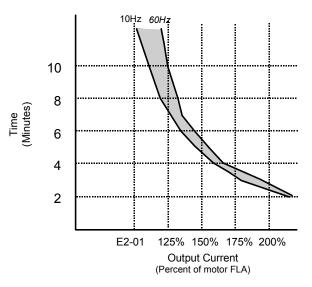
Figure 97. Motor Overload Protection Time based on Output frequency and Load
