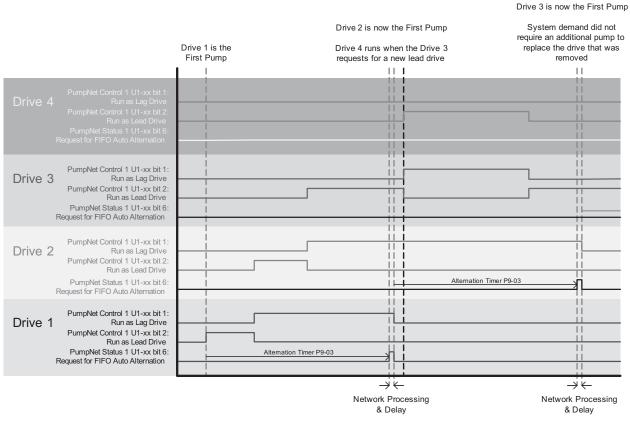
Figure 179. Alternation Mode is FIFO Auto
