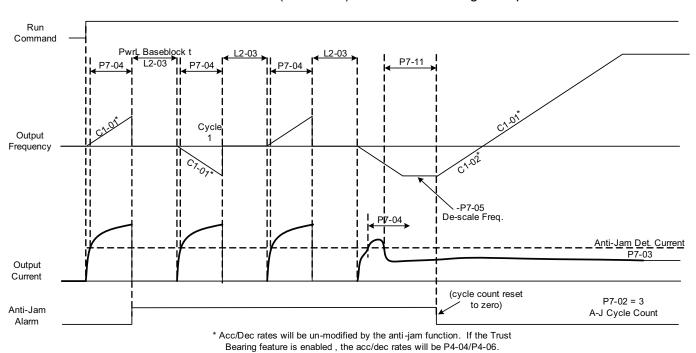
Anti-Jam Function Enabled (P7-01 = 1) – Jam clears during rev. operation
