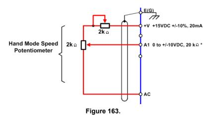
Connection Diagram of External Signal
