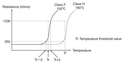
Figure 80. PTC Thermistor Temperature-Resistance Value Characteristics
