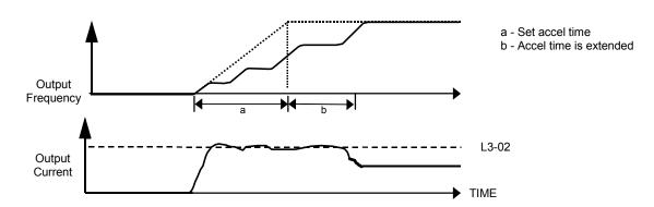
Figure 101. Time Chart for Stall Prevention During Acceleration
