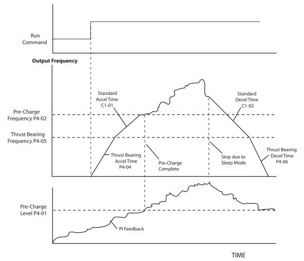
Thrust Bearing Mode and Pre-Charge Function in Auto Mode
