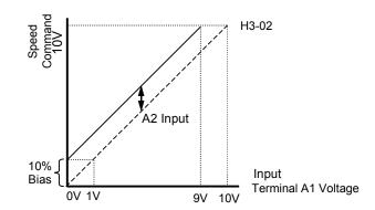
Figure 77. Effect of Frequency Bias Function on Speed Command
