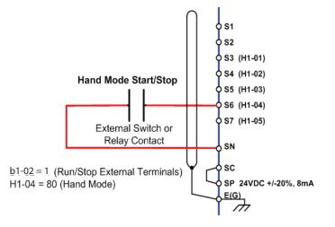
Figure 49. Connection Diagram for External Hand Mode Contact (b1-02 = 1)
