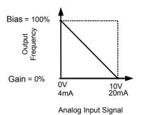
Figure 75. Output Frequency with Inverted Gain and Bias Settings
