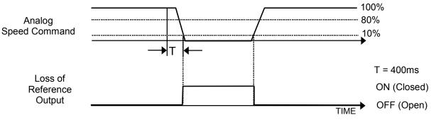
Figure 67. Loss of Reference Function Characteristics
