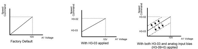
Figure 78. Frequency Bias Applied to Analog Speed Command
