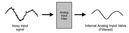
Figure 82. Analog Input Filter Time Constant Effect on "Noisy" Signal
