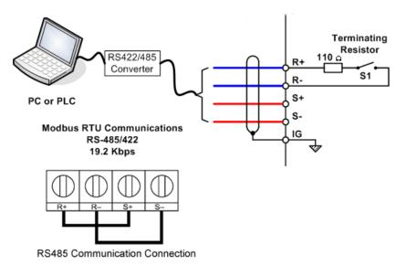
Figure 5. Connection Diagram of PC or PLC
