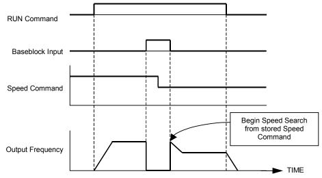
Figure 42. External Baseblock Characteristics
