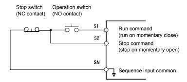
Figure 39. Terminal Configuration for 3-Wire Control
