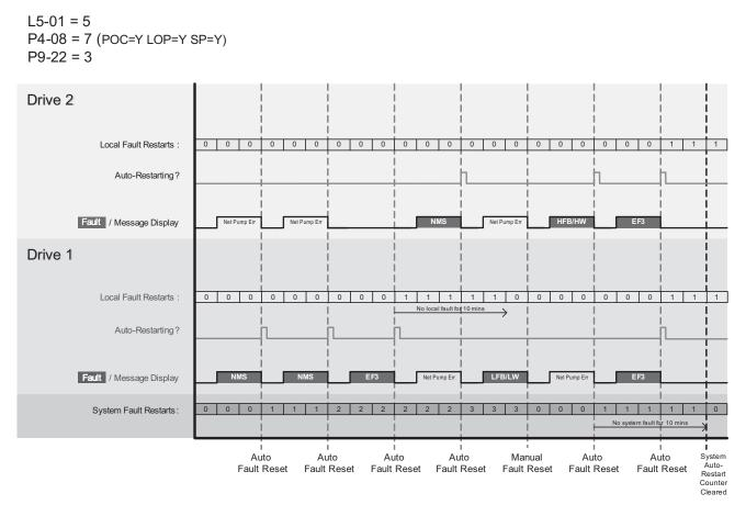
Figure 152. System Fault Auto-Restart Fault Counter
