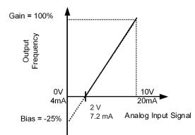
Figure 74. Output Frequency with Reduced Bias Setting
