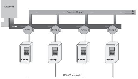
Figure 112. Example of Connections between Master and Drive <0034>
