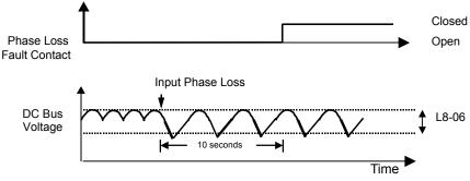
Figure 108. Input Phase Loss Detection Diagram
