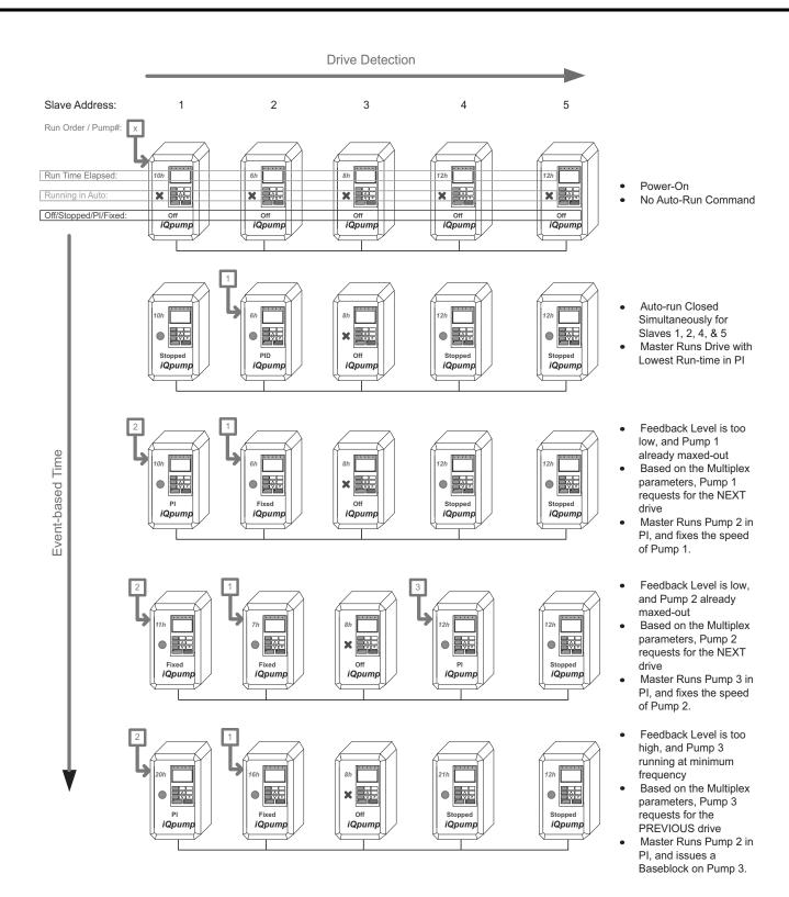
Figure 183. Multiplex Operation when P9-01 = 0 (Lowest Run-Time) and P9-05 = 0 (Lag Fixed)
