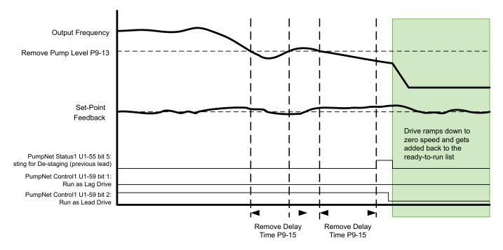
Figure 187. Drive Requests for a De-Stage using Output Frequency (P9-12 = 0)
