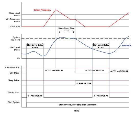
Figure 117. Sleep Function Based on Feedback Level
