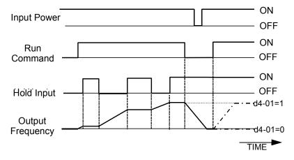
Figure 43. Accel / Dec Ramp Hold Function Timing Diagram
