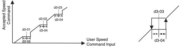
Figure 37. Jump Frequency Characteristics
