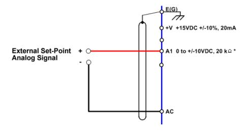
Figure 4. External Analog Signal Setpoint Reference
