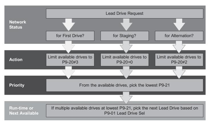
Figure 194. Lead Drive Selection Layers
