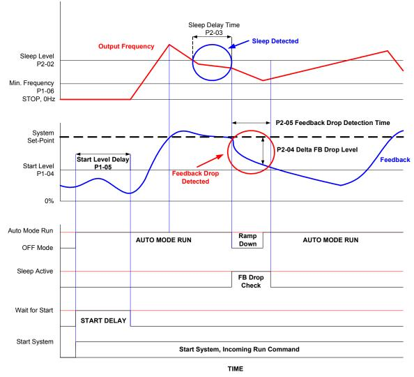
Figure 120. No-Flow Detection During Deceleration
