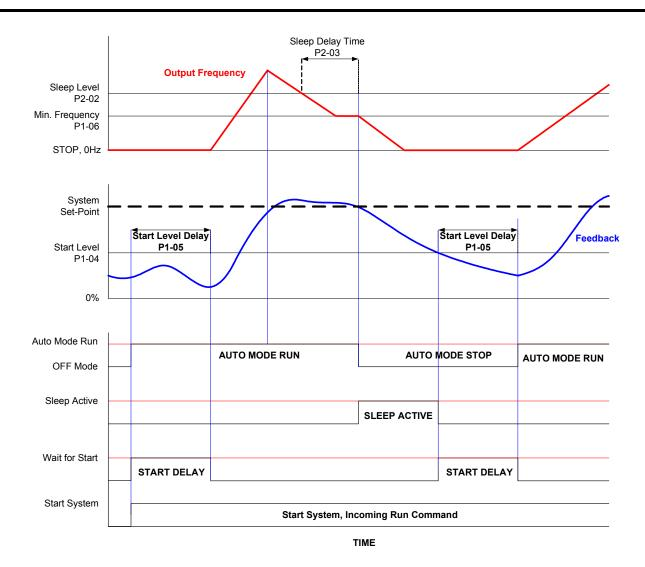
Figure 115. Sleep Function Based on Output Frequency
