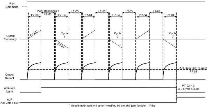
Anti-Jam Function Enabled (P7-01 = 1) – Anti-Jam Fault
