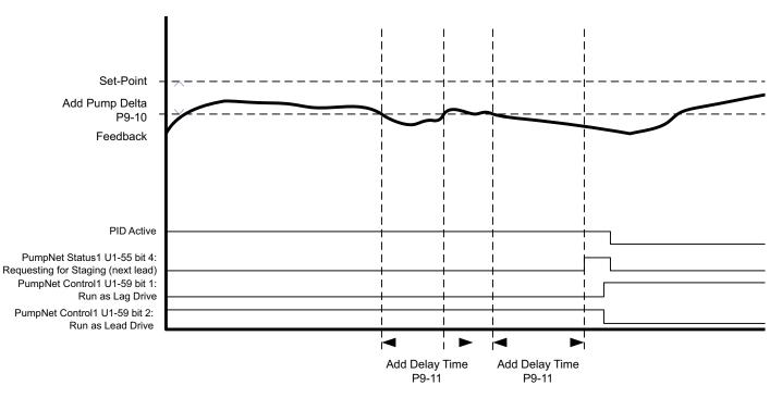
Figure 185. Drive Requests for a New Lead Drive using Feedback (P9-08 = 1)
