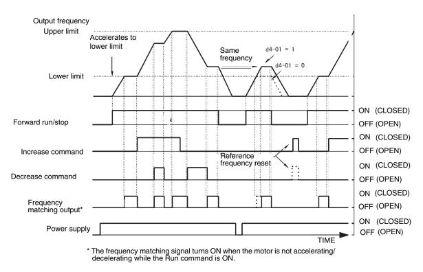
Figure 44. Floating Point Control Time Chart
