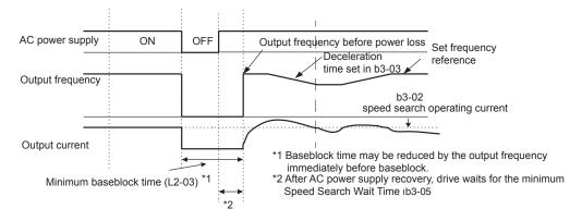
Figure 23. Speed Search (Current Detection Method) after momentary power loss where the power loss time is less than the minimum baseblock time
