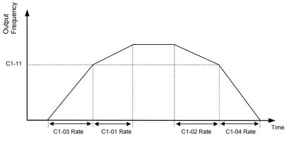
Figure 31. Accel / Decel Switch Frequency Operation
