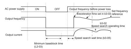
Figure 24. Speed Search (Current Detection Method) after momentary power loss where the power loss time exceeds the minimum baseblock time
