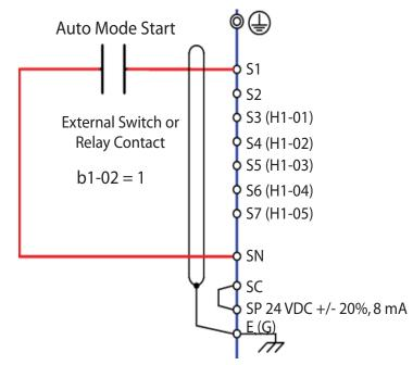
Figure 8. Connection Diagram of External Start / Stop Switch
