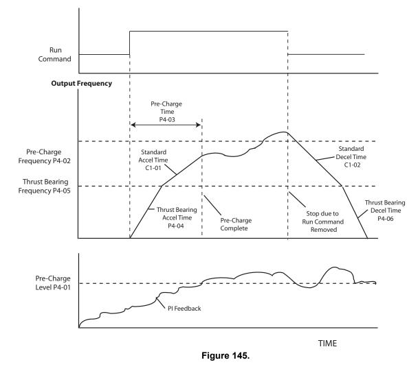
Thrust Bearing Mode and Pre-Charge Function in Auto Mode (Pre-Charge Time Expired)
