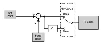
Figure 47. PI Error signal Inversion Block Diagram
