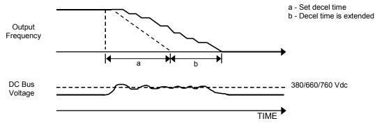
Figure 102. Time Chart for Stall Prevention During Deceleration
