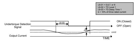
Figure 68. Trq Det 1 N.C. Timing Diagram
