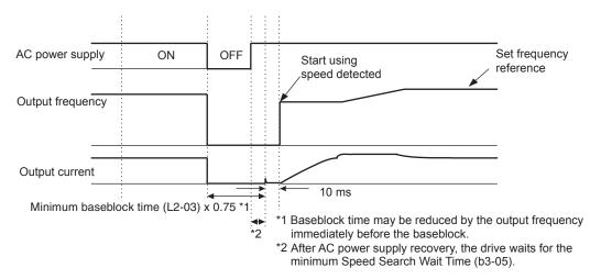
Figure 20. Speed Search (Estimated Speed Method) after momentary power loss where the power loss time is less than the minimum baseblock time
