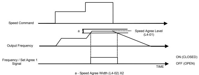
Figure 63. Fref / Set Agree 1 Timing Diagram
