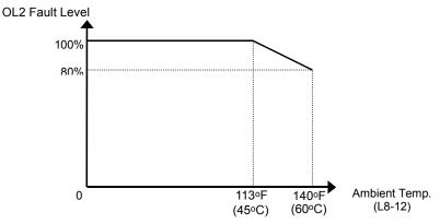
Figure 110. Ambient Temperature Derating Curve
