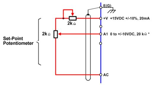
Figure 3. Setpoint Potentiometer Connection Diagram
