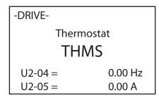
Figure 53. Thermostat Fault on Operator
