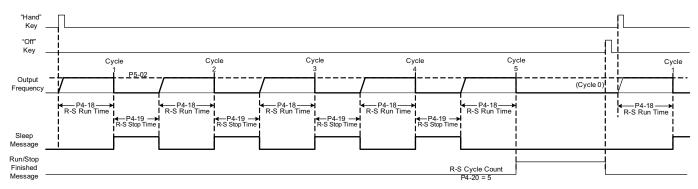
Figure 9. Run / Stop Control - HOA Operator JVOP162 - Coast to Stop
