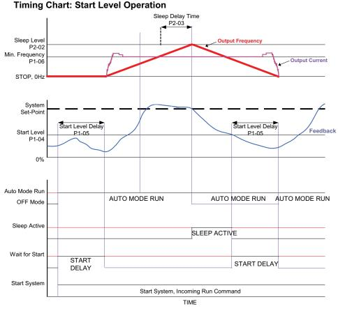
Figure 116. Sleep Function Based on Output Current
