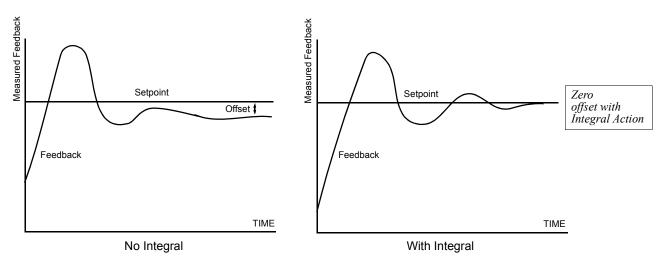
Figure 29. PI Feedback Response Characteristics
