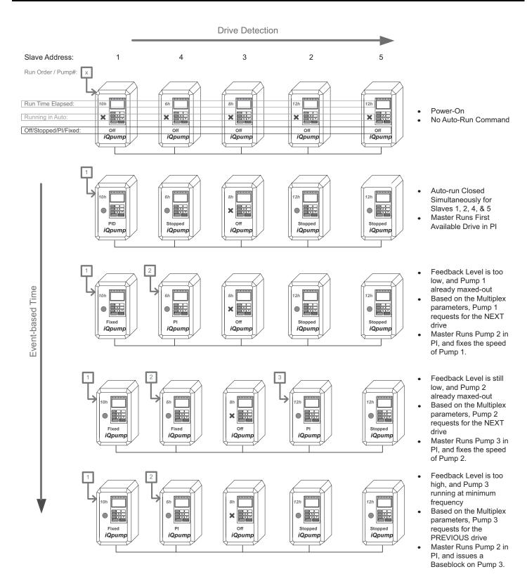
Figure 182. Multiplex Operation when P9-01 = 0 (Next Available) and P9-05 = 0 (Lag Fixed)
