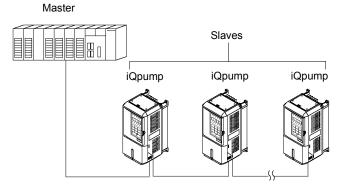
Figure 86. Example of Connections between Master and Drive
