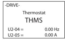
Figure 57. Thermostat Fault on Operator
