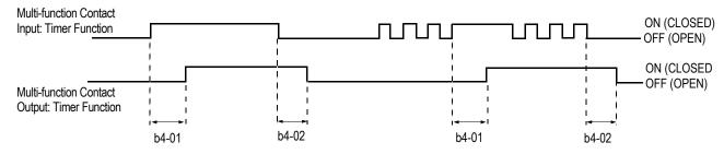
Figure 25. Timing Diagram of Timer Function
