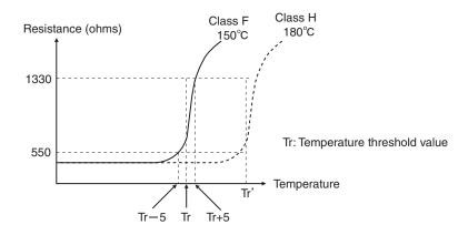
Figure 99. PTC Thermistor Temperature-Resistance Value Characteristics
