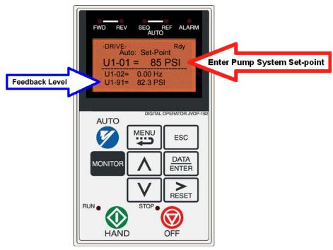
Figure 2. Digital Operator Auto Setpoint
