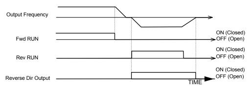
Figure 69. Reverse Direction Timing Diagram
