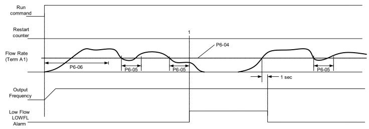
Figure 167. Low Flow Alarm (P6-07 = 1)
