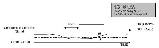
Figure 66. Trq Det 1 N.O. Timing Diagram
